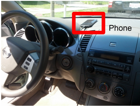
Figure 2: The data acquisition module running on a Galaxy Nexus smart phone, deployed in car.
