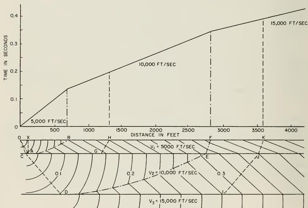
Fig. 3. - Wave-front diagram and travel-time graph. (After Johnson, 1954.)
