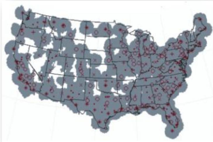
**Figure 7: PSR Coverage at 5000 Feet AGL [15]**
