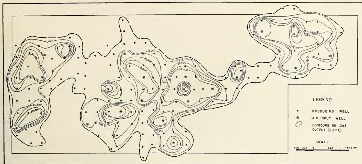
FIGURE 2. A repressured area in Crawford County, Illinois, with contours showing equal volumes of gas output per day.
