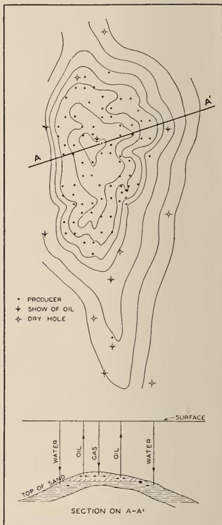
Fig. 13: Well density and contours showing structure
