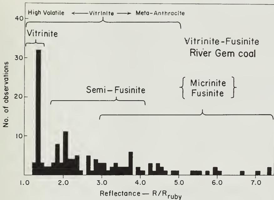
Fig. 3. - Reflectance of components of River Gem coal.
