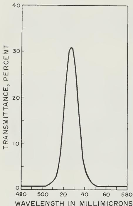
Fig. 1. - Spectral transmission of G.A.B. green filter.
