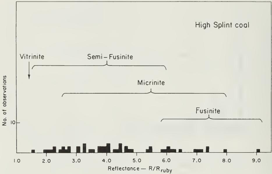
Fig. 5. - Reflectance of components of High Splint coal.
