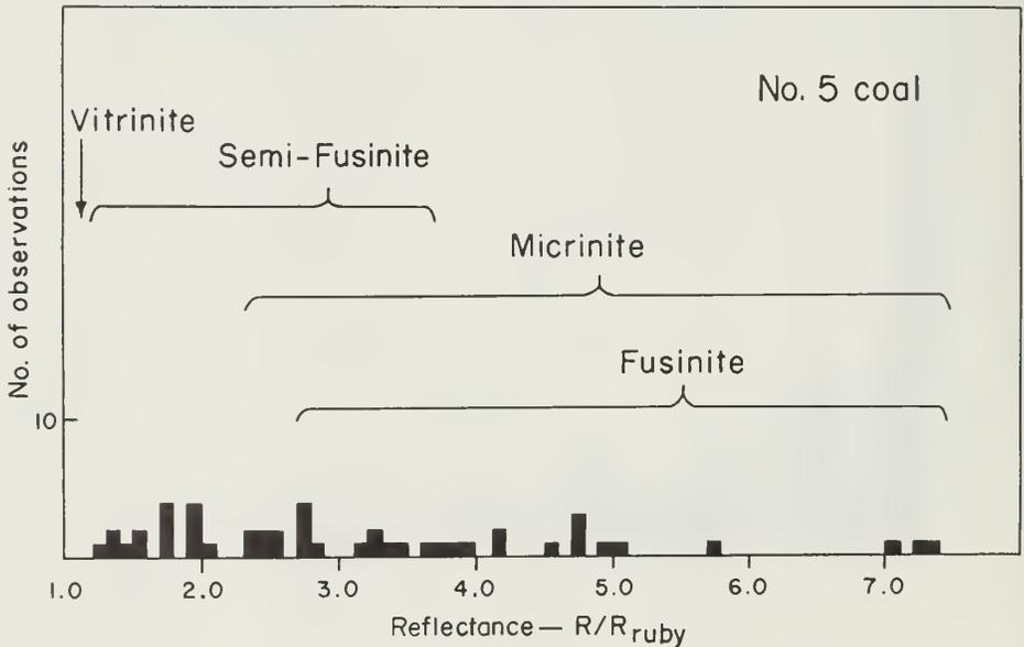
Fig. 6. - Reflectance of components of Illinois No. 5 coal.
