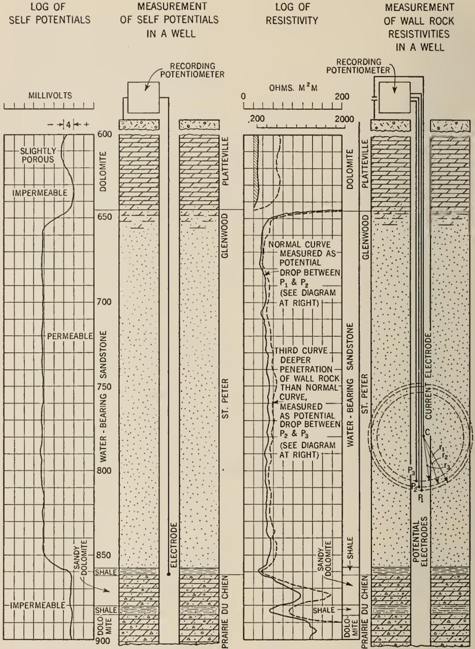
FIG. 1. Electric Logging of Water Well
