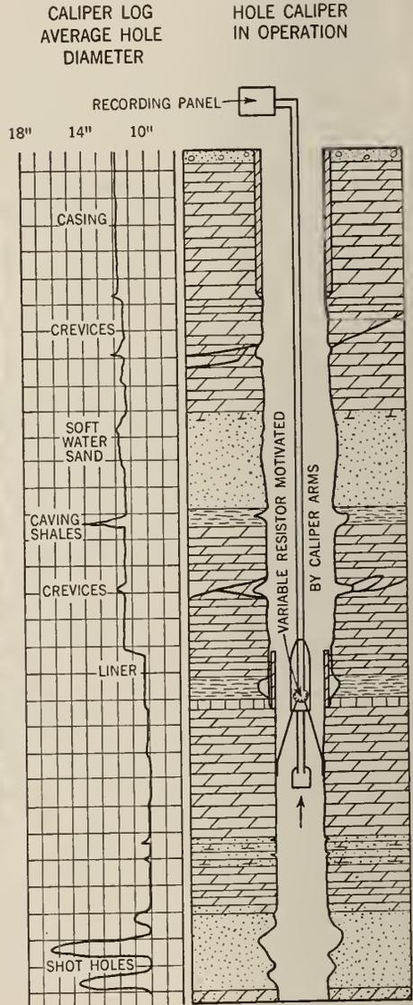
FIG. 3. Caliper Logging of Well
