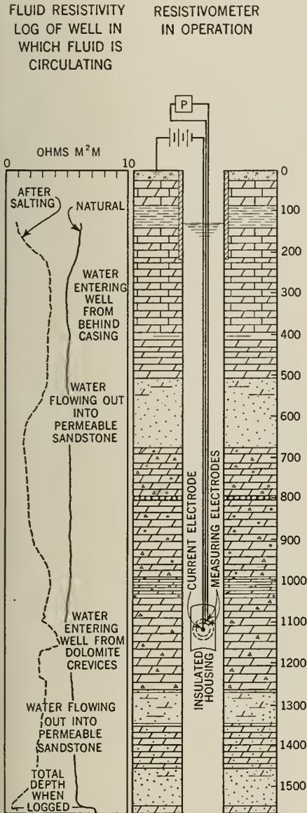
FIG. 4. Resistivometer Survey of Well
