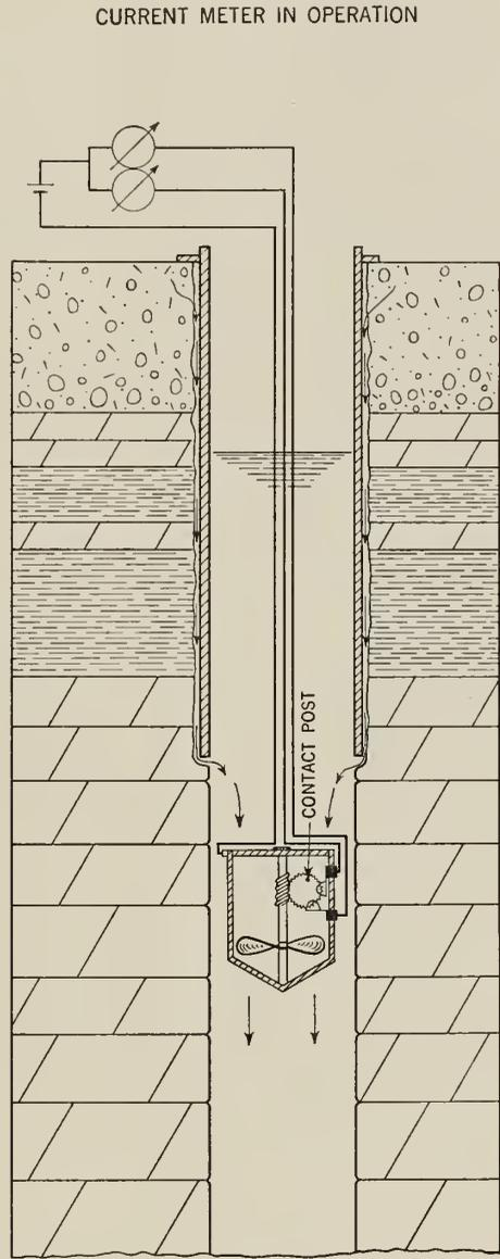
FIG. 5. Current Meter Survey of Well
