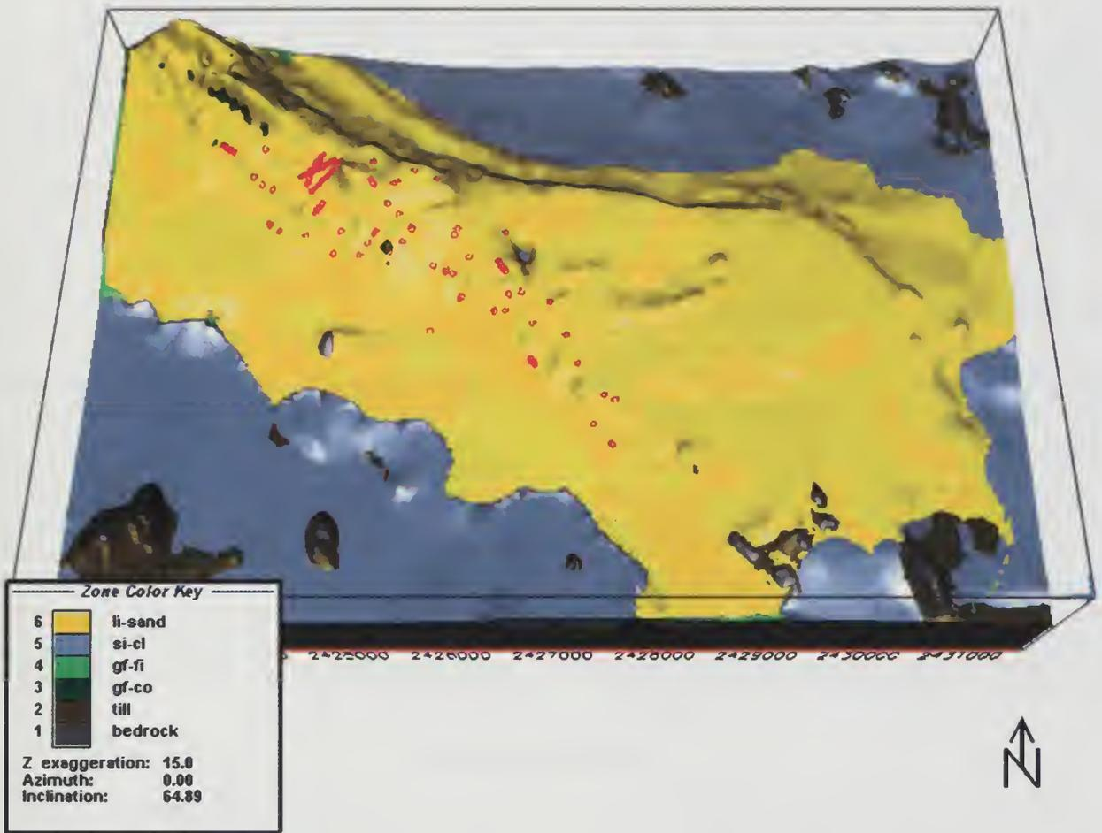
**Figure 6** Locations of the observed kettle holes (Mäkinen 2001, unpublished data) placed on the 3-D model as an annotation file (red dots). Observations are mostly based on the ground-penetrating radar and drilling log data. li-sand, littoral sand unit; si-cl, glaciolacustrine silt and clay unit; gf-fi, fine-grained glaciofluvial/glaciolacustrine unit; gf-co, coarse-grained glaciofluvial unit.
