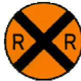
Advance Warning Sign
