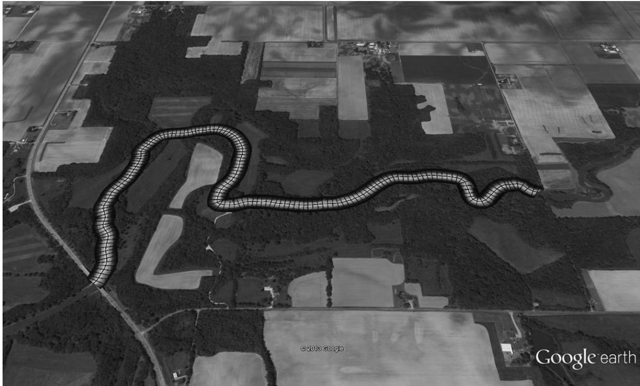
Figure 103.2: An example of the GIS maps created from side scan image files from the upper Kaskaskia River at the reach scale. Habitat will be quantified for the entire river segment by delineating habitat based on these images.
