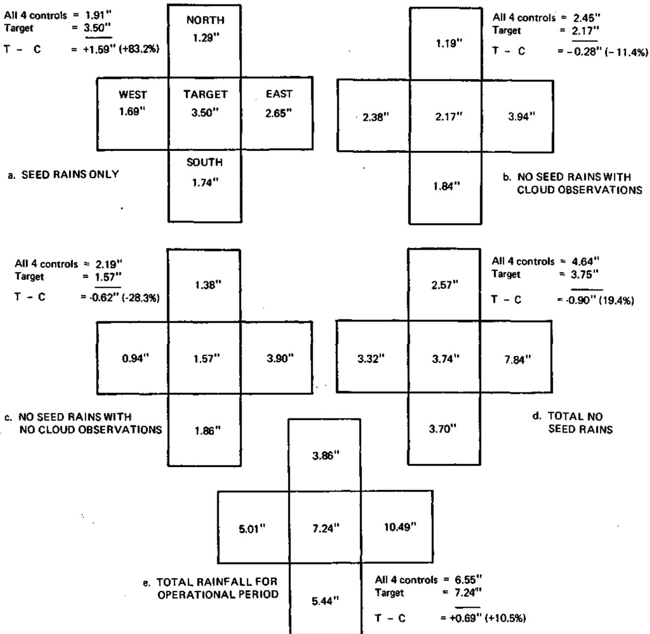
Figure 6. Area mean rainfall in target and control areas during the Southeastern Illinois Cloud Seeding Project in 1979. Values are based on NWS data.
