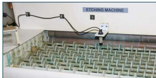
Sensor on etching machine to save water
