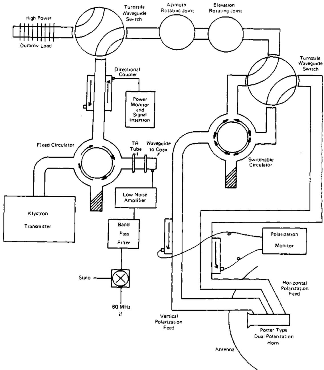
Figure 1. S-Band System for CHILL Radar.
