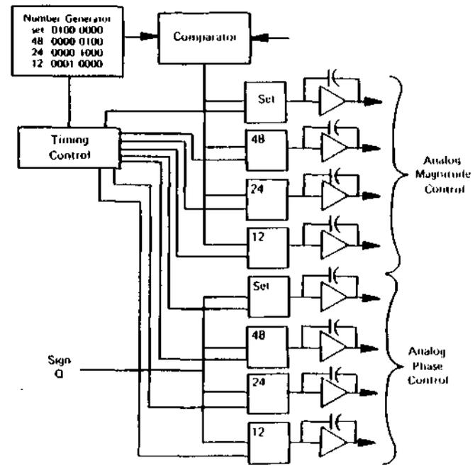
Figure 3. Block Diagram of Receiver System for CHILL Radar.
