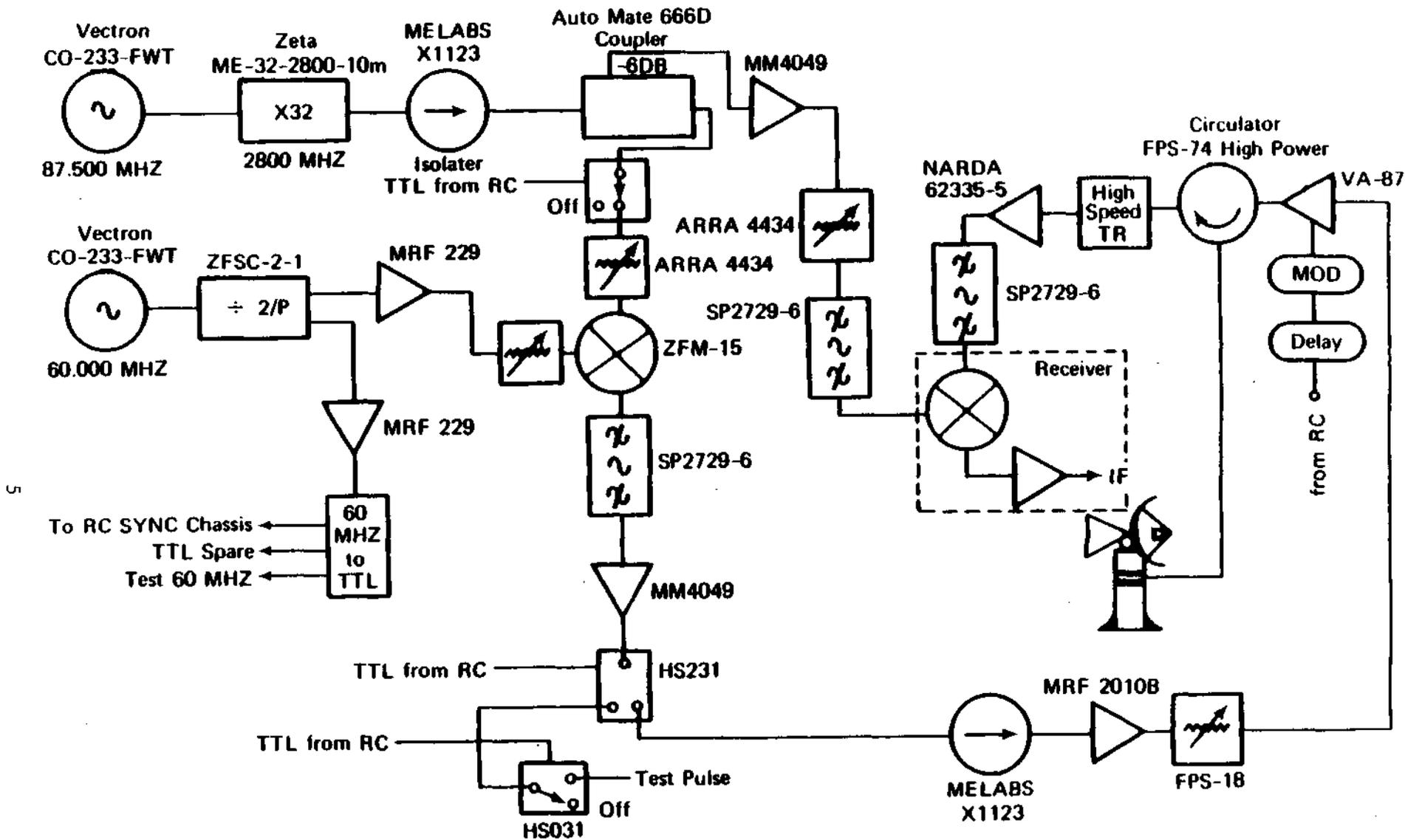
Figure 2. Block Diagram of Radio Frequency Source Redesign for CHILL Radar.
