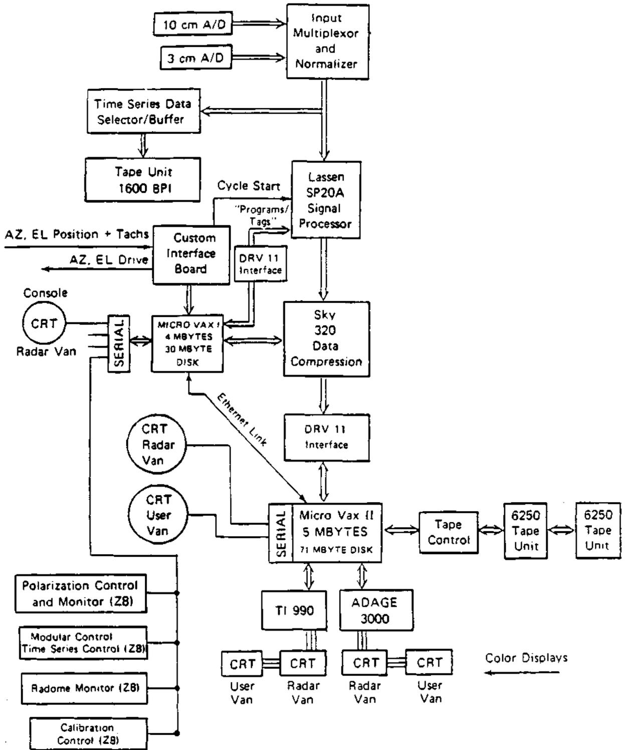
Figure 4. Block Diagram of Data Systems for CHILL Radar.
