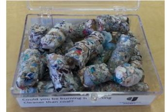
Fuel pellets made from label production waste
