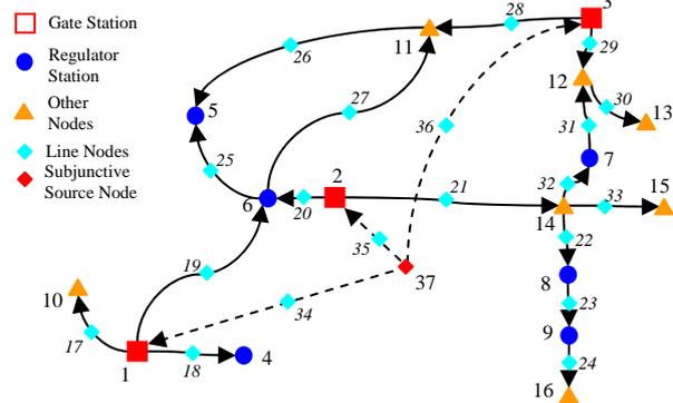
Figure 2. Directed graph model of MLGW gas network.
