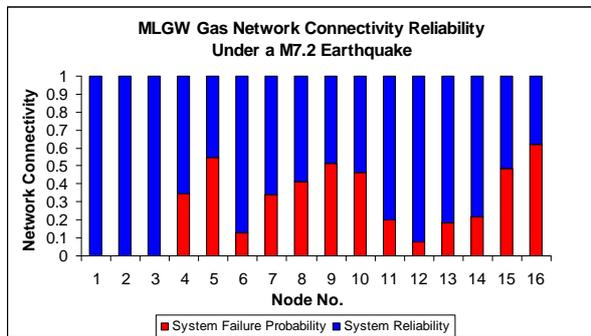
Figure 5. Connectivity reliabilities and failure probabilities of network nodes.
