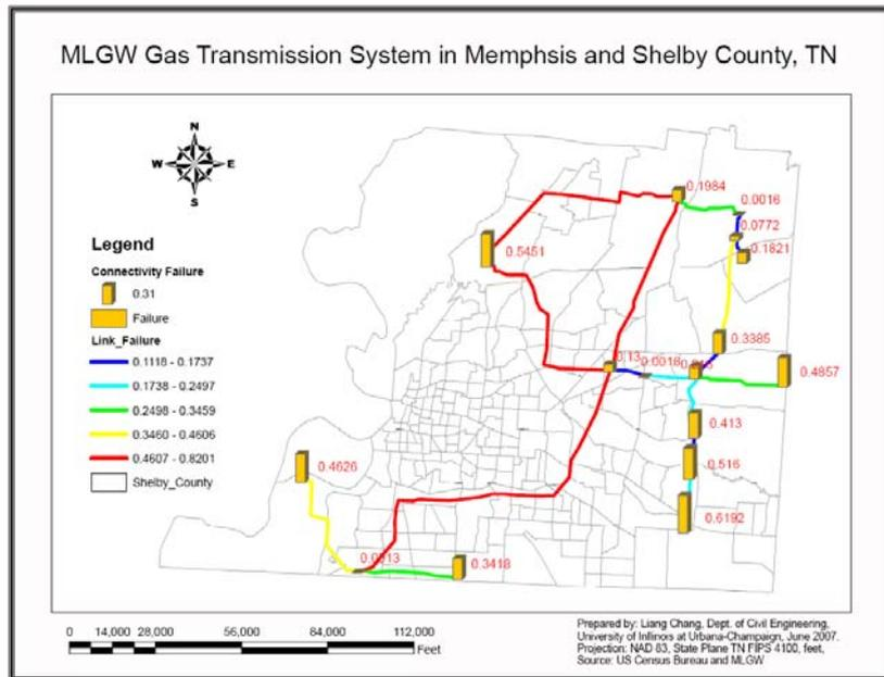
Figure 7. Connectivity failure probabilities of MLGW gas network (*ArcGIS* presentation)
