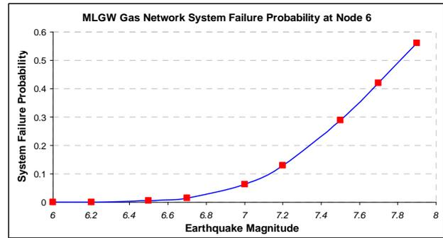
Figure 6. Failure probability at *Node 6* versus earthquake magnitude.
