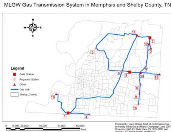
Figure 1. MLGW gas network in Shelby County, TN (modified from Chang et al., 1996).
