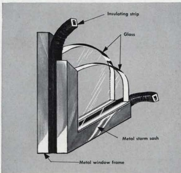
A metal window frame should be separated from a metal storm sash or storm panel to lessen condensation on the metal. For storm sash, use strips of wood, rubber or other insulating material.
