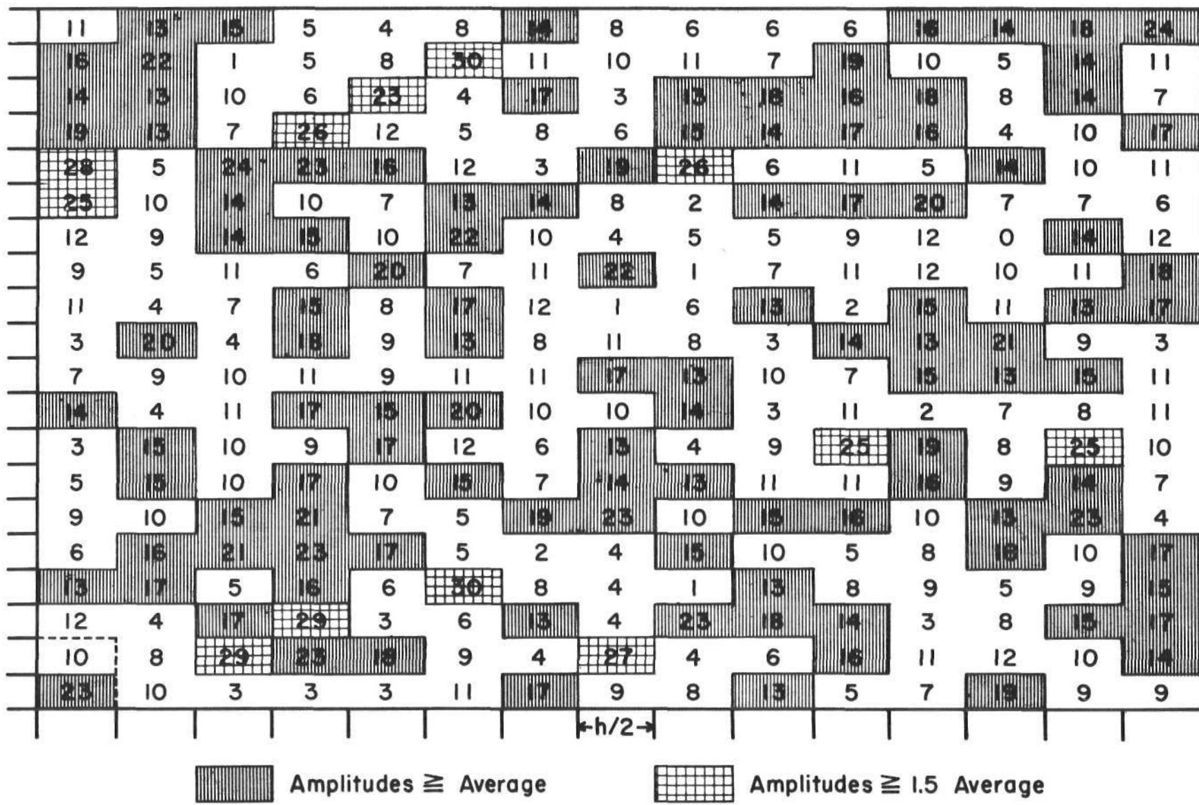
FIG. 3 TYPICAL APPEARANCE OF A SECTION OF A BRIGHTNESS-MODULATED DISPLAY. The Numbers Represent Amplitude Values Received From Element Of Area Resolved. (From McGill Univ. Rep. M.W. 4)
