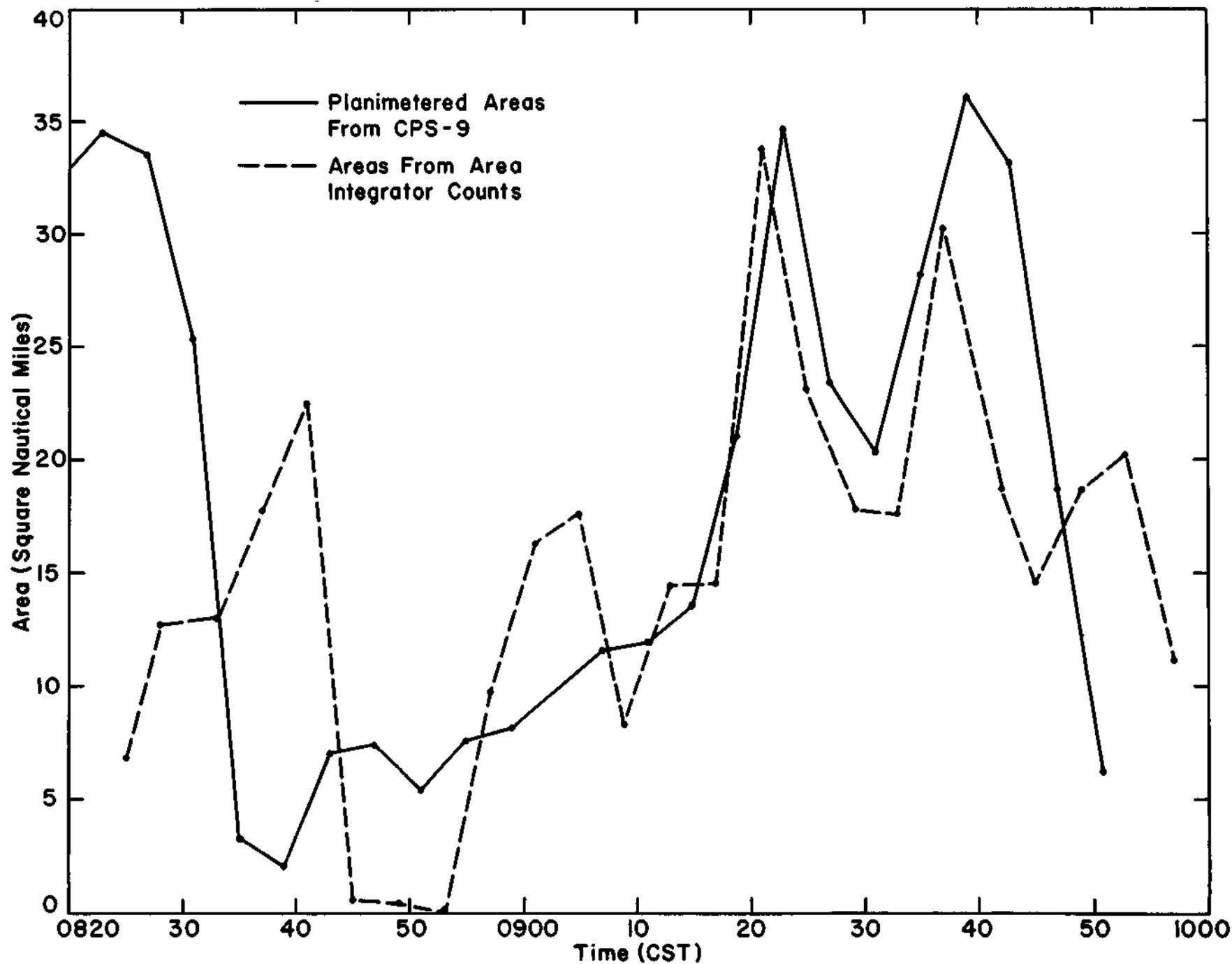
FIG.8 MINUTE BY MINUTE AREA COMPARISONS STORM OF AUGUST 29,1956
