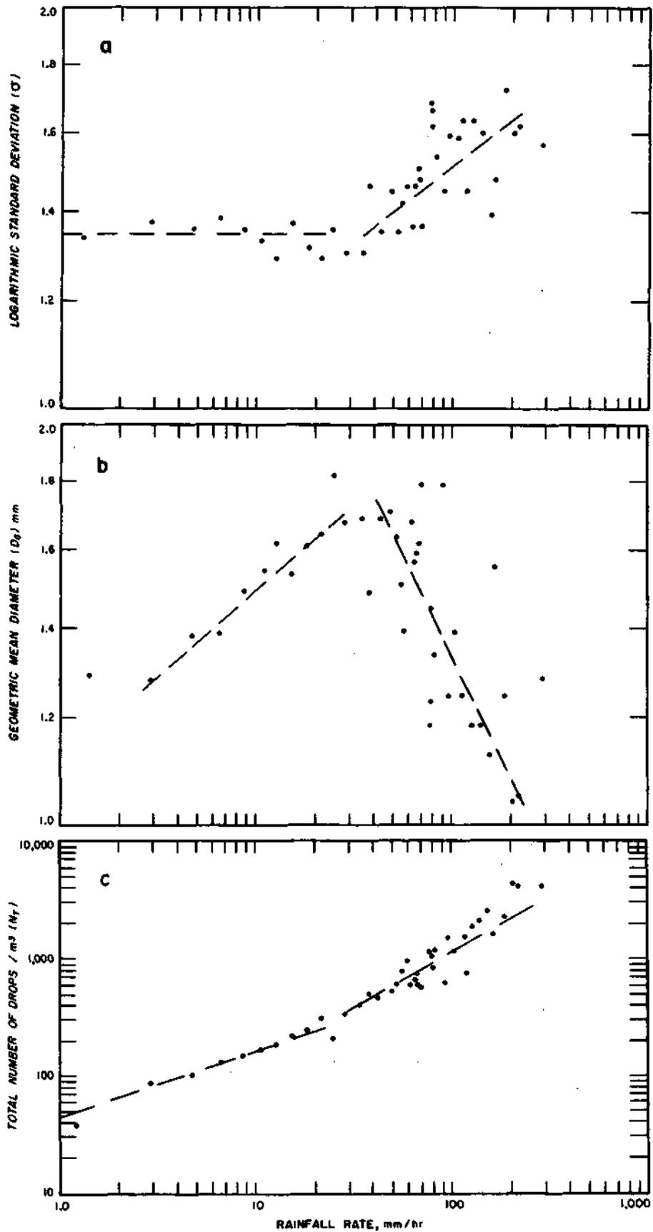
Figure 1. EXAMPLE OF DEPENDENCE OF THE LOG NORMAL COEFFICIENTS ON RAINFALL RATE FOR MIAMI THUNDERSTORMS
