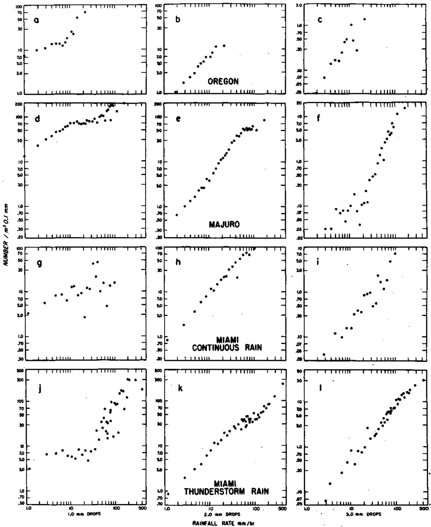
Figure 2. COMPARISON OF THE VARIATION OF DROP CONCENTRATION WITH RAINFALL RATE FOR DROP SIZES OF 1.0, 2.0, AND 3.0 mm
