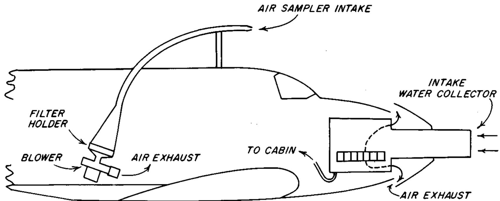
**Fig. 3 SCHEMATIC DIAGRAM OF AIRPLANE PRECIPITATION AND AIR SAMPLING SYSTEMS**
