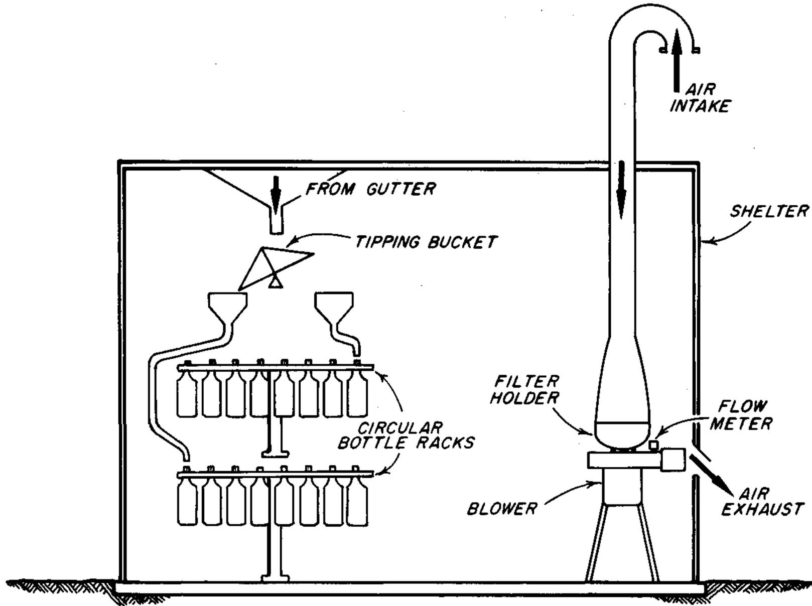
Fig. 2 SCHEMATIC DIAGRAM OF A SURFACE AIR AND PRECIPITATION SAMPLING STATIONS
