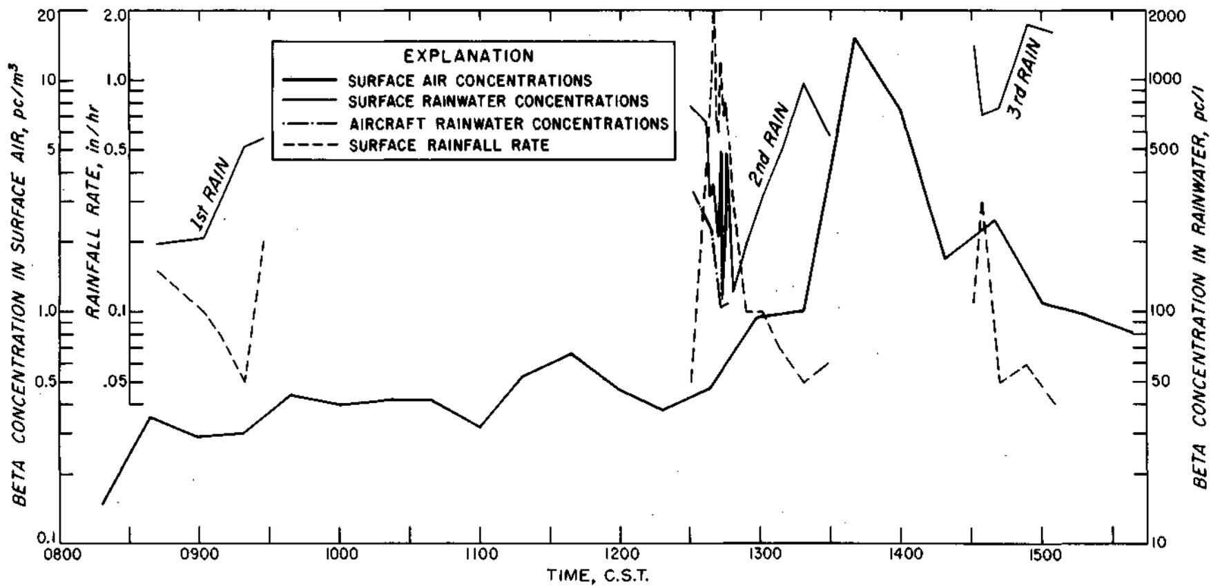
Fig. 5 DISTRIBUTION OF RADIOACTIVITY CONCENTRATIONS AND RAINFALL RATE AT STATION 12 ON MAY 26 , 1965
