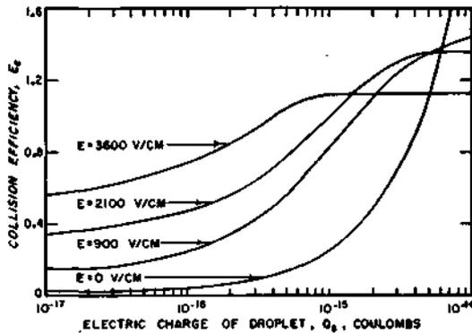
Fig. 9. Collision efficiency curves for a positively charged  $5\text{-}\mu$  droplet colliding with an uncharged  $30\text{-}\mu$  drop in electric fields oriented at  $= 0^\circ$ .
