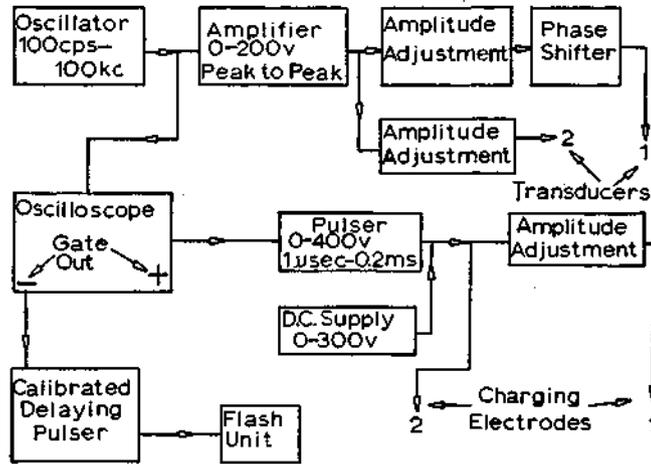
FIG. 2. Block diagram of the electrical apparatus.
