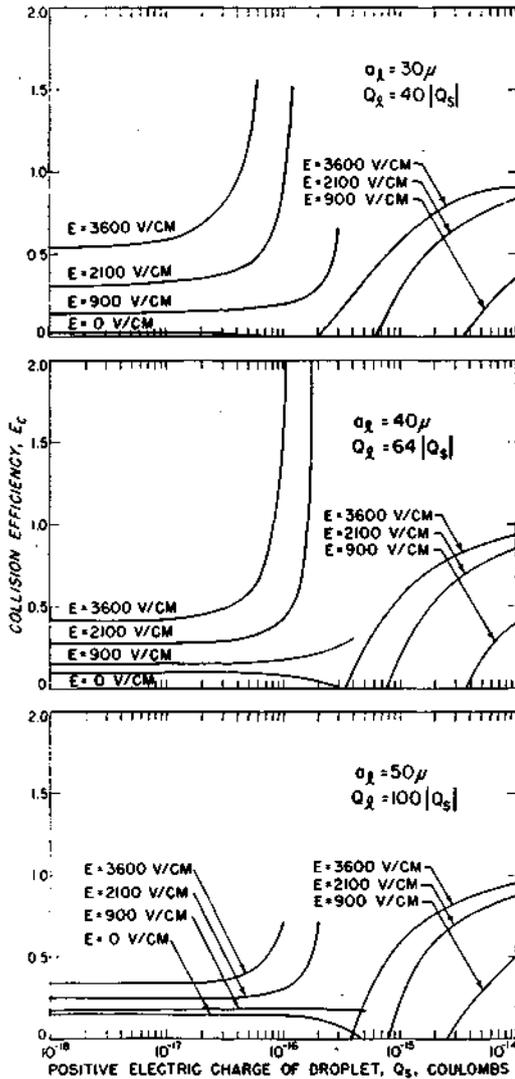
Fig. 3. Collision efficiency curves for a positively charged 5- $\mu$  droplet colliding with a 30-, 40-, and 50- $\mu$  drop in electric fields oriented at  $= 0^\circ$
