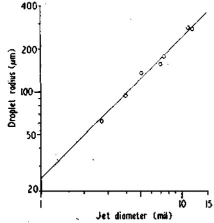
Figure 2. Jet diameter plotted against resulting droplet radius.
