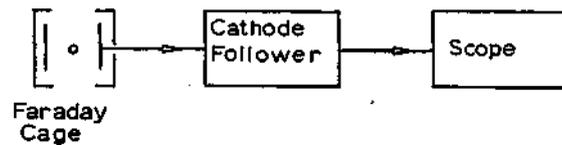
FIG. 3. Schematic diagram of electrical apparatus to measure the charge on the droplets.
