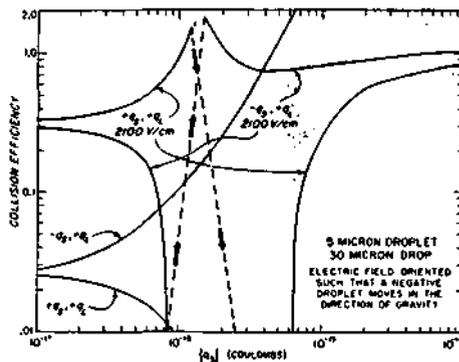
Fig. 5. Collision efficiencies for a 5 micron droplet with a 30 micron drop as a function of charge and electric field.
