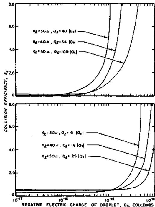
Fig. 2. Collision efficiency curves for a 5- $\mu$  (above) and 10- $\mu$  (below) droplet with a 30-, 40-, and 50- $\mu$  drop.
