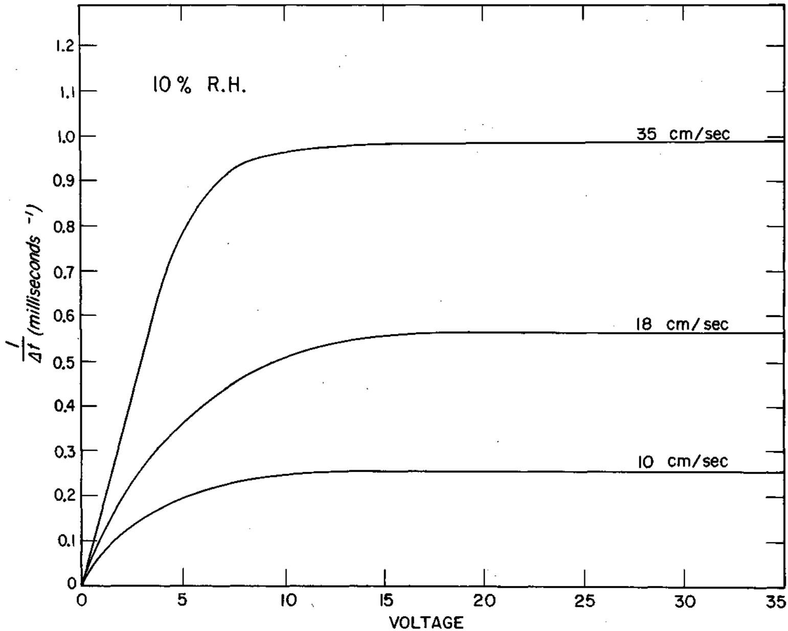
Figure 3. The inverse coalescence delay time versus voltage at impact velocities of 10, 18, and 35 cm/sec and 10 percent relative humidity.
