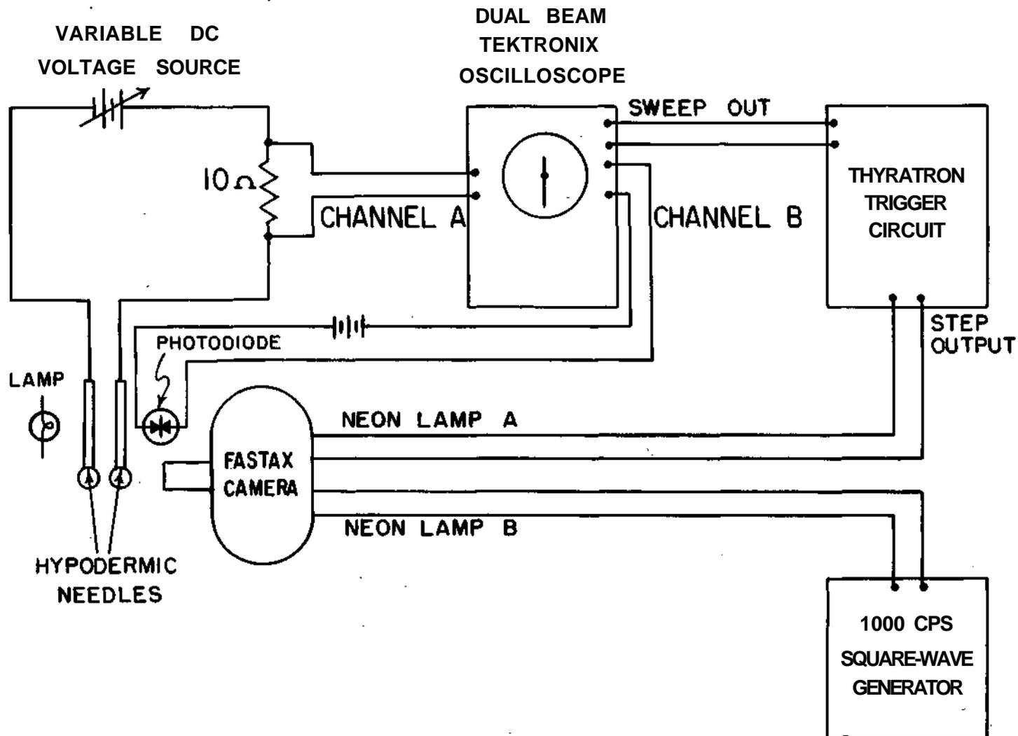
Figure 1. Block diagram of the experimental apparatus used for the determination of coalescence delay time.
