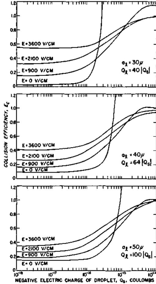
Fig. 8. Collision efficiency curves for a negatively charged 5- $\mu$  droplet colliding with a 30-, 40-, and 50- $\mu$  drop in electric fields oriented at  $\theta = 180^\circ$ .
