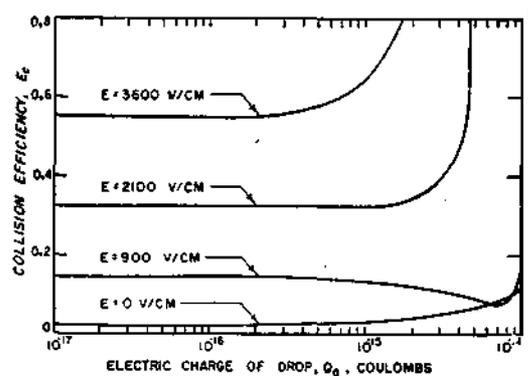
Fig. 10. Collision efficiency curves for an uncharged  $5\text{-}\mu$  droplet colliding with a positively charged  $30\text{-}\mu$  drop in electric fields oriented at  $= 0^\circ$ .
