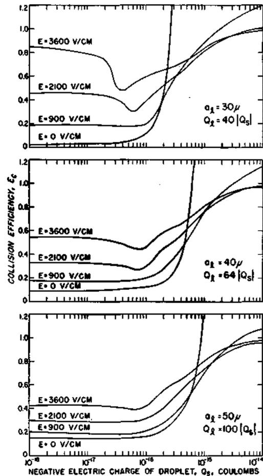
Fig. 6. Collision efficiency curves for a negatively charged  $5\text{-}\mu$  droplet colliding with a  $30\text{-}\mu$ ,  $40\text{-}\mu$ , and  $50\text{-}\mu$  drop in electric fields oriented at  $= 90^\circ$ .
