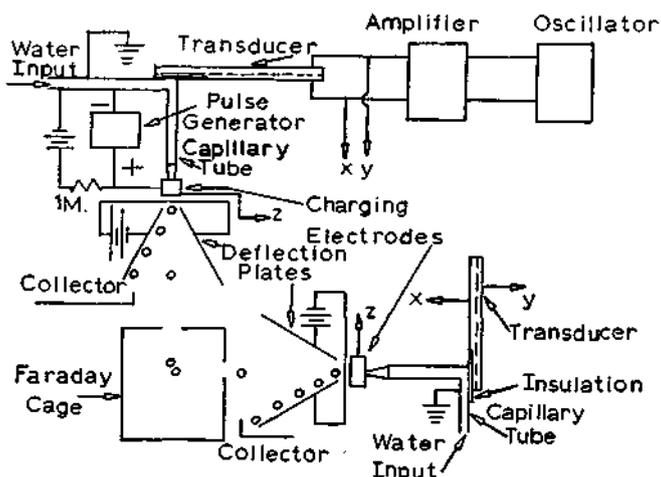
FIG. 1. Schematic diagram of experimental apparatus to study the collision of two liquid droplets.
