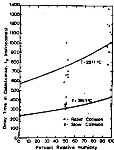
Fig. 1. Coalescence delay time as a function of relative humidity determined from Newton ring patterns.
