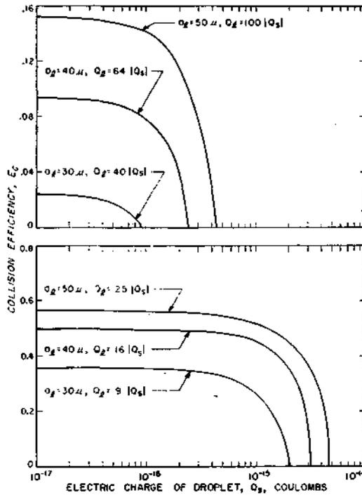
Fig. 1. Collision efficiency curves for a 5- $\mu$  (above) and 10- $\mu$  (below) droplet with a 30-, 40-, and 50- $\mu$  drop.
