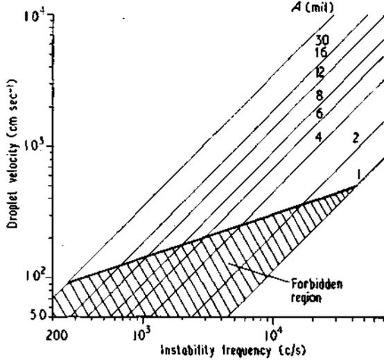
Figure 1. Droplet velocity, plotted against instability frequency for various jet diameters.
