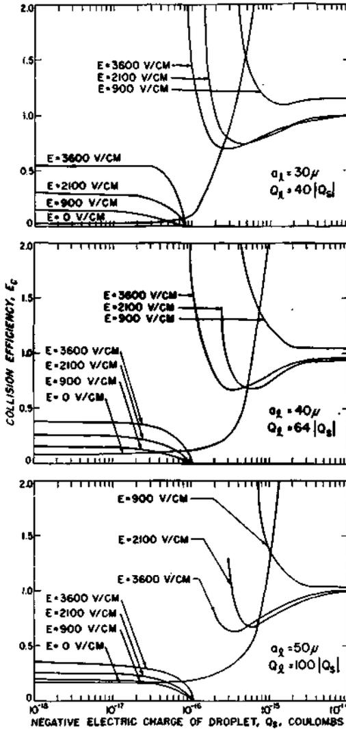
Fig. 4. Collision efficiency curves for a negatively charged 5- $\mu$  droplet colliding with a 30-, 40-, and 50- $\mu$  drop in electric fields oriented at  $= 0^\circ$ .
