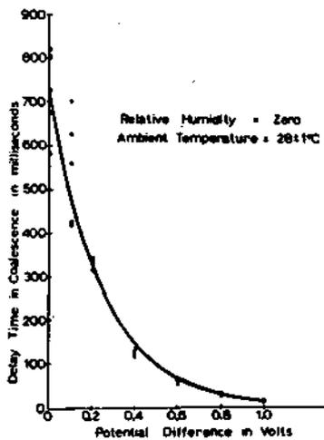
Fig. 2. Coalescence delay time as a function of voltage determined from Newton ring patterns.
