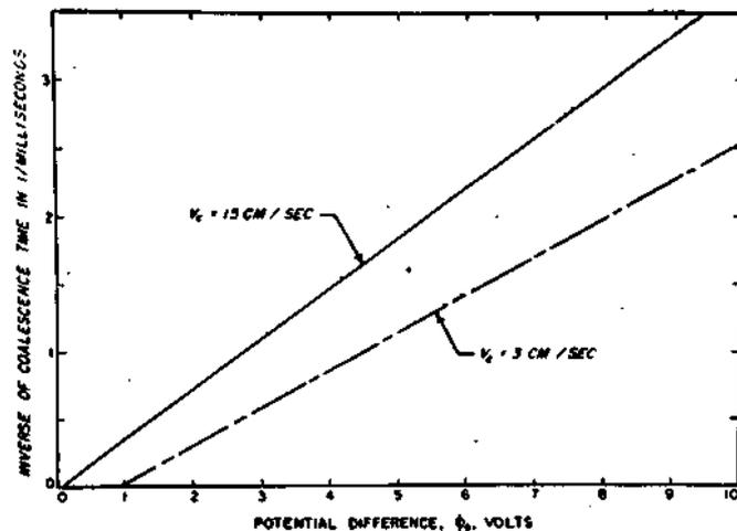
Fig. 4. Coalescence delay time as a function of voltage determined from collision profiles.
