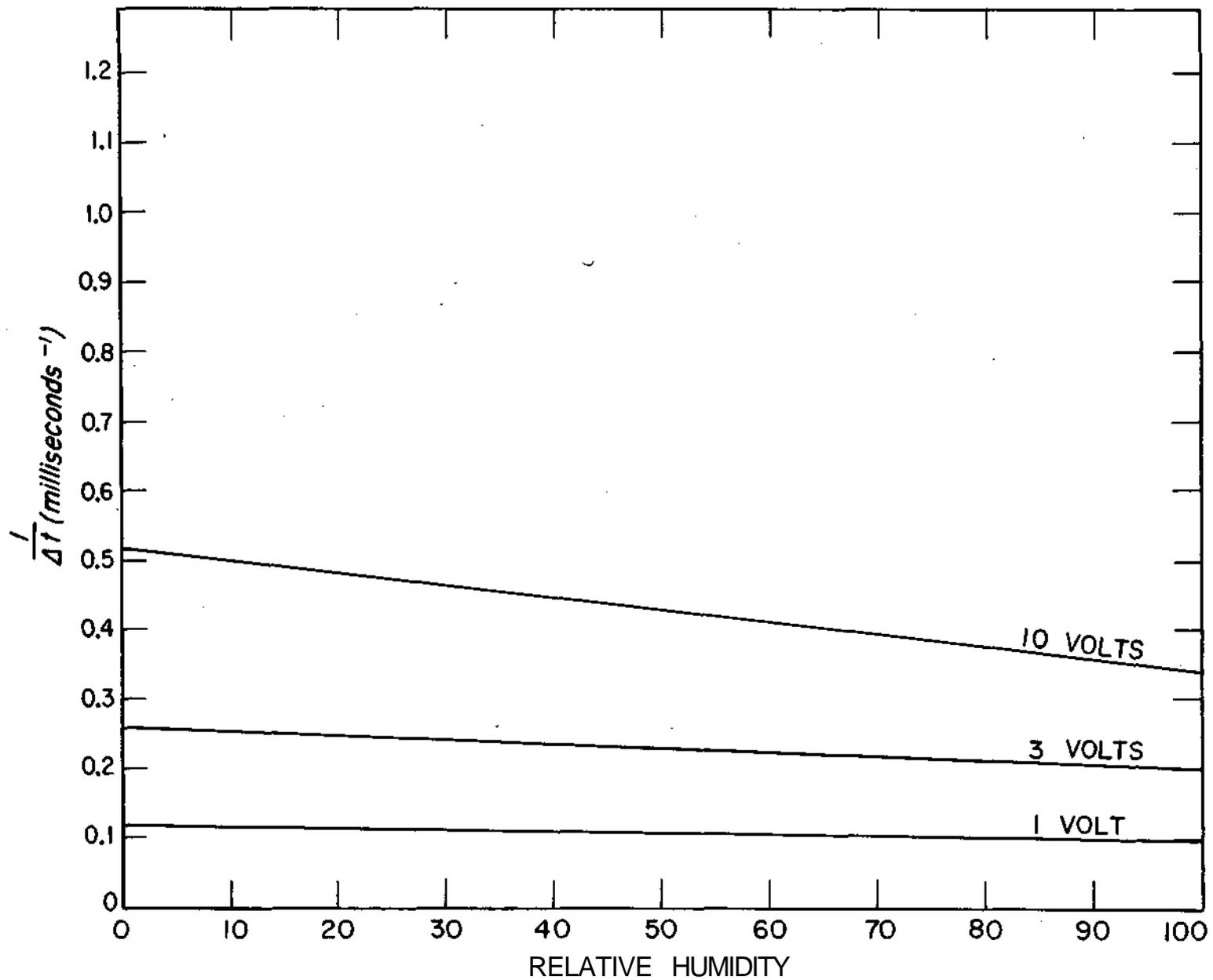
Figure 6. The inverse coalescence delay time versus relative humidity at 1, 3, and 10 volts and 18 cm/sec impact velocity.
