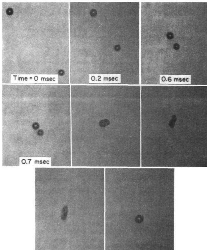
FIG. 5. The collision and coalescence of a  $96 \mu$  and a  $79 \mu$  droplet with opposite sign of charge.
