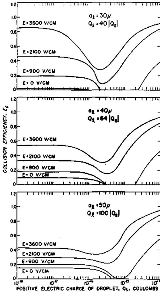
Fig. 5. Collision efficiency curves for a positively charged  $5\text{-}\mu$  droplet colliding with a  $30\text{-}\mu$ ,  $40\text{-}\mu$ , and  $50\text{-}\mu$  drop in electric fields oriented at  $= 90^\circ$ .
