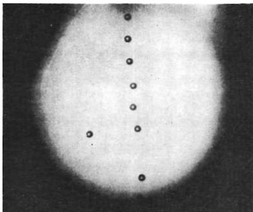
Figure 4. A charged droplet pulsed out of a stream of uncharged droplets.
