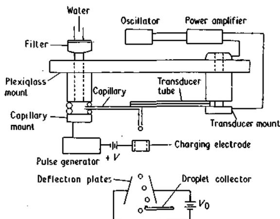
Figure 3. Schematic diagram of the experimental apparatus.
