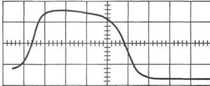
FIG. 4. Pulse from a charged droplet measured with the Faraday cage.
