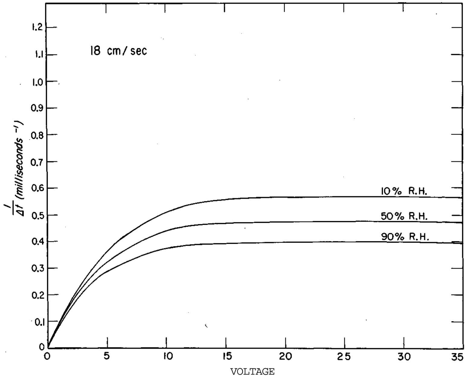
Figure 5. The inverse coalescence delay time versus voltage at relative humidities of 10, 50, and 90 percent and 18 cm/sec impact velocity.
