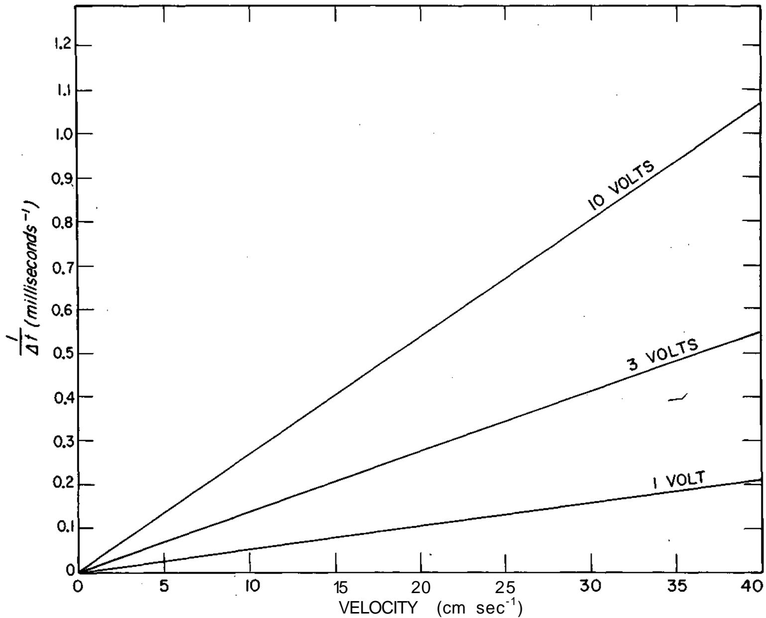
Figure 4. The inverse coalescence delay time versus impact velocity at 1, 3, and 10 volts and 10 percent relative humidity.
