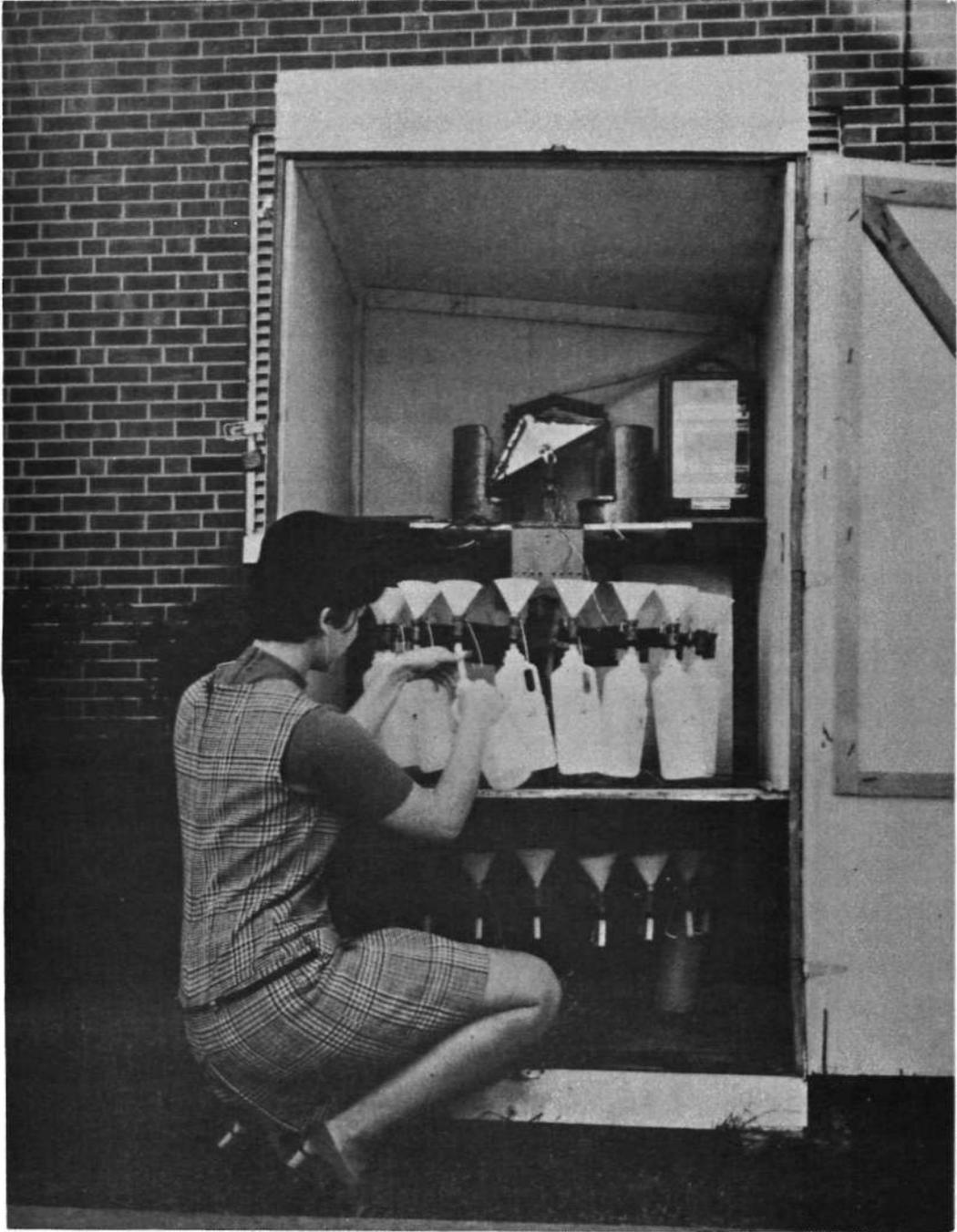
Figure 2. Sequential precipitation sampler
