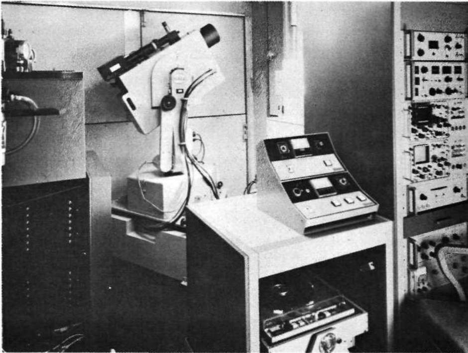
(b) MARK IX LIDAR AND ASSOCIATED RECORDING AND DISPLAY ELECTRONICS
