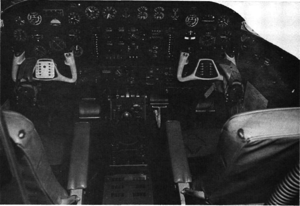
Figure 3. Cockpit of the University of Wyoming research aircraft showing aviation and navigational displays, X-band radar scope, and digital computer real-time display of meteorological parameters.
