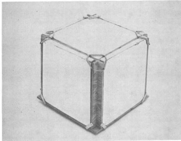
Figure 2. The Illinois State Water Survey hailcube.
