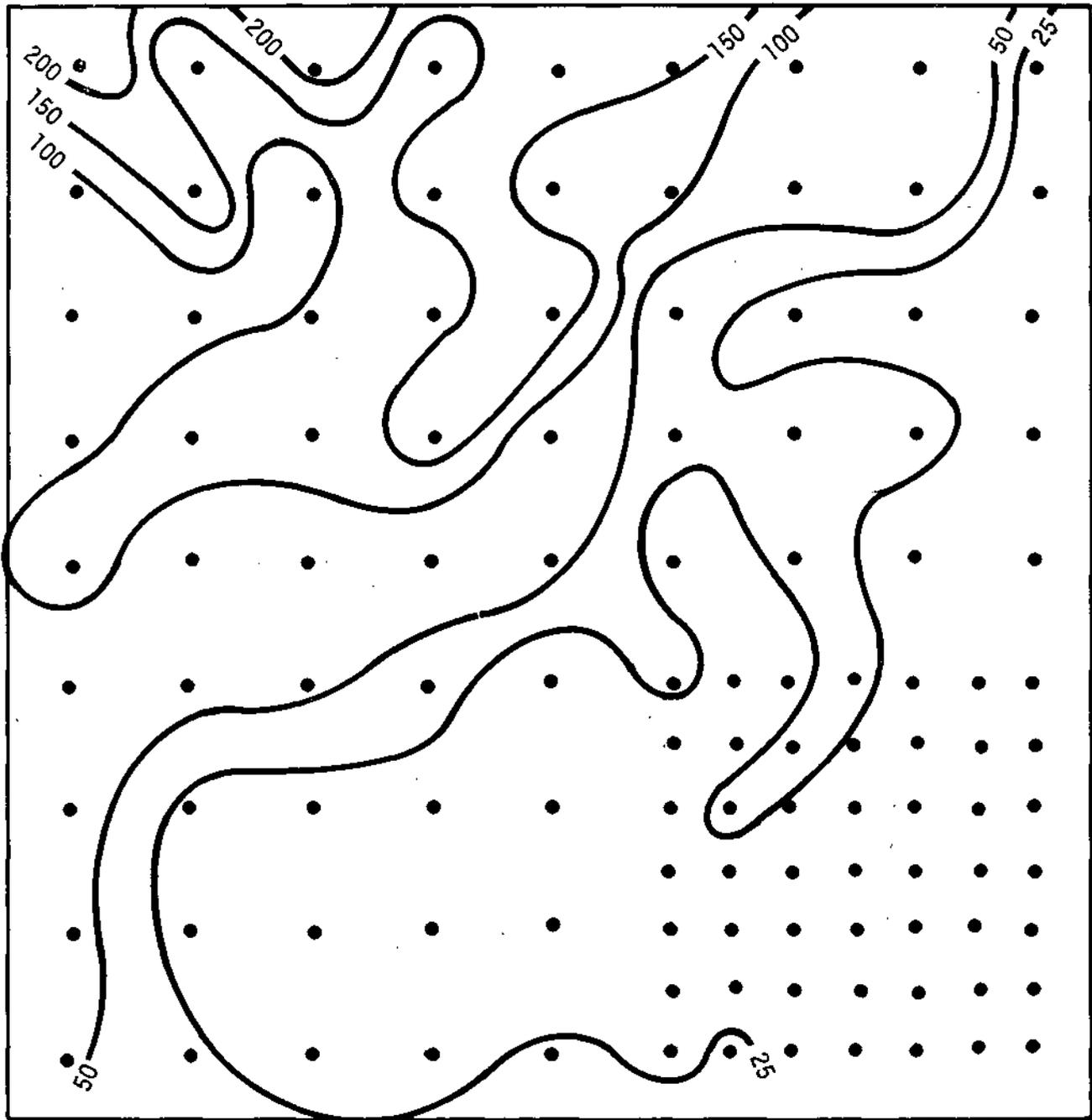
Figure 16. Distribution of vertical kinetic energy (joules/m<sup>2</sup>); storm of 22 July 1973.
