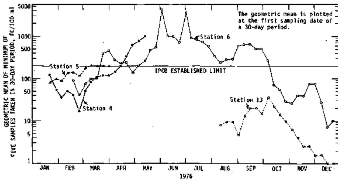
Figure 19. Geometric means of fecal coliform densities, stations 4, 5, 6, and 13
