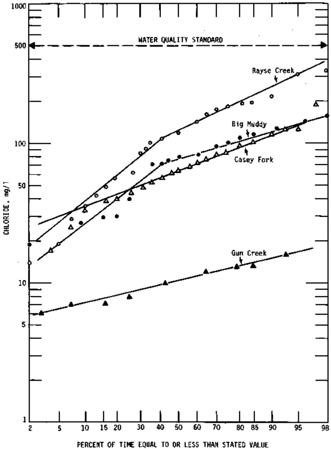
Figure 9. Distribution of chloride data for streams
