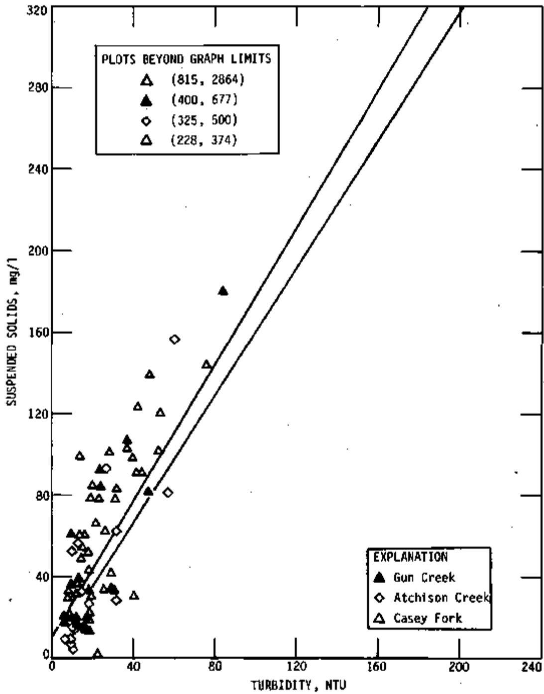
Figure 16. Relationship of suspended solids and turbidity for three streams
