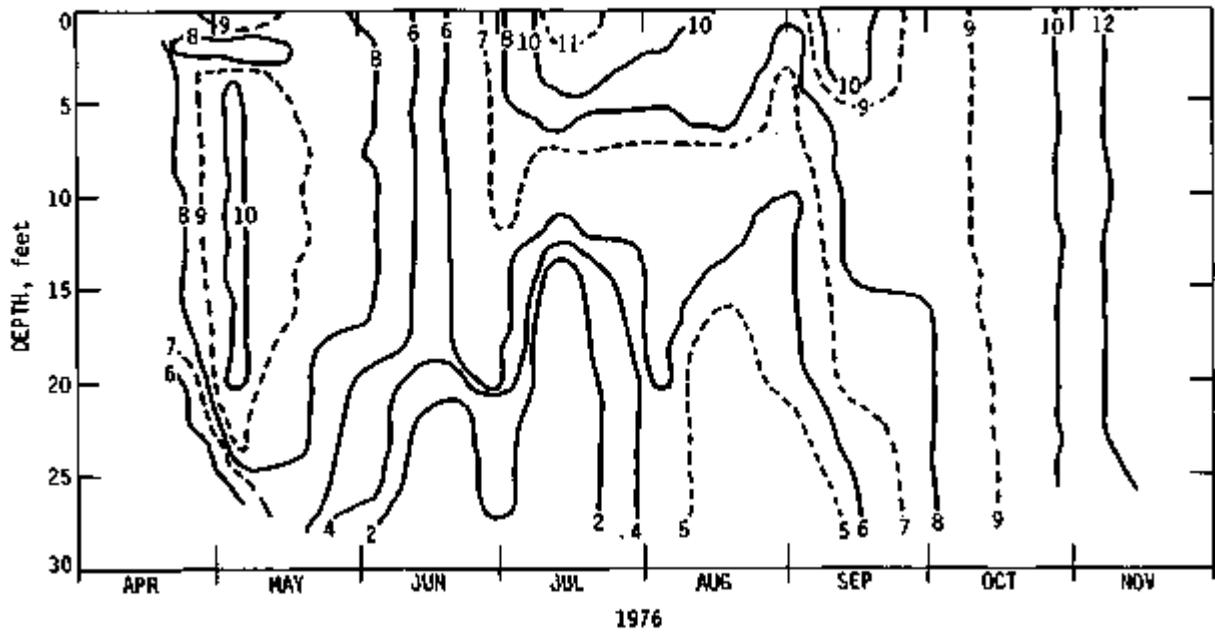
Figure 26. Isoleths of dissolved oxygen in Rend Lake, stations 9 and 12
