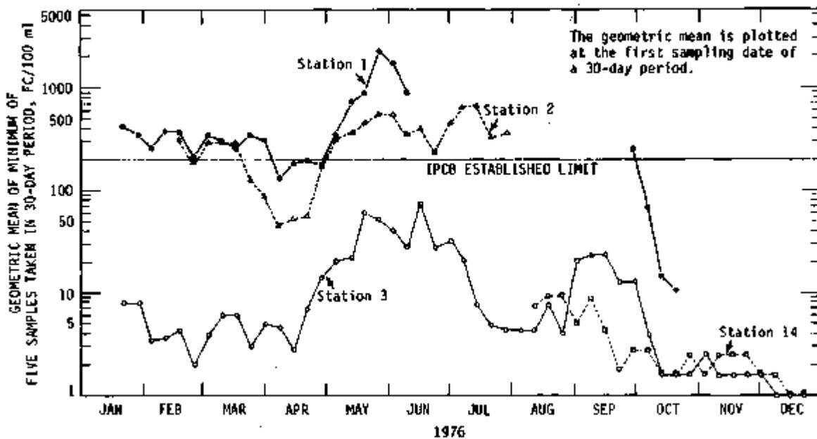
Figure 18. Geometric means of fecal coliform densities, stations 1, 2, 3, and 14
