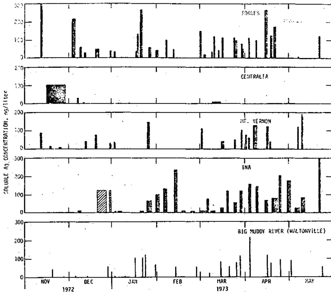
Figure 11. Silver Concentrations in Relation to Sampling Date. Adjacent Hatched Bars Indicate Separate Rain Periods in Same Sample.
