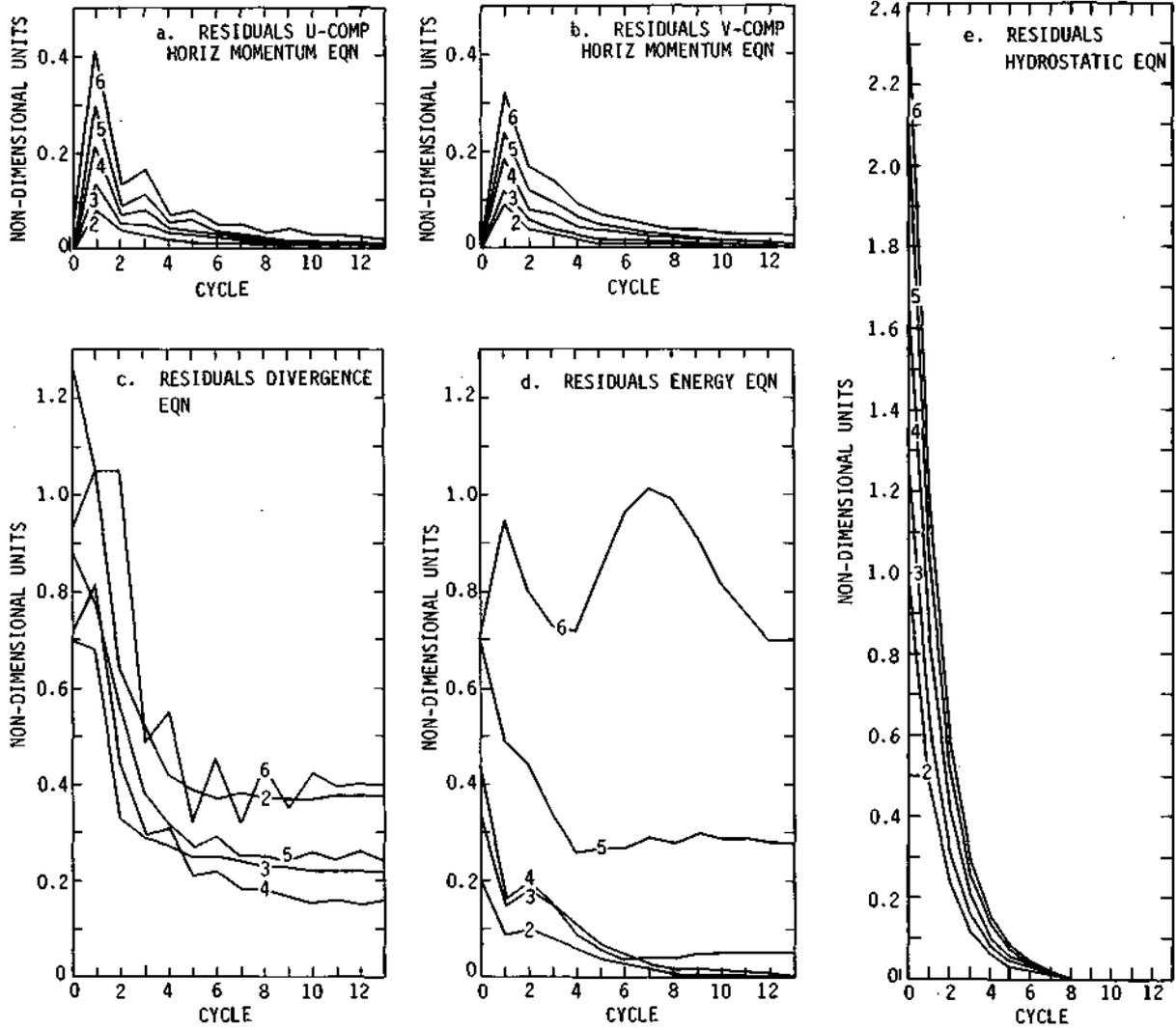
Figure 8. Root mean square residuals for the five adjustable sigma levels as a function of cycle for the five constraints.
