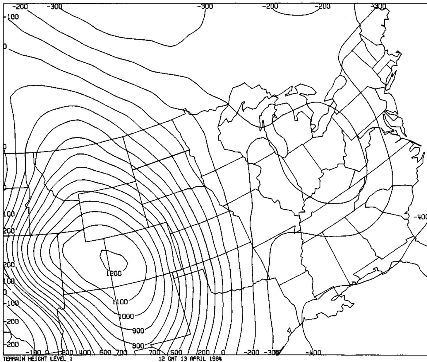
Figure 1. The smoothed surface topography that forms the lower boundary of the variational model. Heights are in departures from a reference value of 425 m.
