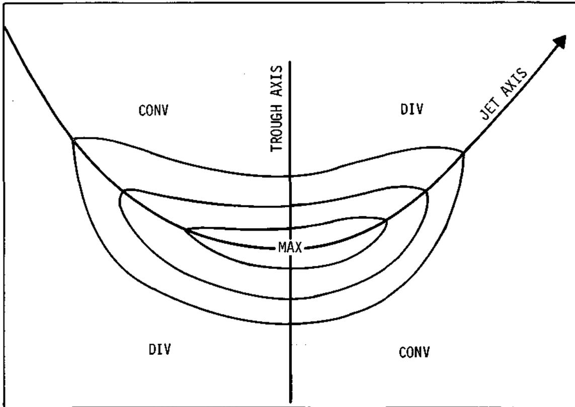
Figure 16. Illustration of the convergence pattern surrounding a strong wind maximum (jet maximum) embedded within a mid level trough.
