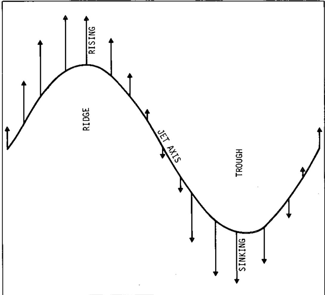
Figure 18. Illustration of magnitude and direction of vertical velocities along the axis of a jet stream that flows through a large scale ridge-trough pattern.
