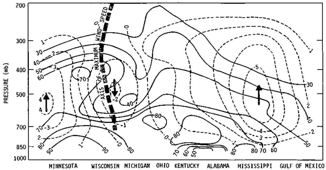
Figure 22. Vertical velocity (dashed lines) in  $\text{cm s}^{-1}$  and relative humidity along a vertical cross section constructed along a line approximately 200 km ahead of the cold front from Minnesota to the Gulf of Mexico.
