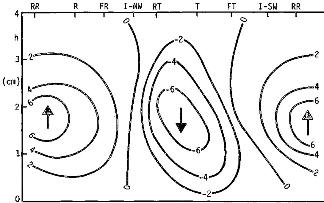
Figure 17. Vertical velocity ( $\text{cm s}^{-1}$ ) measured along the axis of a jet stream simulated by rotating tank experiments (from Reiter, 1961).
