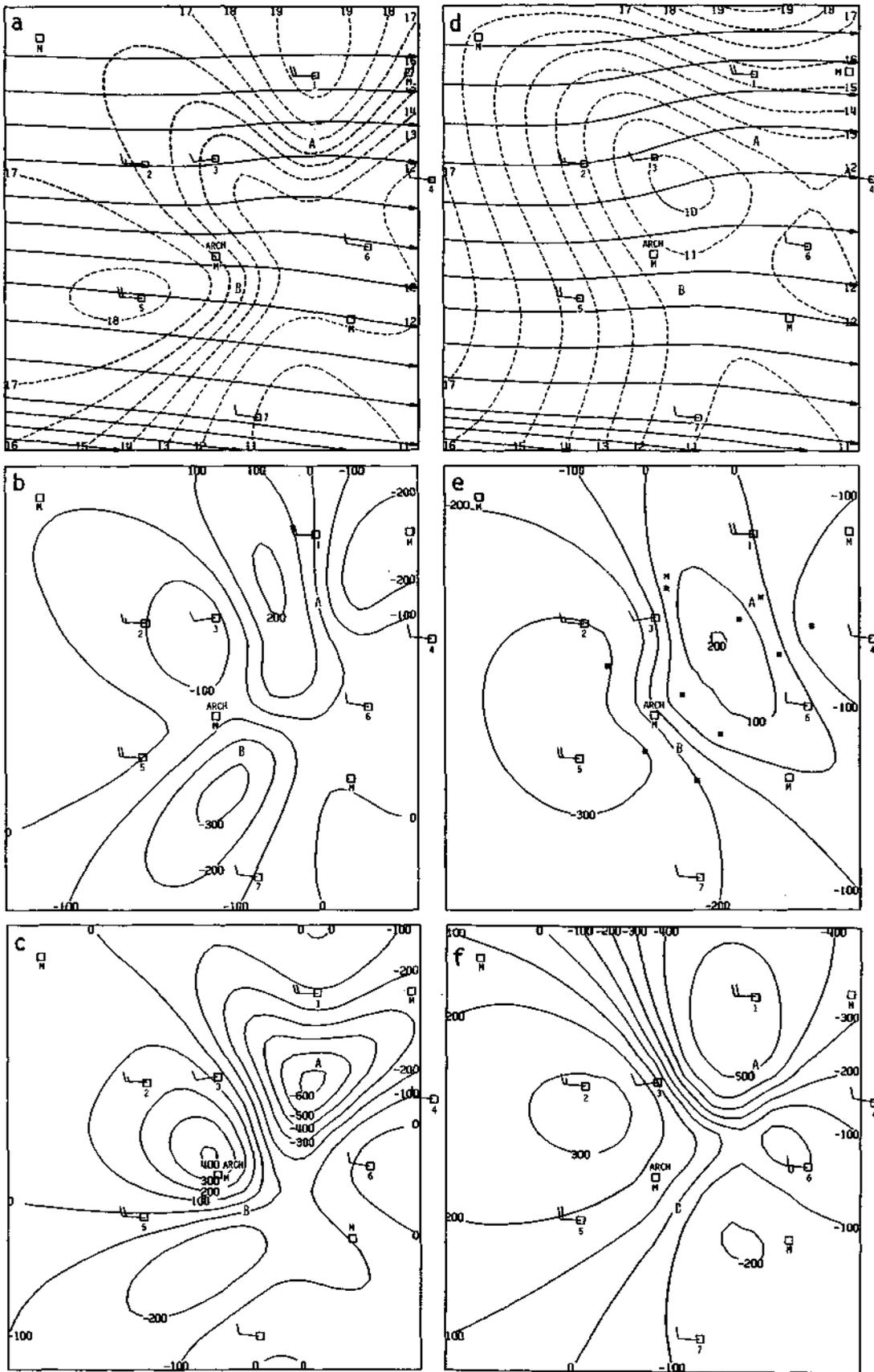
Figure 1. a) SC streamlines and isotachs, b) SC divergence, c) SC vorticity, d) LI streamlines and isotachs, e) LI divergence, and f) LI vorticity for the St. Louis area at 1600 m MSL, 1600 CST, 26 July 1973. Units are  $\text{m sec}^{-1}$  for isotachs and  $10^{-6} \text{ sec}^{-1}$  for divergence and vorticity.
