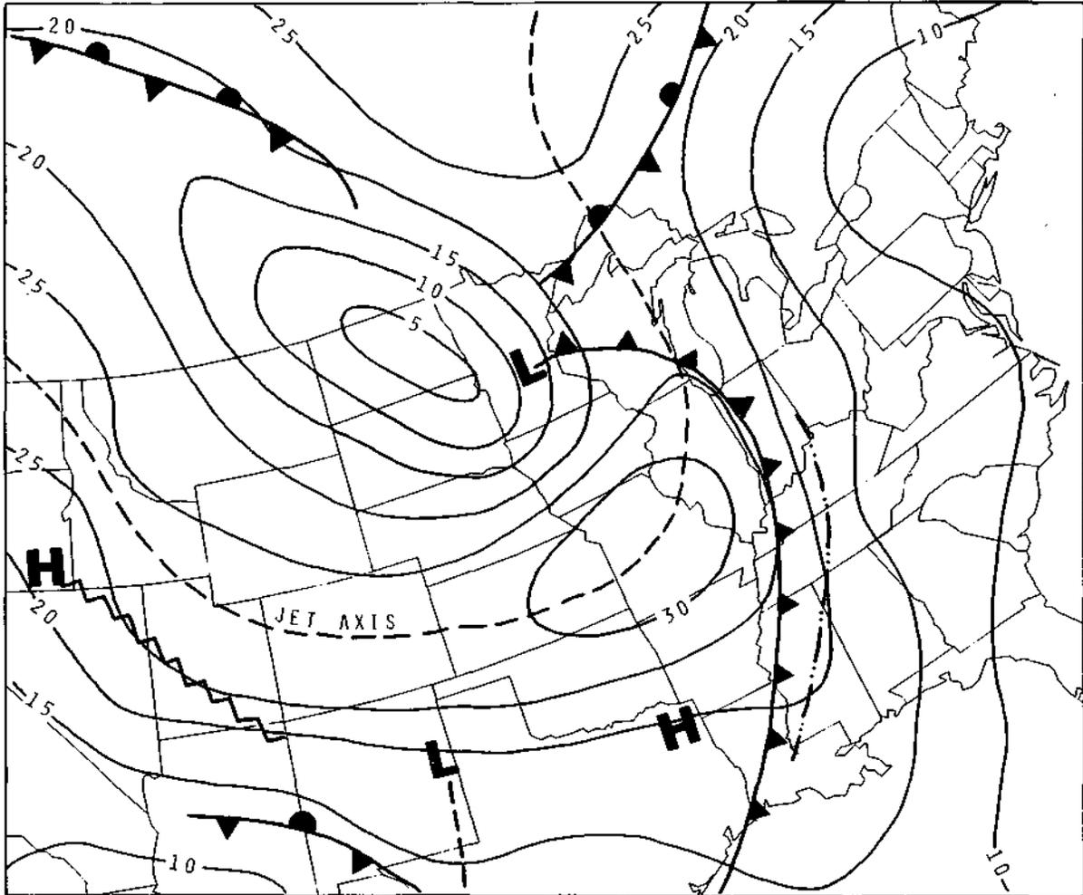
Figure 5. Isotachs ( $\text{m s}^{-1}$ ) of wind speed at 500 mb 12 GMT 13 April 1964.
