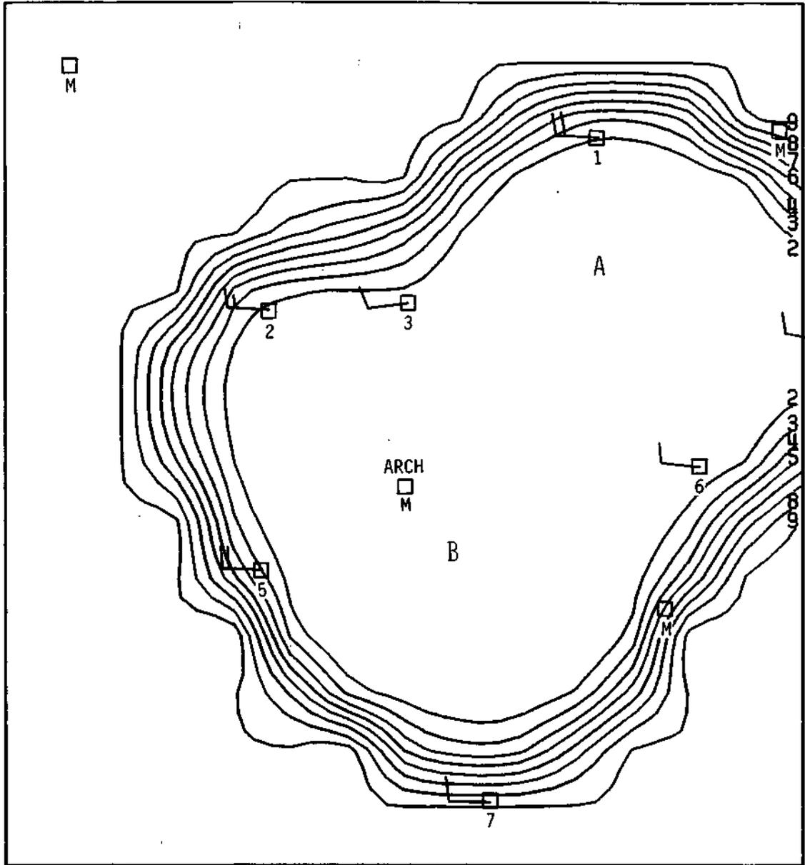
Figure 2. Distribution of the space function  $g(x,y)$  that weighted the SC and LI methods in the variational analysis.
