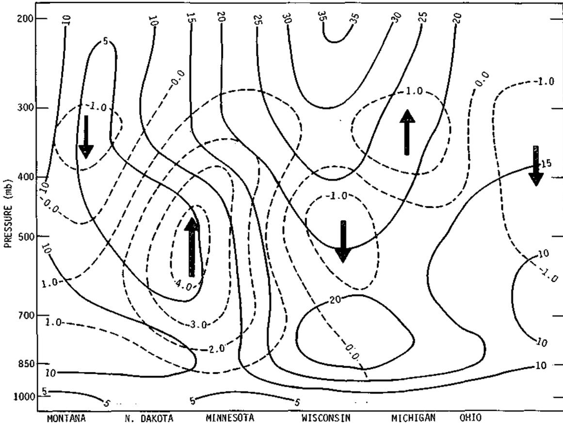
Figure 20. Vertical velocity (dashed lines) in  $cm s^{-1}$  and horizontal velocity (solid lines) in  $m s^{-1}$  along a vertical cross section constructed from Montana to Ohio through the mid tropospheric jet stream.
