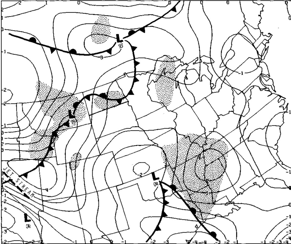
Figure 30. Summary of variational vertical velocity patterns, precipitation patterns (shaded) and the positions of low pressure centers and fronts for 00 GMT 12 April 1964.
