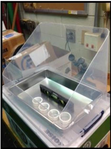
Table 1 shows the results from the experiment. After three days of placing the model under the sun for three hours, no water was collected in the beaker on the first two days and only 1.4 mL on the third. These results imply either a deficiency in the ability of the solar desalination model to capture the purified water or to evaporate effectively the water solution in the container inside of it.
