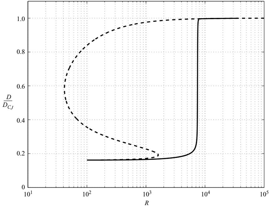
FIGURE 8. Detonation initiation by a weak source for a mixture with  $\gamma = 1.2$ ,  $Q = 50$ ,  $E = 13$ . Solid line is a quasi-steady  $D$ - $R$  curve and dashed line is a solution of the  $\dot{D}$ - $D$ - $\kappa$  equation with initial conditions  $D_0 = 1.101$ ,  $R_0 = 100$ .
