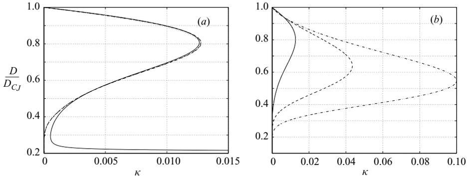
FIGURE 3. (a)  $D$ - $\kappa$  curves for  $\gamma=1.2$ ,  $Q=30$ ,  $E=20$  for several reaction orders,  $\nu=1/2$  (solid),  $\nu=2/3$  (dashed),  $\nu=3/4$  (dash-dot), and  $\nu=1$  (dotted). (b)  $D$ - $\kappa$  curves for  $\nu=1$ ,  $Q=30$ ,  $E=20$  for several  $\gamma$ :  $\gamma=1.2$  (solid),  $\gamma=1.4$  (dashed), and  $\gamma=1.6$  (dash-dot).
