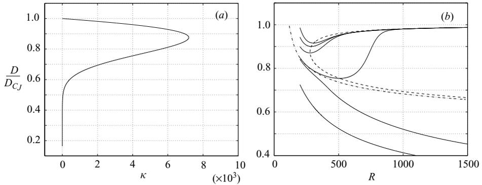
FIGURE 5. (a)  $D$ - $\kappa$  curve for detonation in an ideal gas with  $\gamma = 1.25$ ,  $Q = E = 40$ . (b) Ignition and failure. Dashed line is the quasi-steady  $D$ - $R$  curve, dash-dot line is the ignition separatrix, and solid lines are solutions of equation (74) with initial conditions given by  $R_0 = 200$  and various  $D_0$ :  $D_0 = 6.8, 6.5, 6.2, 5.85, 5.84$  and  $5.0$  from top to bottom.
