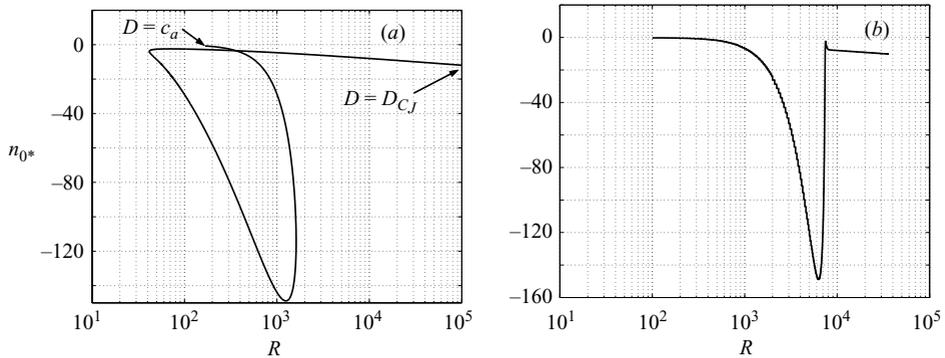
FIGURE 9. (a) The sonic locus along the quasi-steady  $D$ - $R$  curve and (b) the sonic locus for weak ignition, both of figure 8.
