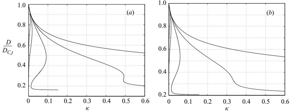
FIGURE 2.  $D$ - $\kappa$  curves for  $\nu=1$ ,  $\gamma=1.2$ , and (a)  $Q=50$  and (b)  $Q=30$  for various activation energies:  $E=0, 5, 10, 20$  and  $30$ .  $E$  increases from right to left on each figure.
