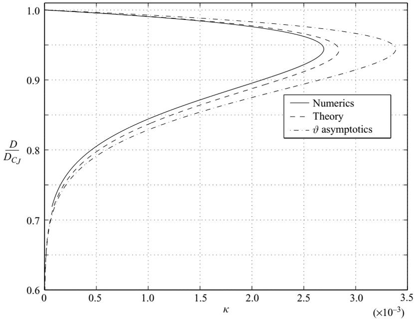
FIGURE 4. Comparison of the theory, large-activation-energy  $\vartheta$  asymptotic version of the theory, and numerically computed  $D$ - $\kappa$  curves for  $\gamma = 1.2$ ,  $E = 50$ , and  $Q = 30$ .
