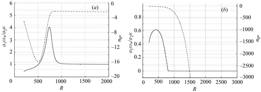
FIGURE 6. Position of the sonic locus,  $n_{0*}$  (dashed line), and the ratio of the heat release term,  $a_1\omega_*$ , to the curvature term,  $a_2\kappa$ , in equation (74) (solid line), during successful (a) ignition and (b) failure for detonation in an ideal gas with  $\gamma = 1.25$ ,  $Q = E = 40$ . (a)  $R_0 = 200$ ,  $D_0 = 5.85$ ; (b)  $R_0 = 200$ ,  $D_0 = 5.841$ .
