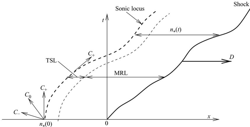
FIGURE 1.  $x$ - $t$  diagram of the shock locus and the sonic locus in self-sustained one-dimensional planar detonation.
