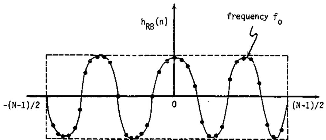
Figure 8. Unit pulse response for a rectangular bandpass filter.
