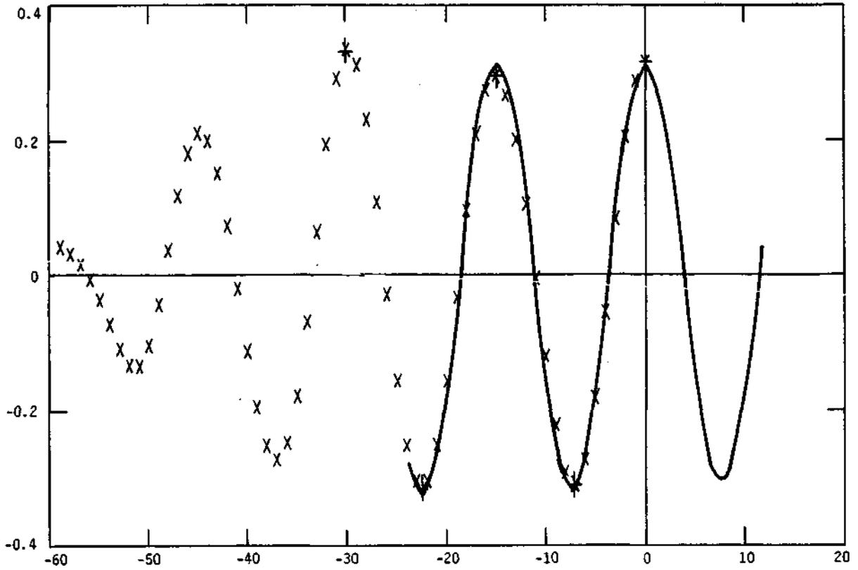
Figure 15. Output of the 15-year filter with an 8-year and 15-year component in the input (nonrecursive).
