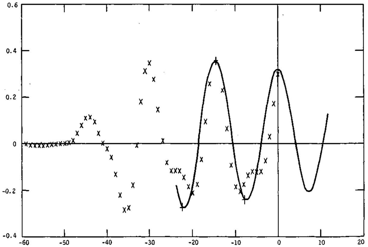
Figure 18. Output of the 15-year recursive filter ( $w_2 - w_1 = 0.05$ ) with 8 and 15-year input components.
