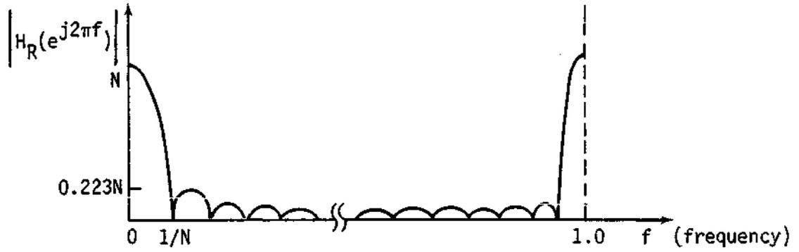
Figure 5. Frequency response of the rectangular lowpass filter.
