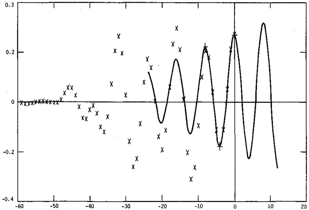
Figure 20. Output of the 8-year filter (recursive with  $w_2 - w_1 = 0.05$ ) for 8 and 15-year input components.
