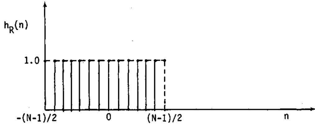
Figure 4. Unit pulse of a rectangular lowpass filter.
