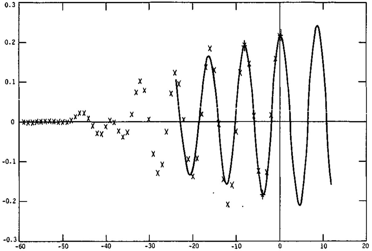
Figure 19. Output of the 8-year filter with 8 and 15-year input components.
