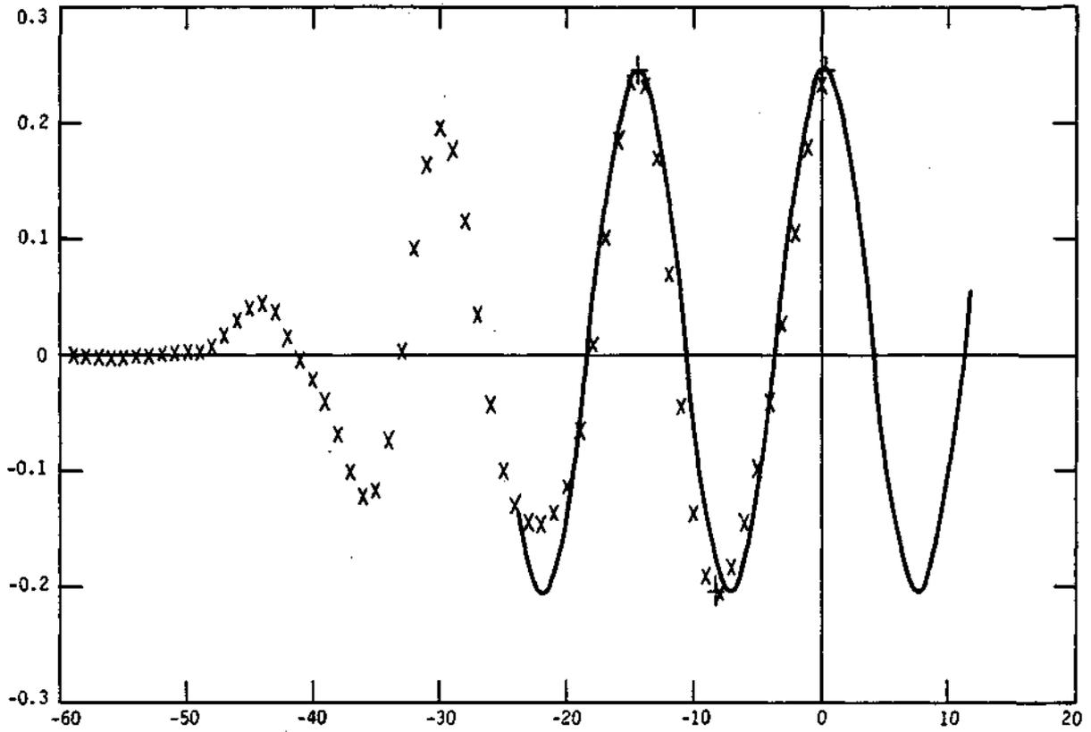
Figure 17. Output of the 15-year recursive filter ( $w_2 - w_1 = 0.015$ ) for 8 and 15-year input components.
