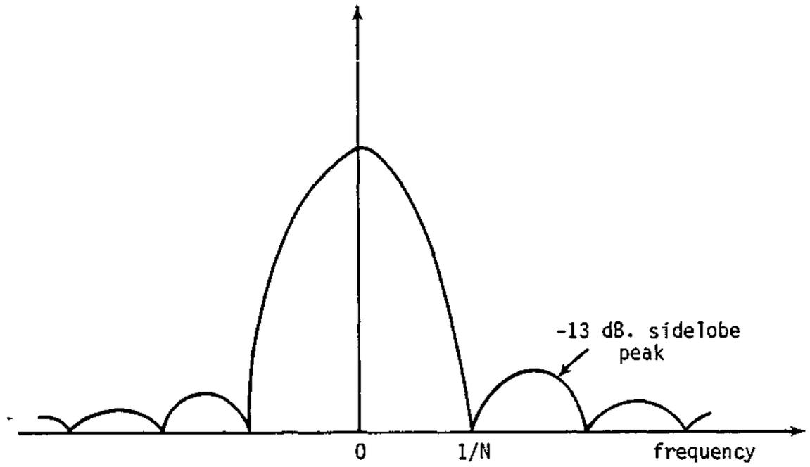
Figure 1. Frequency response of the  $k = 0$  filter in the Fast Fourier Transform.
