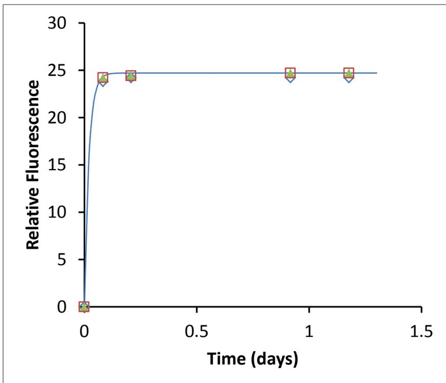
**Figure C-6. Kinetics of extraction of pyrene from silicone.**
