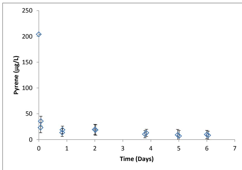
**Figure C-1. Kinetics of pyrene sorption to corn stover char CS450. Overlapping symbols offset in the x direction for clarity. Error bars show 95% confidence intervals.**
