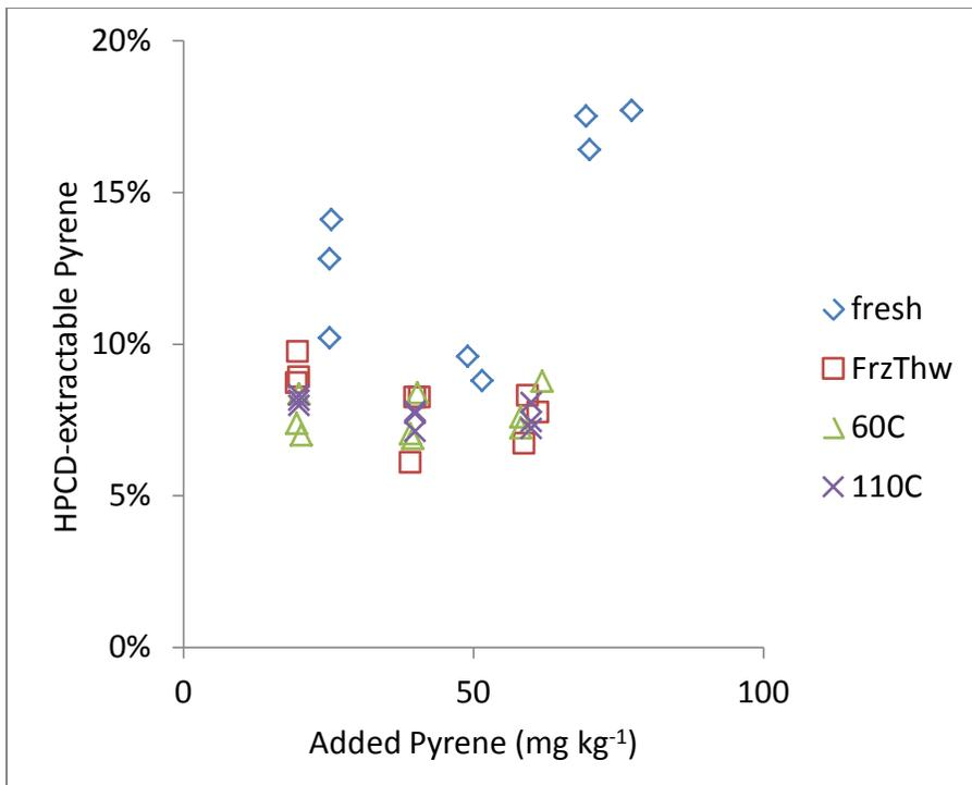
Figure 15. HPCD-extractable pyrene in spiked CS450 biochar.
