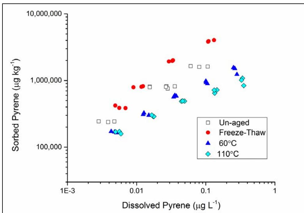
Figure 14. Pyrene sorption to un-aged and artificially aged CS750 biochar.
