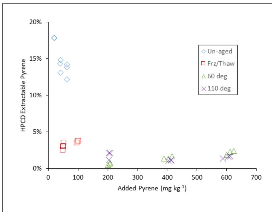
Figure 16. HPCD-extractable pyrene in spiked CS550 biochar.
