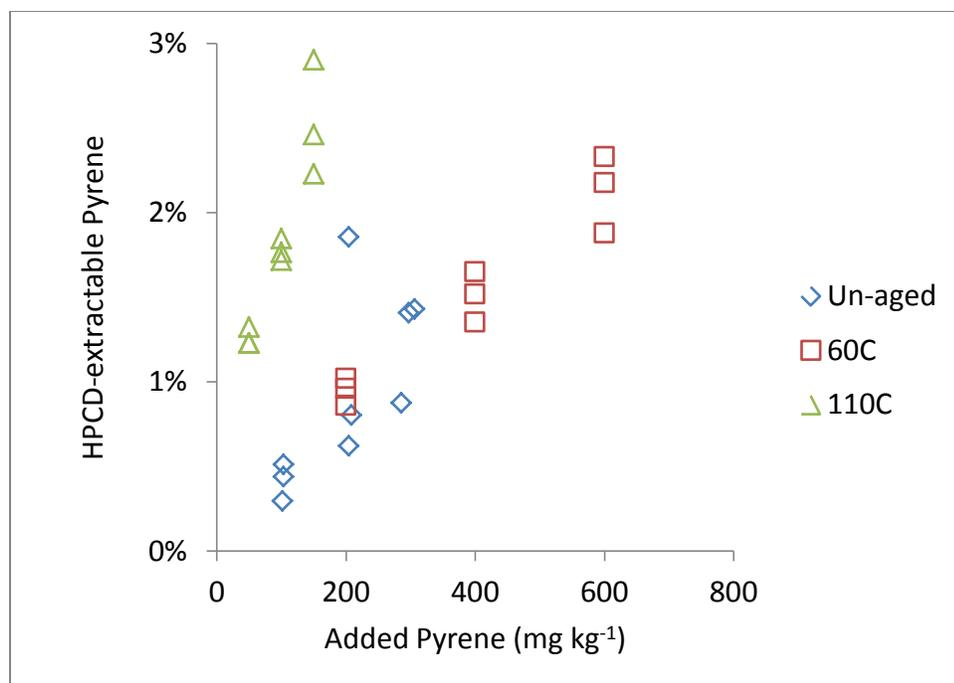
**Figure 17. HPCD-extractable pyrene in spiked CS750 biochar.**
