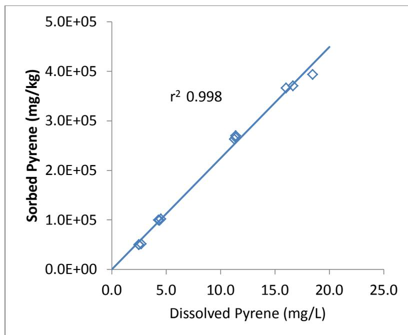
**Figure C-4. Isotherm for pyrene partitioning to POM.**
