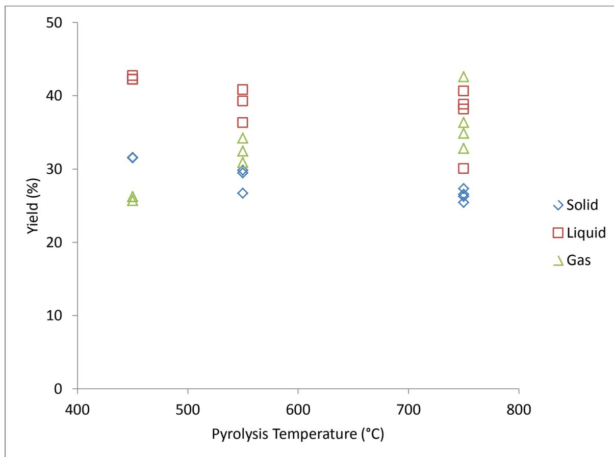
**Figure 1. Yields of solid (biochar), liquid, and non-condensable gas from corn stover pyrolysis.**
