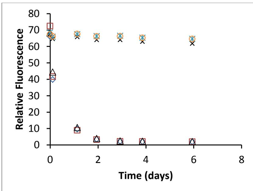
**Figure C-5. Pyrene-silicone partitioning kinetics. Different symbols are used to show replicates.**
