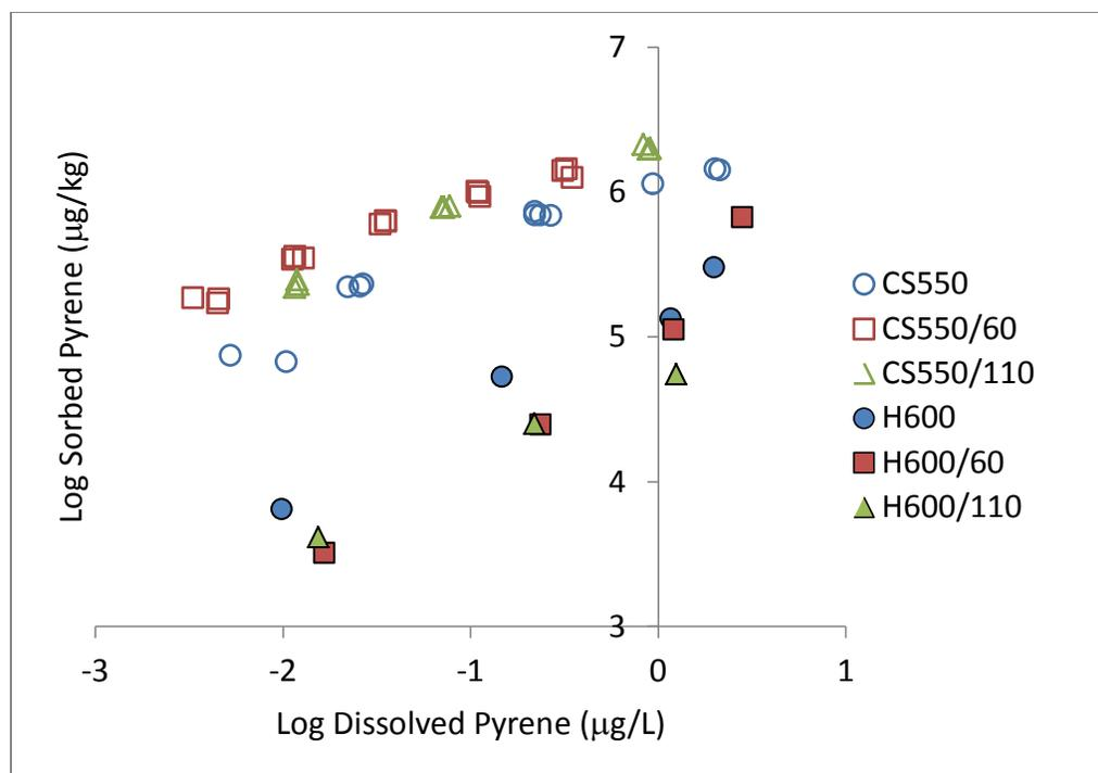
**Figure 19. Comparison of pyrene sorption isotherms of slow pyrolyzed corn stover biochar. Open symbols - present work. Filled symbols - Hale et al. (2011).**
