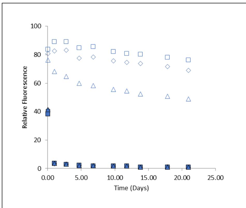
**Figure C-2. Kinetics of partitioning of pyrene to POM. Different symbols are used to show replicates. Open symbols are for bottles with POM, filled symbols are for bottles with no POM.**
