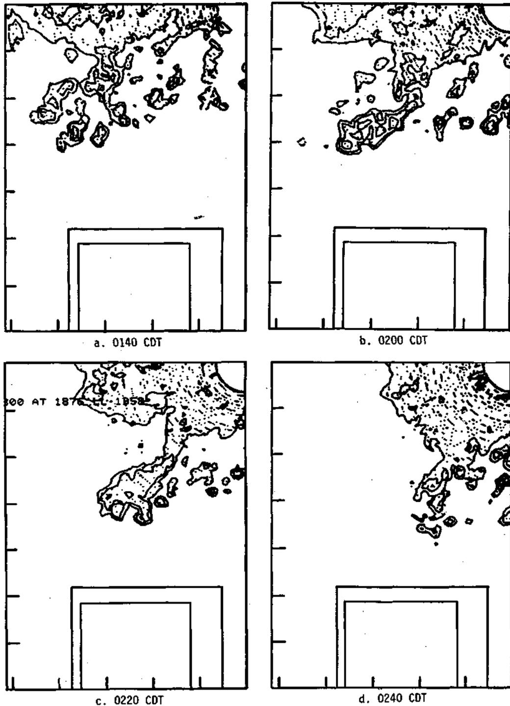
Figure 3. Radar echoes from the "HOT" radar in Joliet, IL on 9 August 1979. The radar was located in the upper right corner. Tic marks along the axes are every 25 km. The radar beam elevation is at  $2.2^\circ$ . Reflectivity contours are 10 dbz intervals with 30 dbz threshold. The larger box represents the approximate boundary of the rain gage network while the smaller box outlines the wind site locations.
