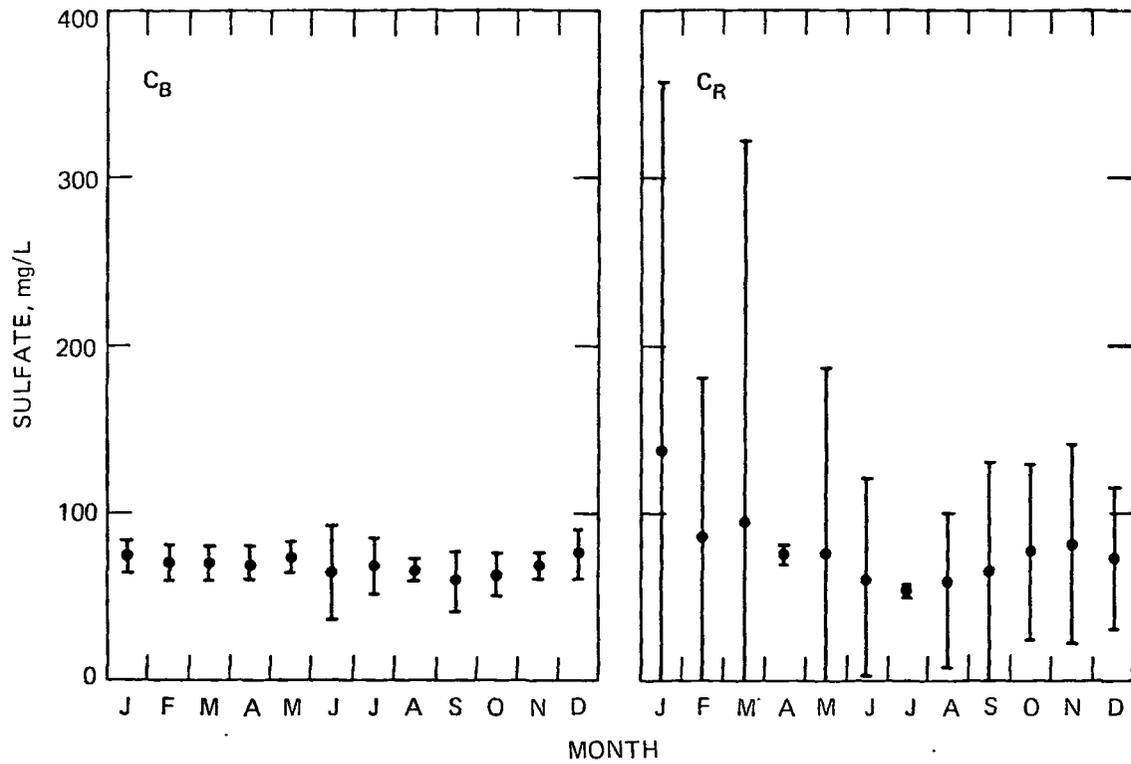
Figure 23. Monthly average sulfate concentrations in base flow and surface runoff.
