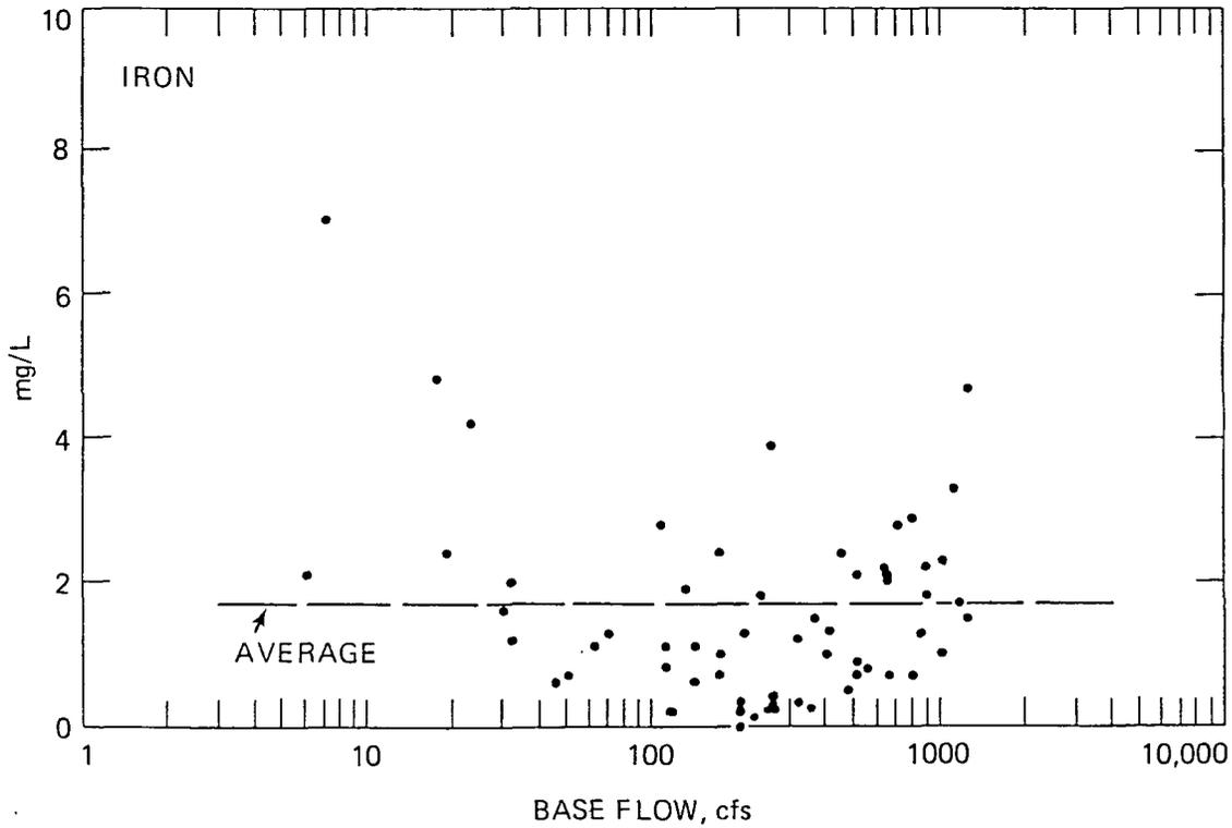
Figure 14. Base flow-chemical data relationship for total iron.
