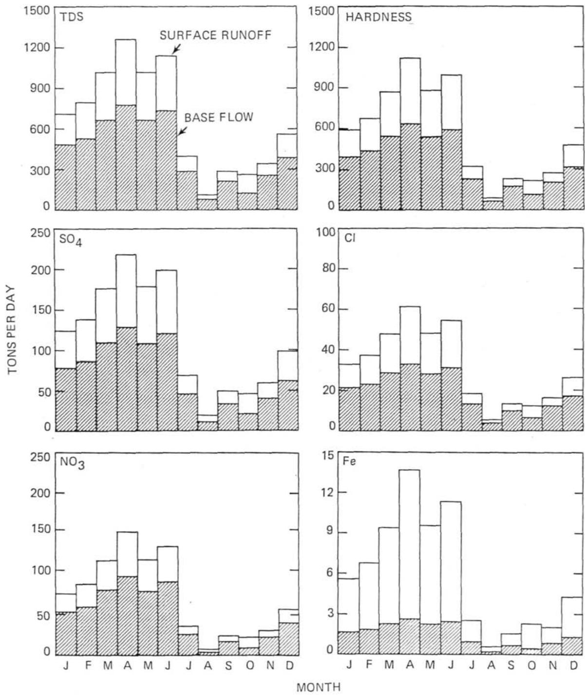
Figure 27. Monthly average chemical loadings for TDS, hardness, sulfates, chlorides, nitrates, and total iron.
