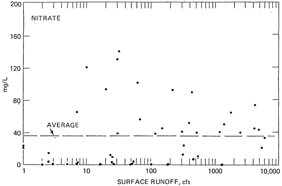
Figure 19. Surface runoff-chemical data relationship for nitrate.
