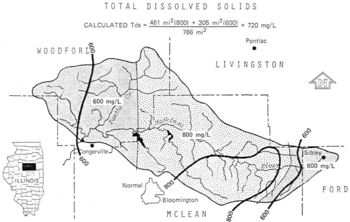
Figure 3. Shallow groundwater total dissolved solids.
