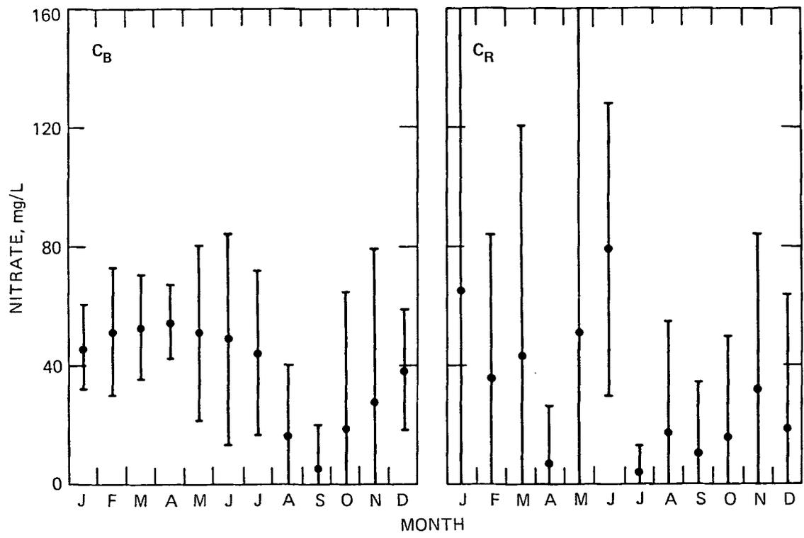
Figure 25. Monthly average nitrate concentrations in base flow and surface runoff.
