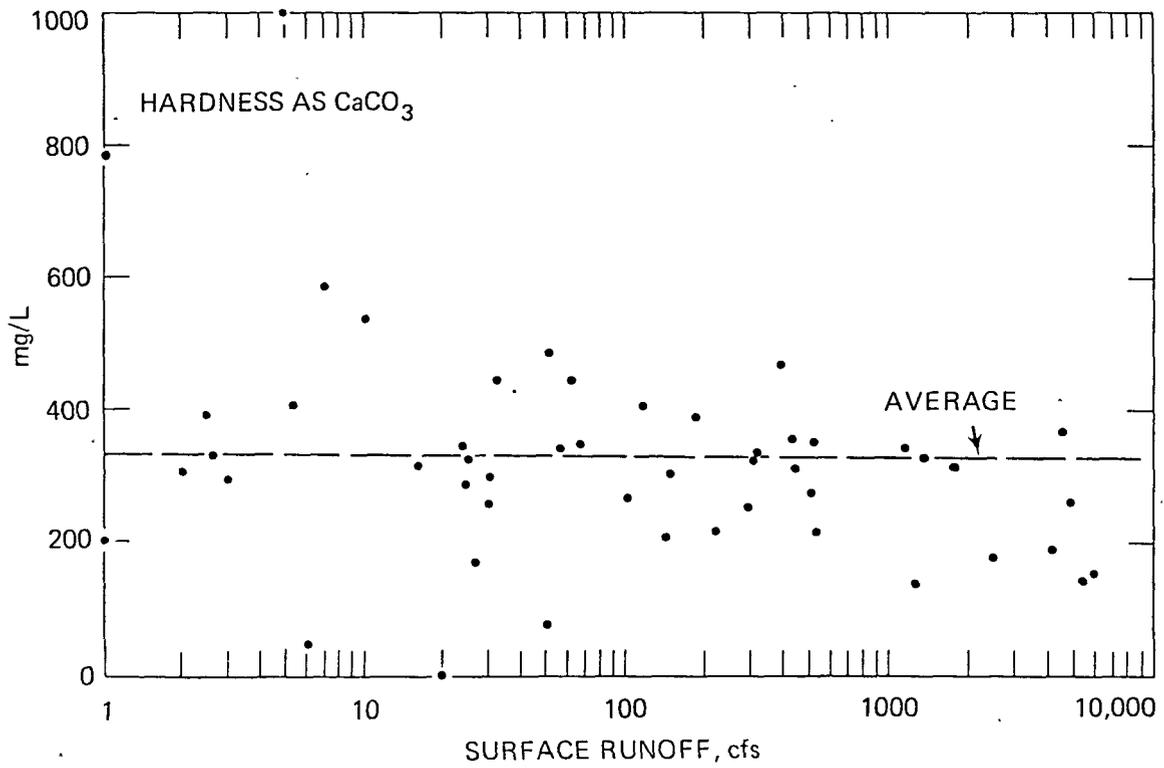
Figure 16. Surface runoff-chemical data relationship for hardness.
