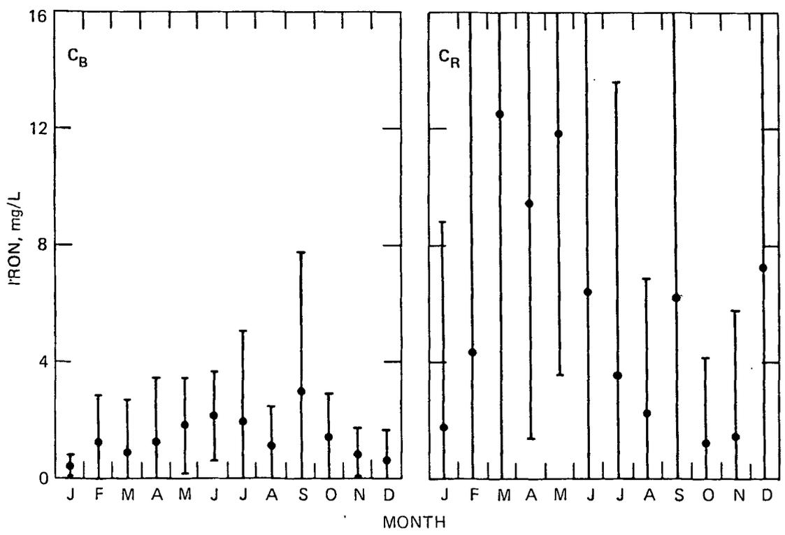
Figure 26. Monthly average total iron concentrations in base flow and surface runoff.
