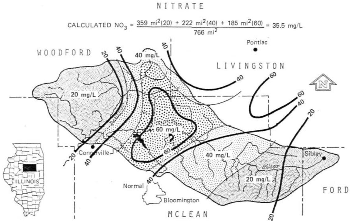
Figure 7. Shallow groundwater nitrates.
