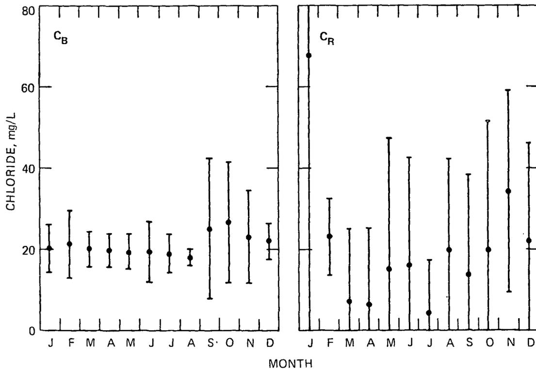
Figure 24. Monthly average chloride concentrations in base flow and surface runoff.
