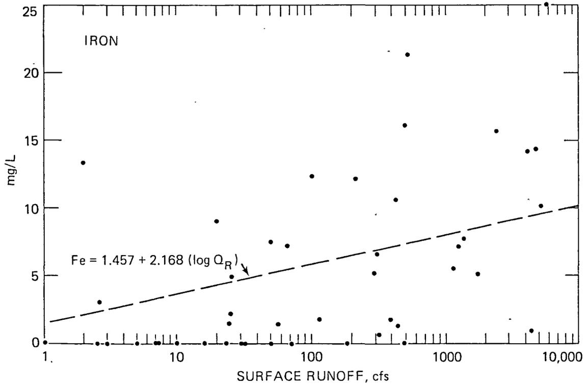
Figure 20. Surface runoff-chemical data relationship for total iron.
