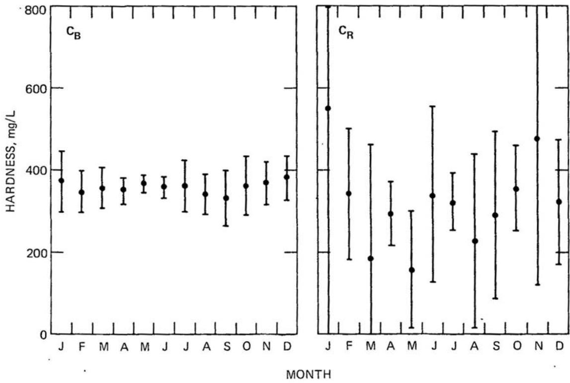
Figure 22. Monthly average hardness concentrations in base flow and surface runoff.
