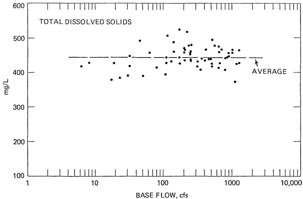
Figure 9. Base flow-chemical data relationship for total dissolved solids.
