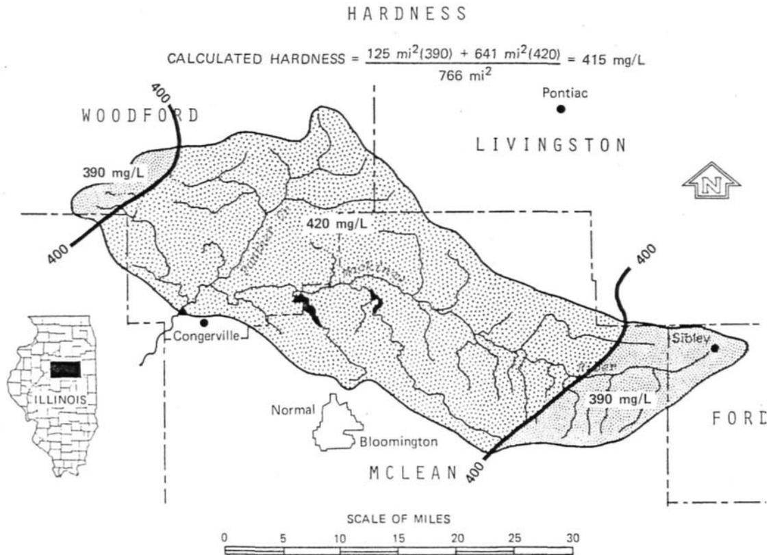
Figure 4. Shallow groundwater hardness.
