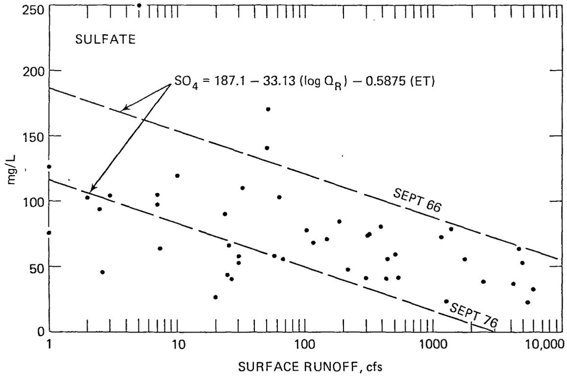
Figure 17. Surface runoff-chemical data relationship for sulfate.
