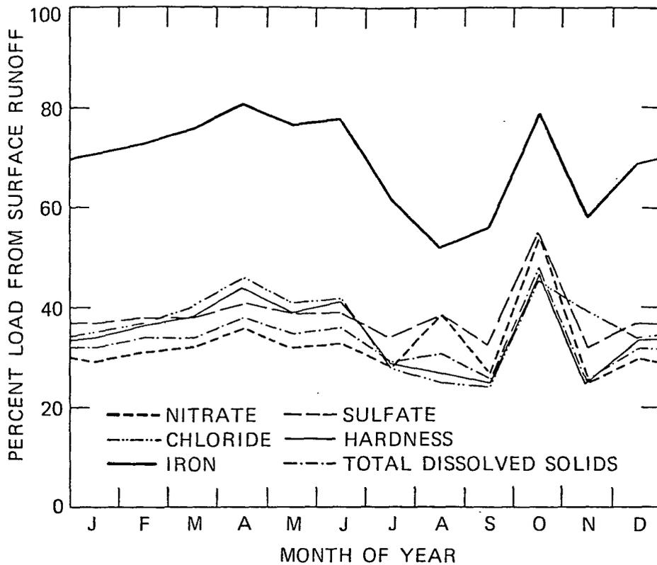
Figure 28. Percent of total chemical load contributed by surface runoff.
