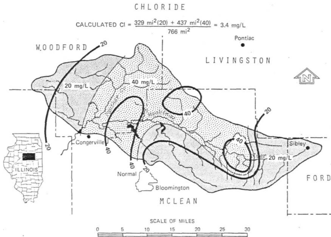
Figure 6. Shallow groundwater chlorides.
