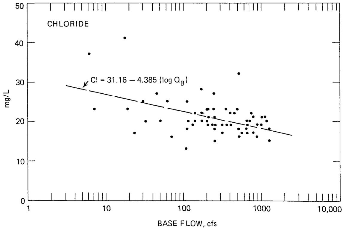
Figure 12. Base flow-chemical data relationship for chloride.
