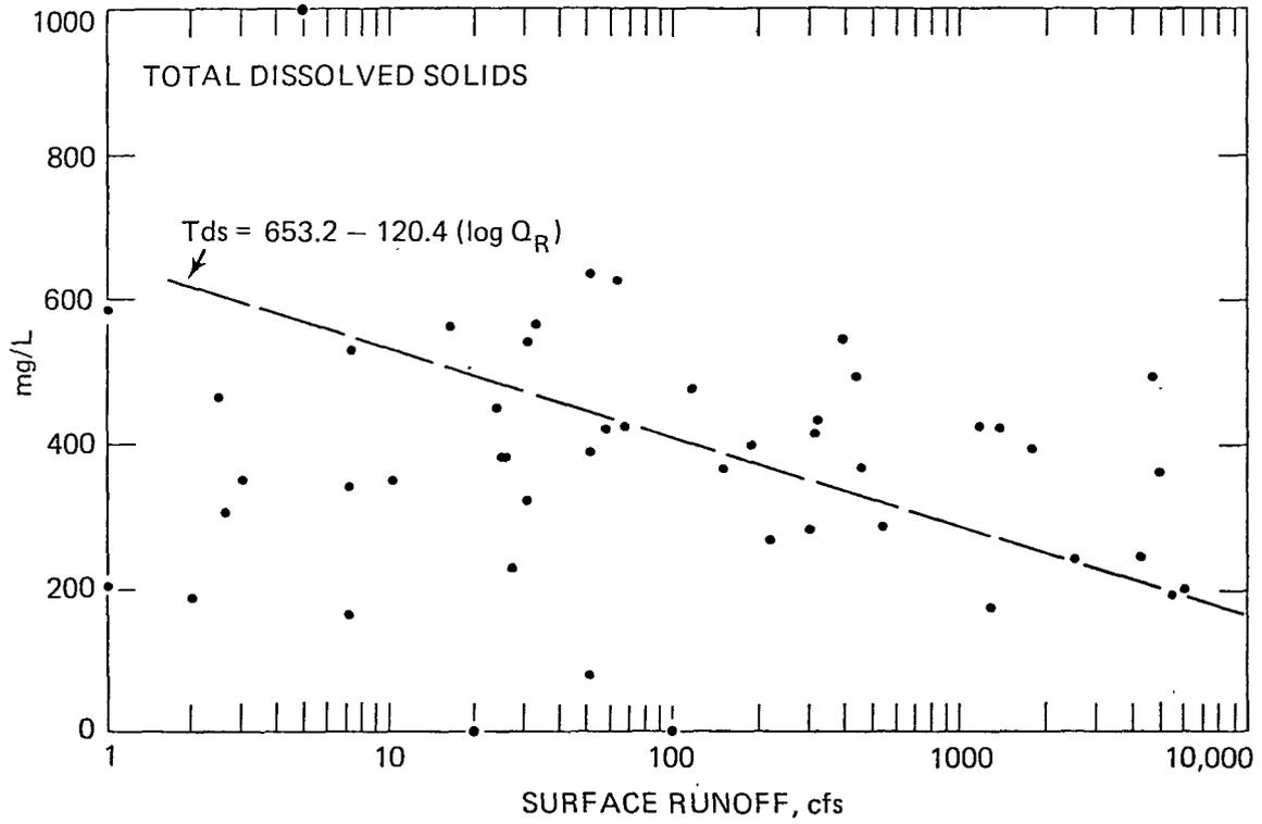
Figure 15. Surface runoff-chemical data relationship for total dissolved solids.
