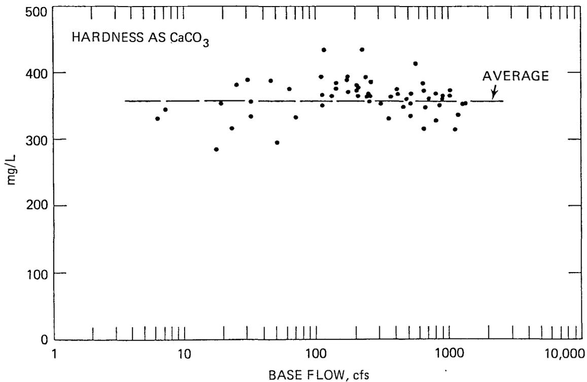
Figure 10. Base flow-chemical data relationship for hardness.
