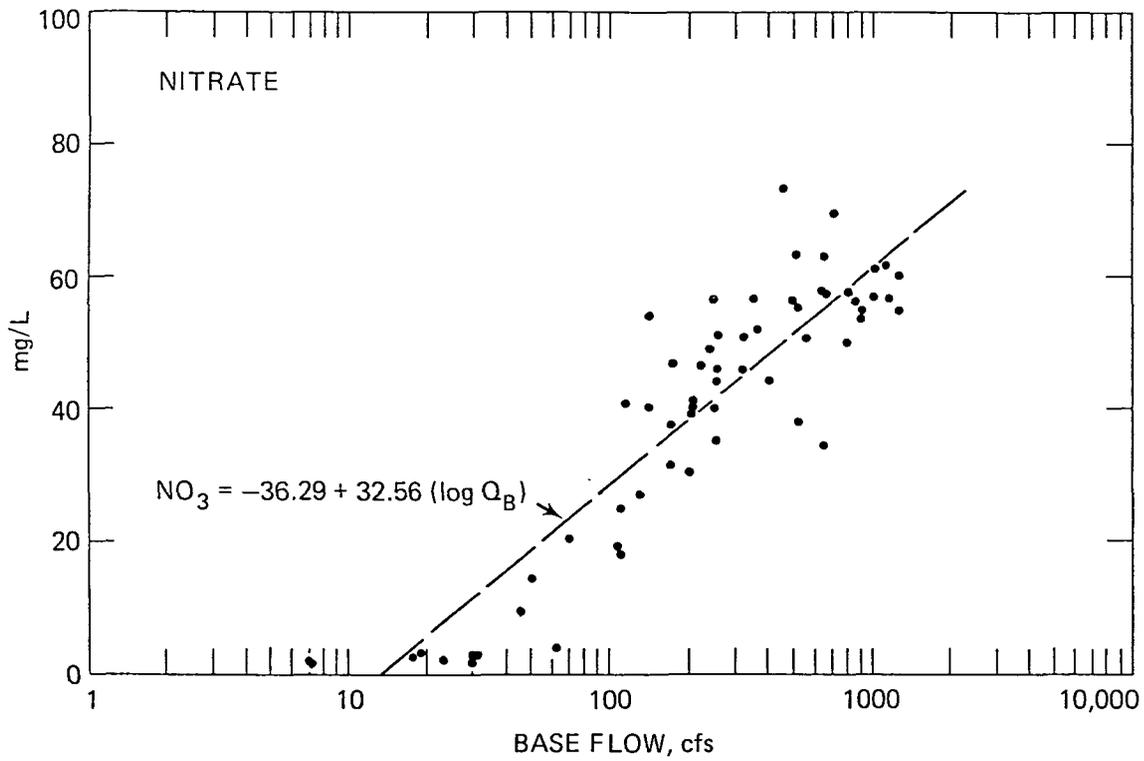
Figure 13. Base flow-chemical data relationship for nitrate.
