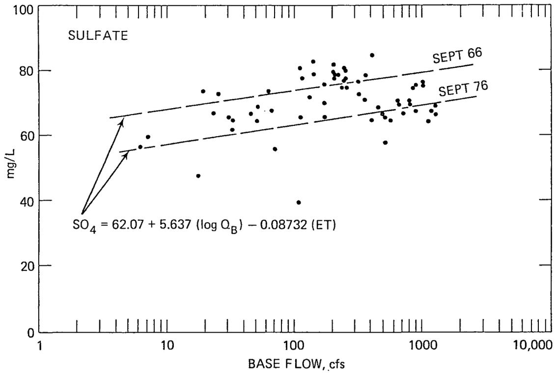
Figure 11. Base flow-chemical data relationship for sulfate.
