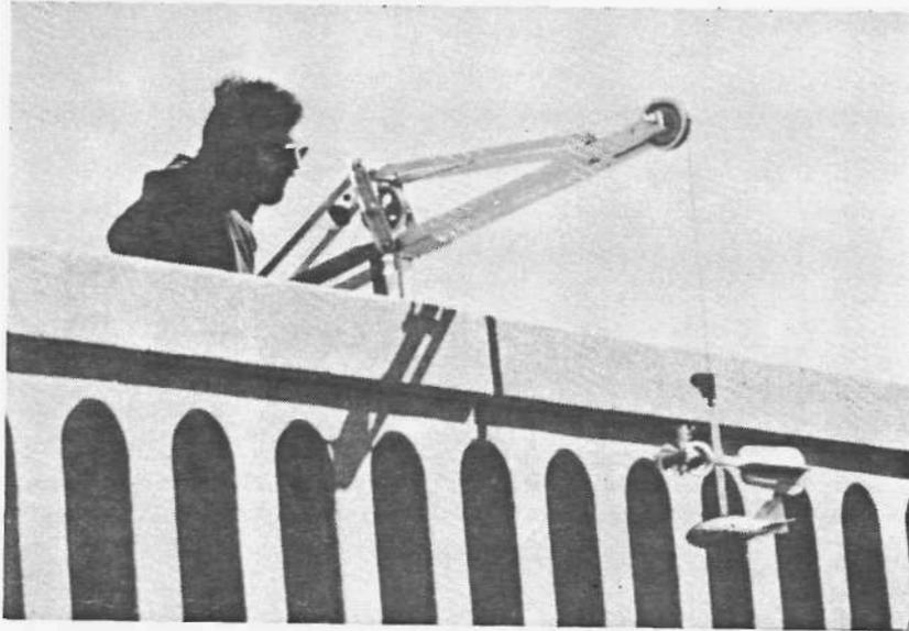
Figure 11. Technician using current meter to measure stream discharge
