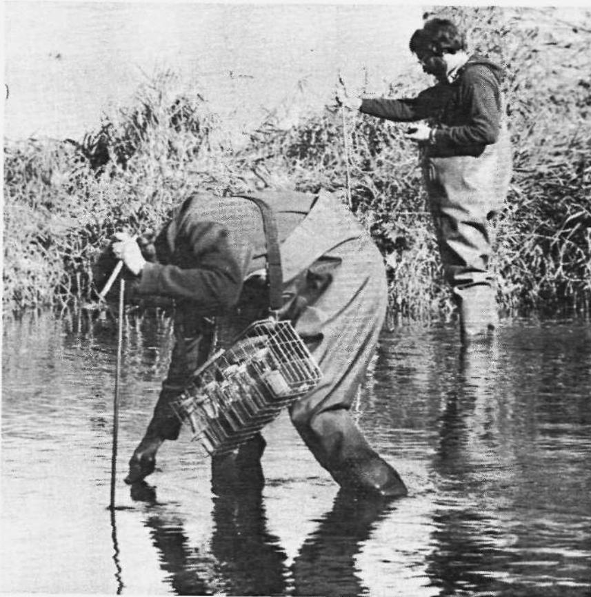
Figure 6. Technicians measuring suspended sediment and water discharge in a wadable stream
