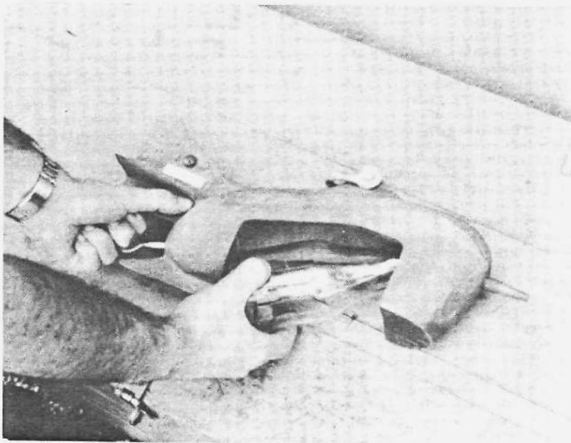
Figure 4. Depth-intergrating suspended sediment hand-type sampler, US DH-59
