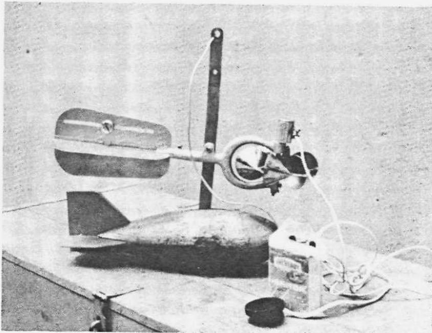
Figure 10. Price Current Meter Type-AA apparatus
