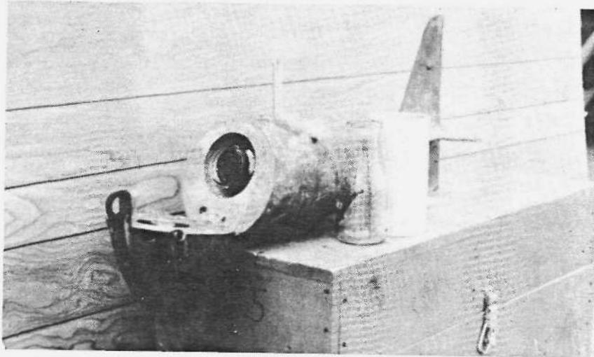
Figure 5. Point-integrating suspended sediment cable and reel sampler, US P-72
