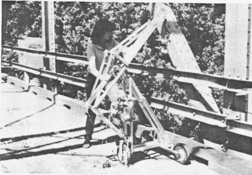
Figure 12. Stevens Sounding Reel and USGS 3-wheel base apparatus
