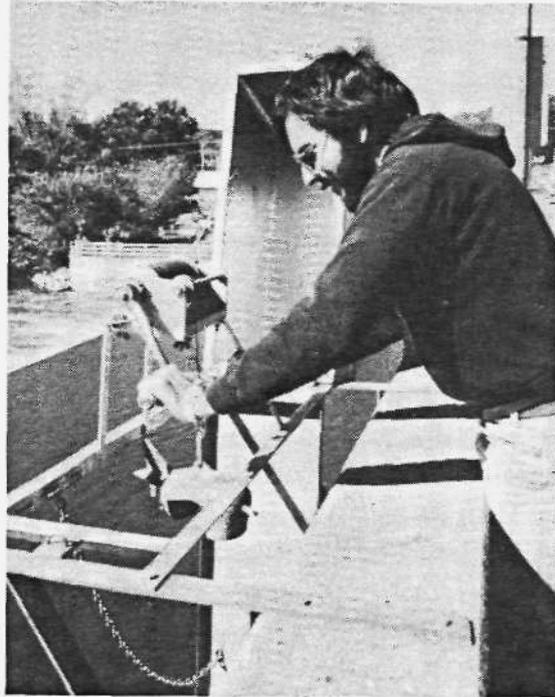
Figure 9. Preparing to collect a sediment sample using a US DH-59 installed in a California-type sediment sampling box
