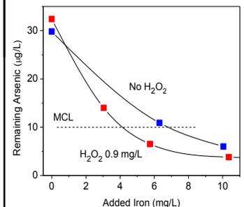
Arsenic removal in pilot scale experiments at the Danvers, IL water treatment plant. With hydrogen peroxide, a lower dose of iron could be used to meet the arsenic MCL.
