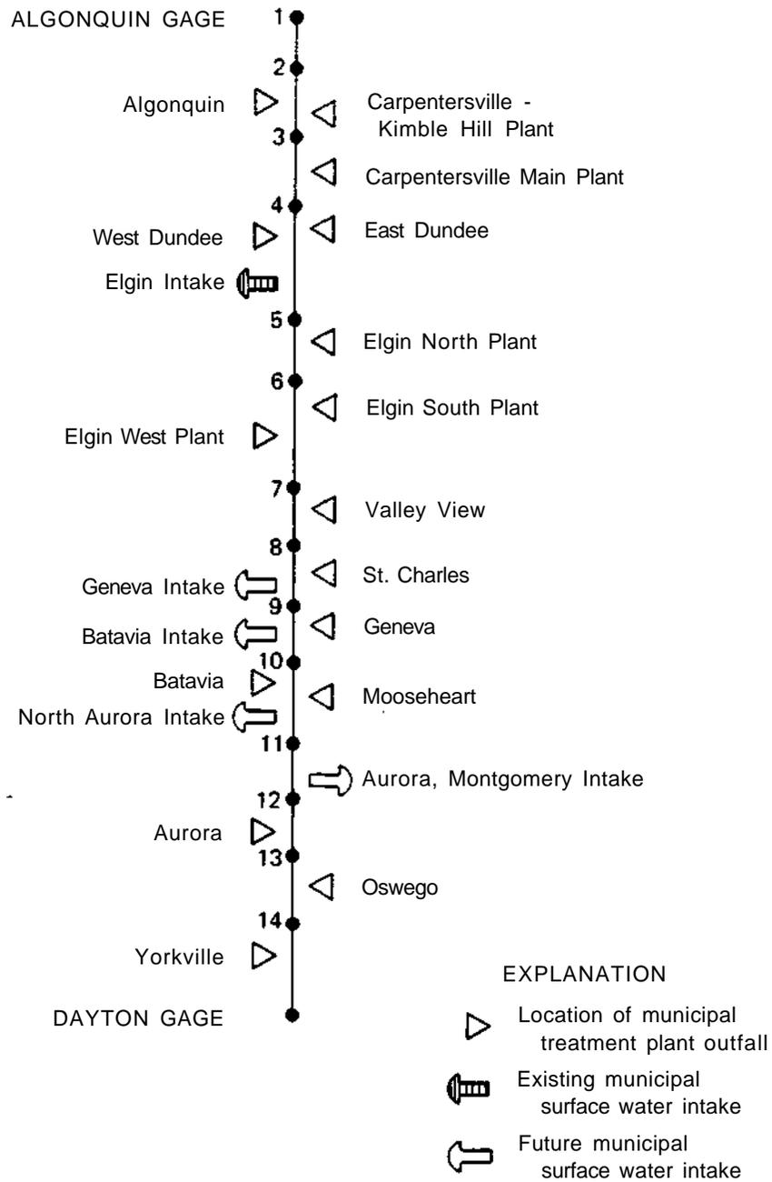
Figure 5. Schematic of Fox River, wastewater treatment plant outfalls, and existing and future municipal surface water intakes
