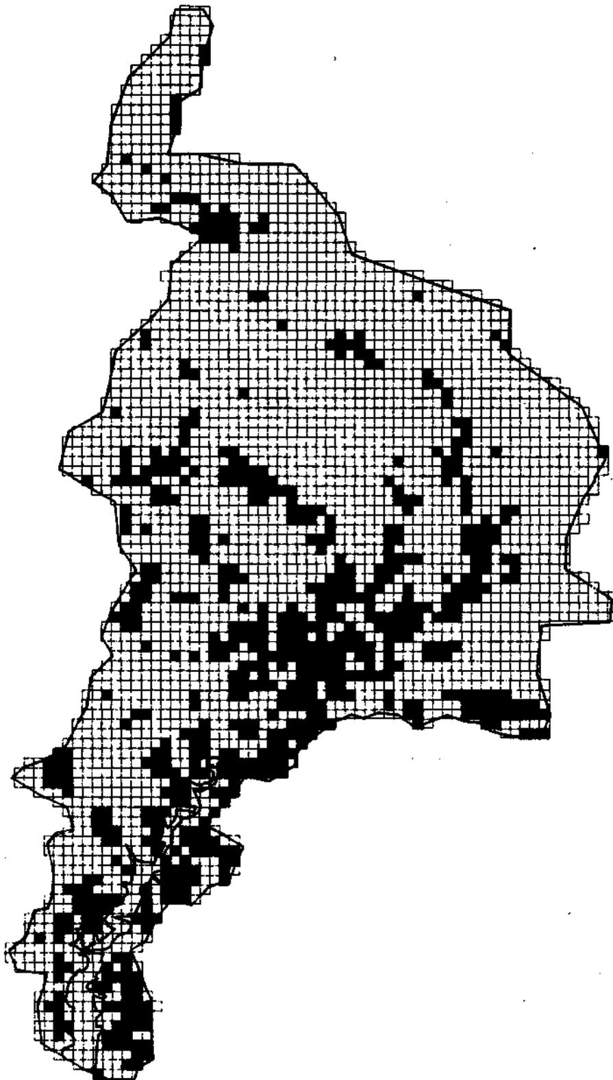
*Figure 18. Areas that generate the highest amounts of clay, as determined by the AGNPS model*
