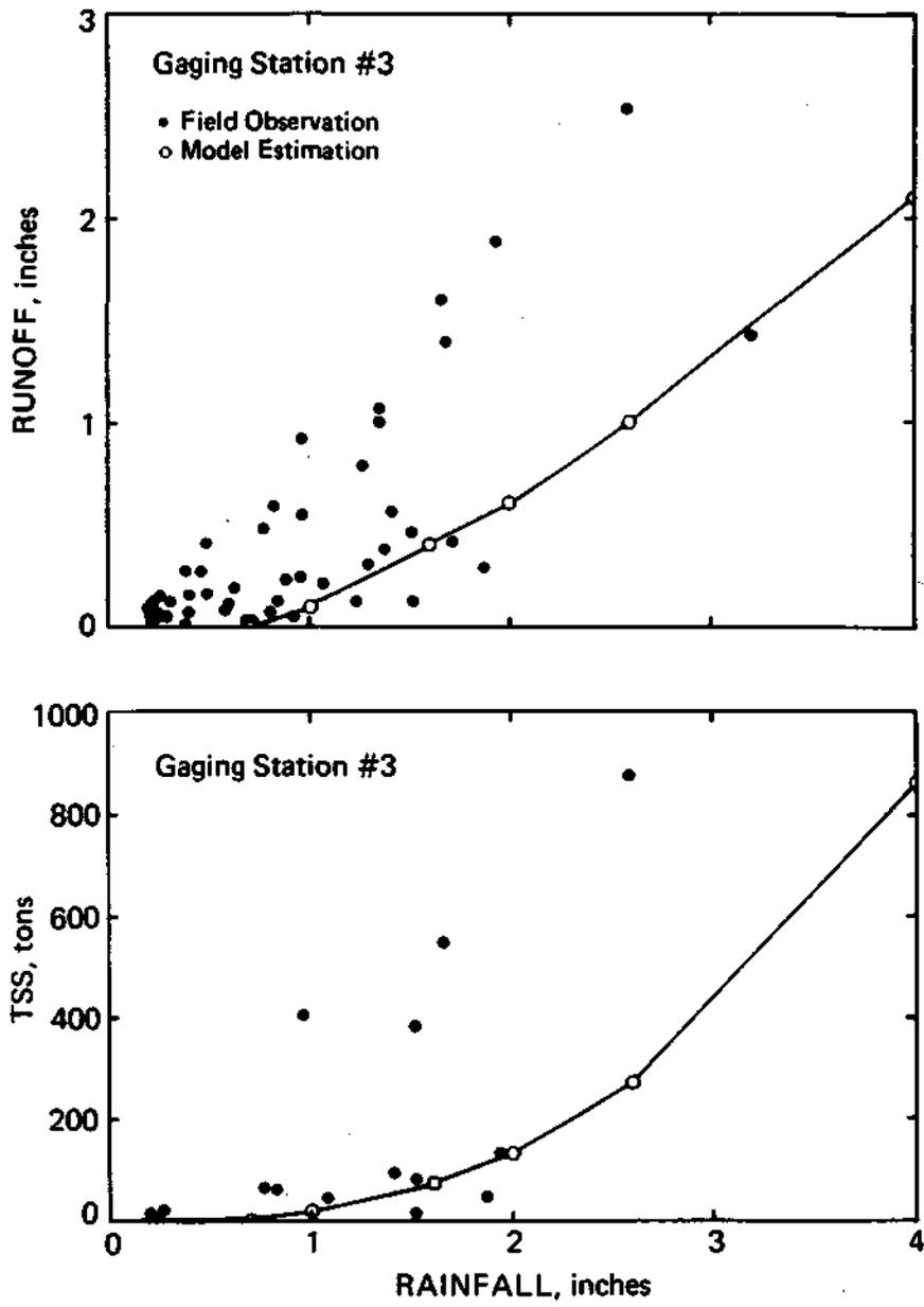
Figure 9. Observed and predicted runoff and total suspended solids at streamgaging station 3
