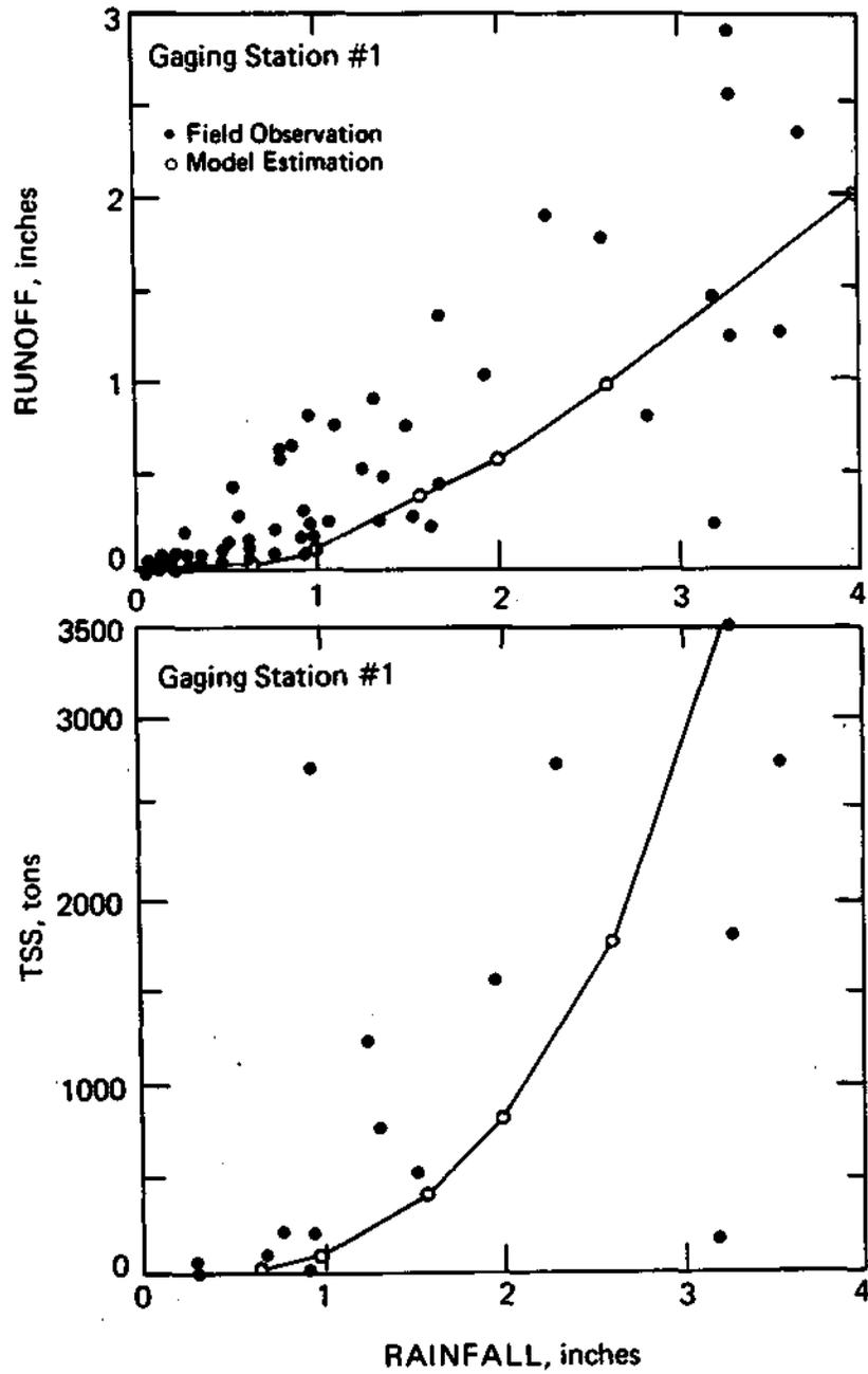
Figure 7. Observed and predicted runoff and total suspended solids at streamgaging station 1
