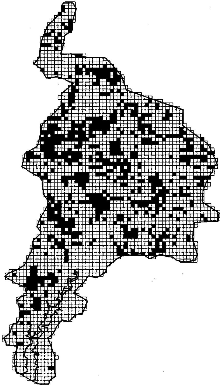
*Figure 19. Areas that generate the greatest amounts of phosphorus, as determined by the AGNPS model*
