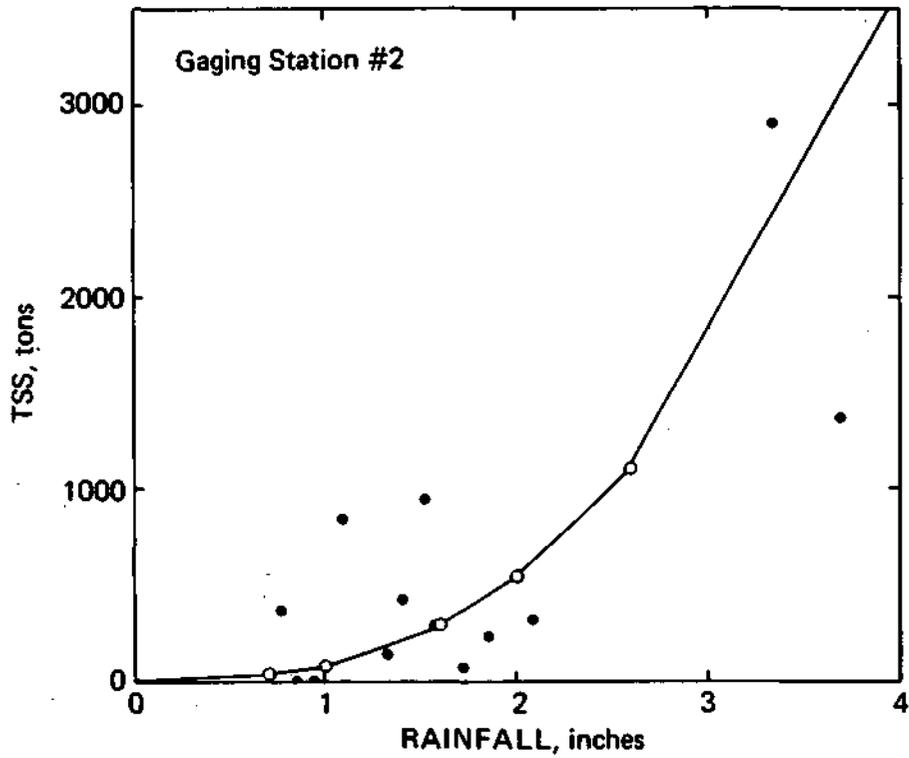
Figure 8. Observed and predicted runoff and total suspended solids at streamgaging station 2
