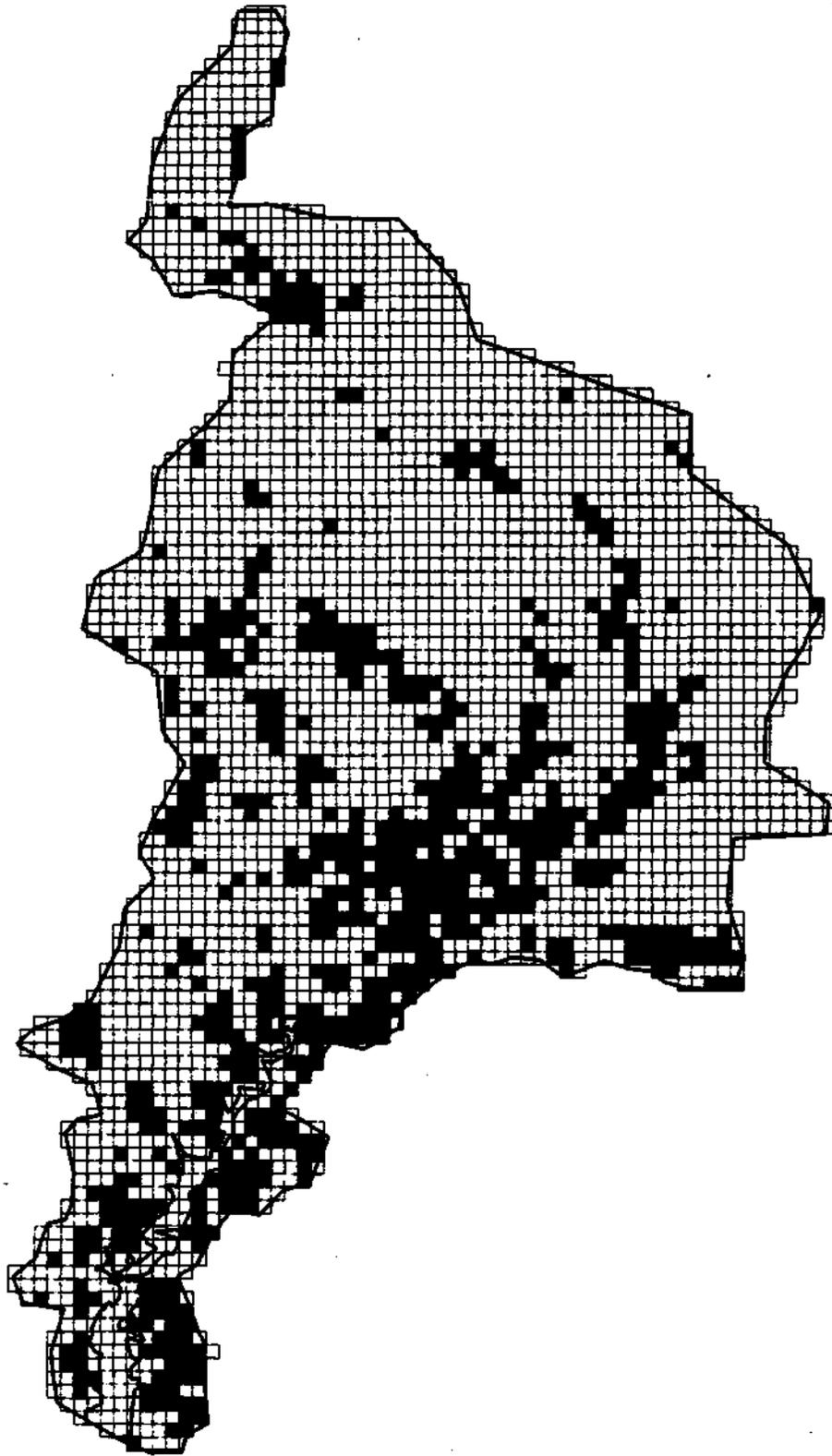
*Figure 17. Areas that generate the most sediment, as determined by the AGNPS model*
