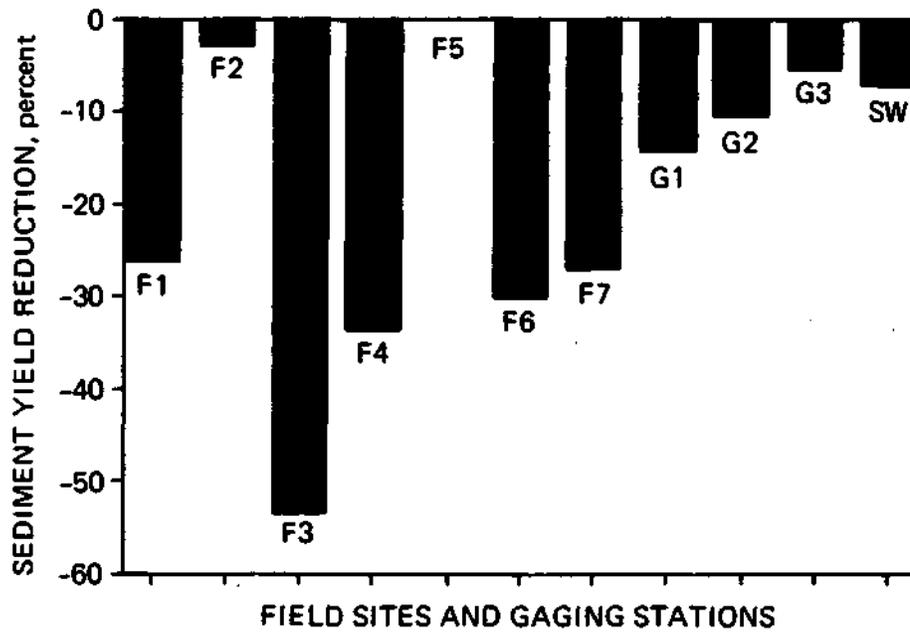
*Figure 10. Changes in sediment yield with implementation of non-structural BMPs*
