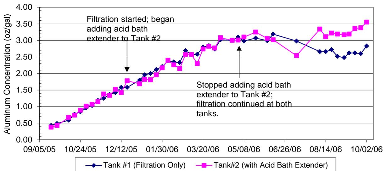
level in the tank without the extender. The acid bath extender had no noticeable effect on the aluminum contamination level. Addition of the acid bath extender ceased in May 2006. The results of using the acid
