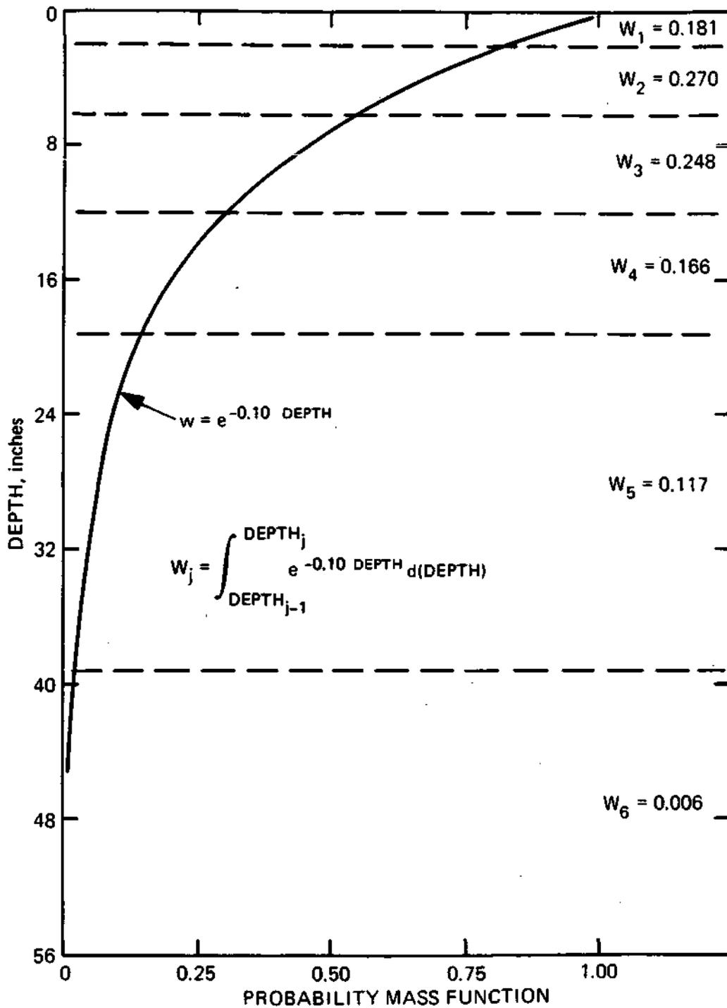
Figure 8. Relationship of the depth of a soil layer to the weighting factor used in the SCS infiltration method
