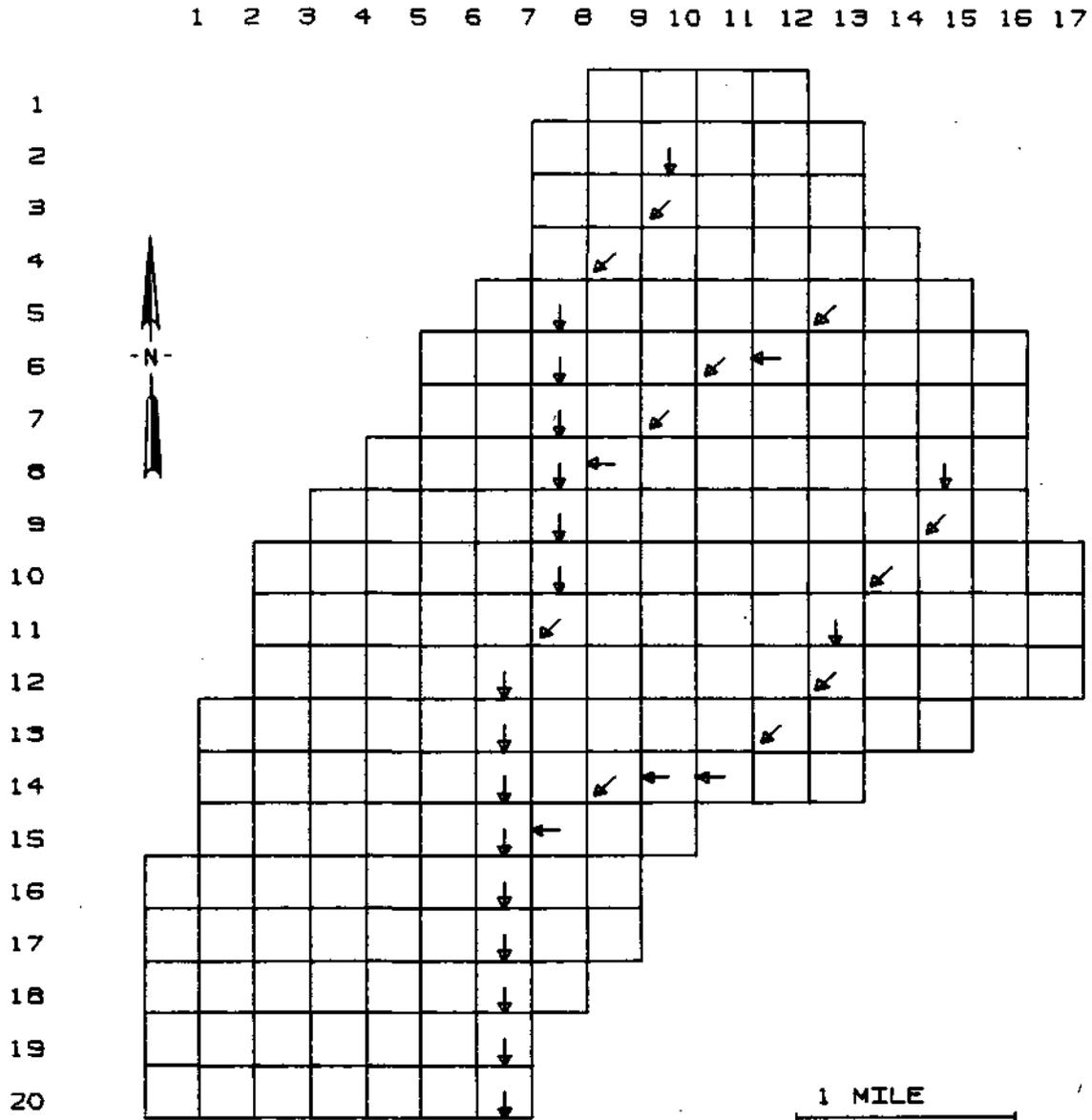
Figure 5. Representation of the channel network of a watershed as a channel grid system
