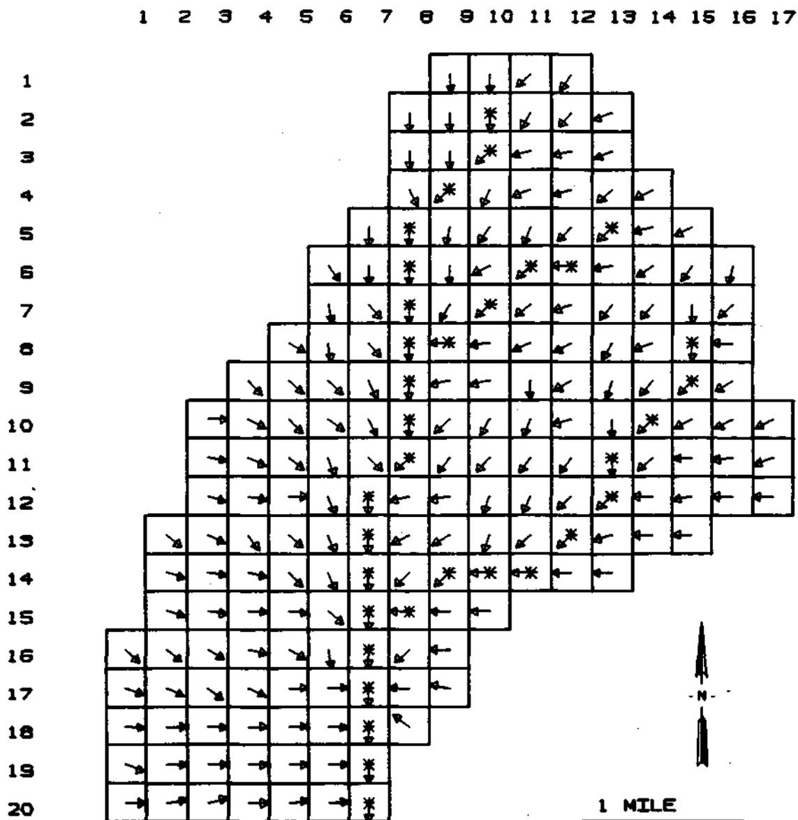
Figure 19. Representation of a catchment as a matrix of square overland and channel elements
