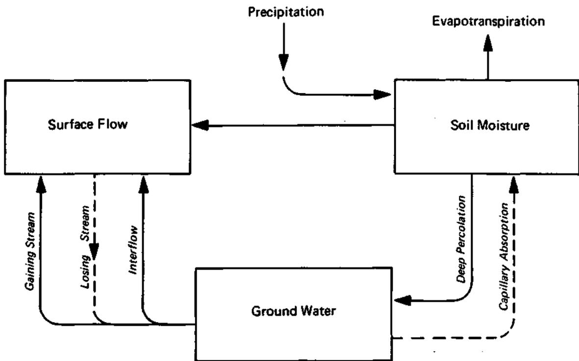
Figure 3. Movement of water within the components of the PWM
