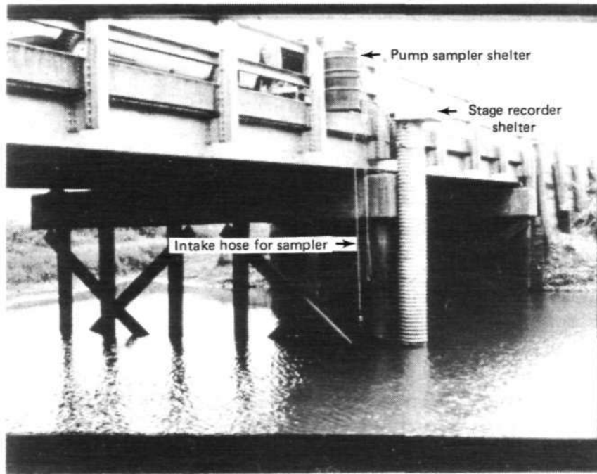
Figure 6. Project monitoring site SL2 at Lick Creek at Curran Road (The photograph shows the equipment shelters for the continuous stage recorder and the automated pump sampler)
