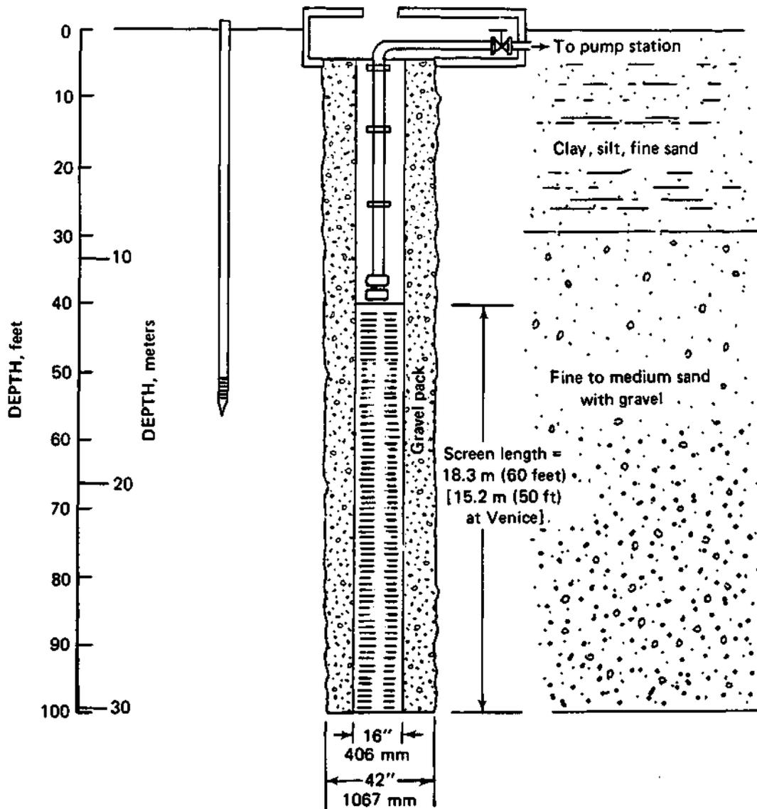
Figure 4. Typical features of a dewatering well
