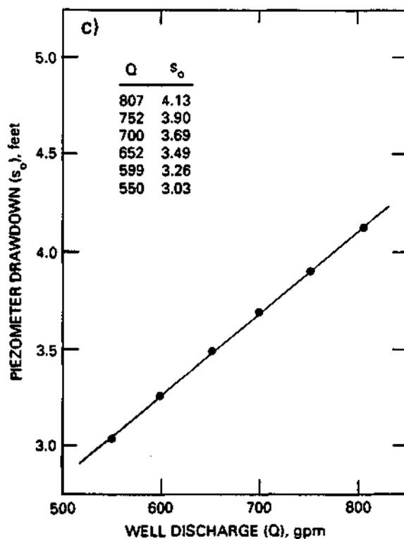
Figure 9. Results from step test of 25th Street Well No. 3, September 6, 1985: a) Determination of well loss coefficient,  $C$ ; b) water-level difference vs. well discharge; c) piezometer drawdown vs. well discharge
