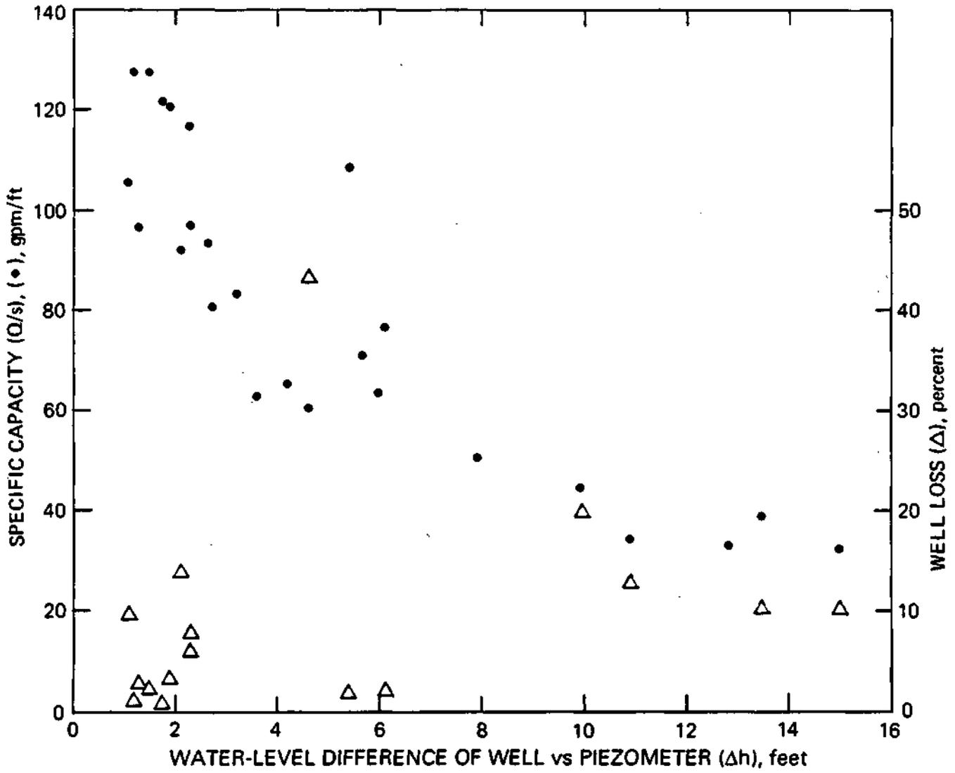
Figure 10. Water-level difference vs. specific capacity and well loss from Phases 1, 2, and 3 step tests
