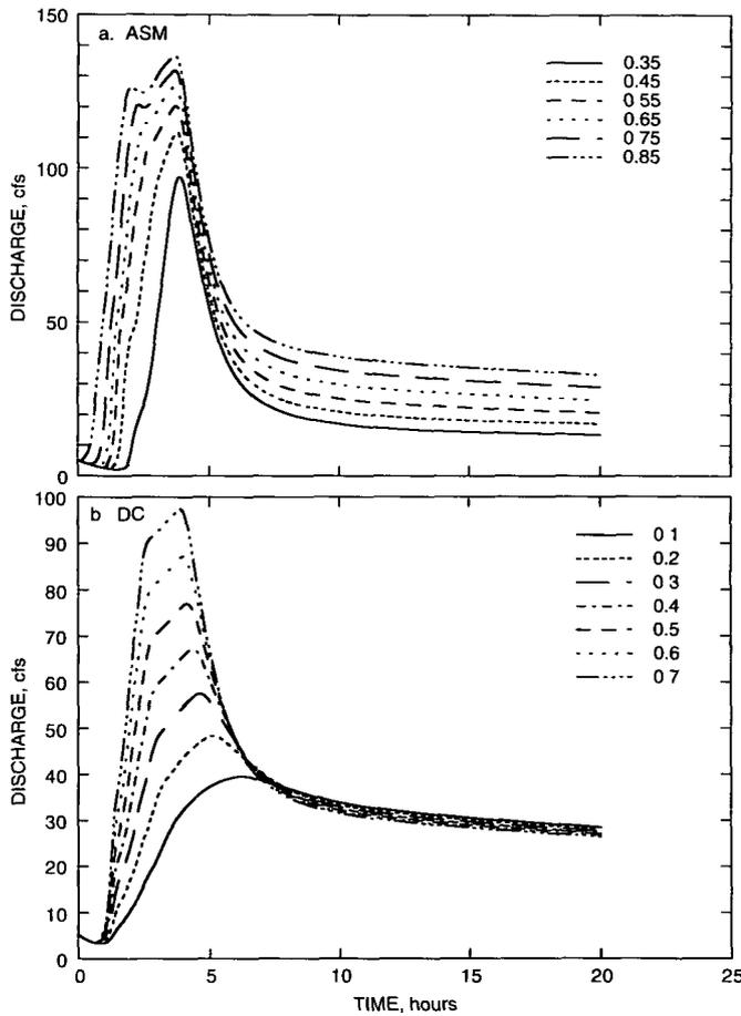
Figure 28. Influence of a) ASM and b) DC on flood hydrograph
