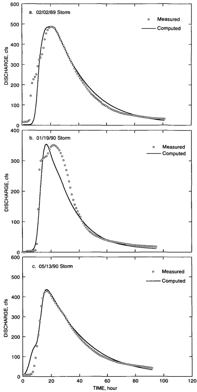
Figure 29. Comparison of computed and measured hydrographs for Cypress Creek for three storms: a) 2/2/89, b) 1/19/90, and c) 5/13/90
