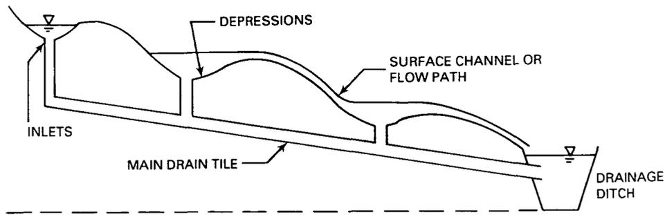
a. Schematic representation of surface drainage system
