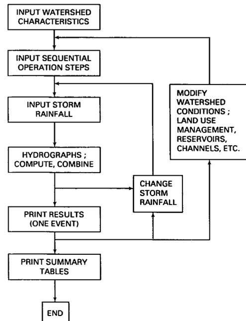
Figure 5. General structure of the TR-20 model (after Soil Conservation Service, 1973)
