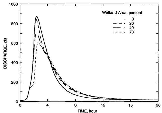
Figure 30. Comparison of discharge hydrographs for different percent wetland at the watershed outlet
