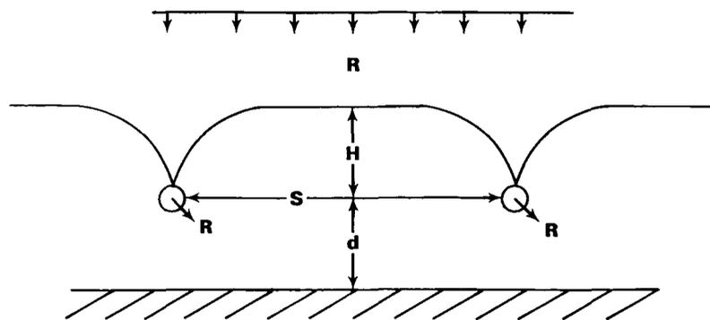
d. Schematic diagram of subsurface tile drainage system
