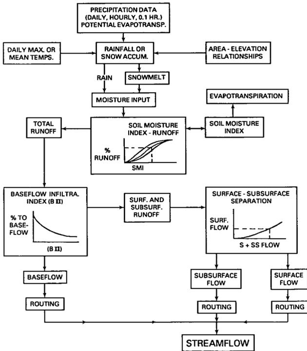
Figure 3. General form of the Streamflow Synthesis and Reservoir Regulation (SSARR) model (after U.S. Army Corps of Engineers, 1972a)
