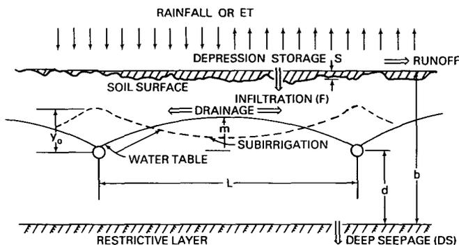
Figure 14. Schematic representation of the DRAINMOD model (after Skaggs, 1980)
