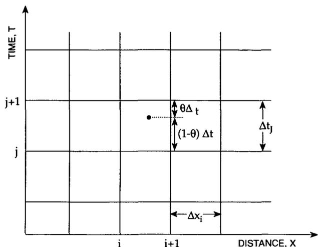
Figure 23. The four-point scheme for finite difference discretization
