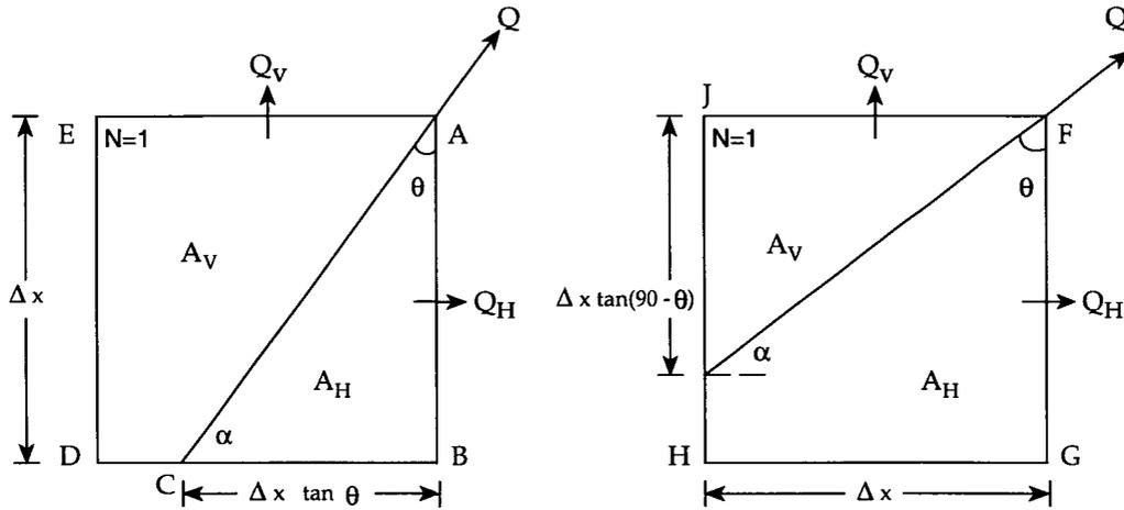
b. Definition of the terms used in the derivation of the vertical and horizontal components of discharge
