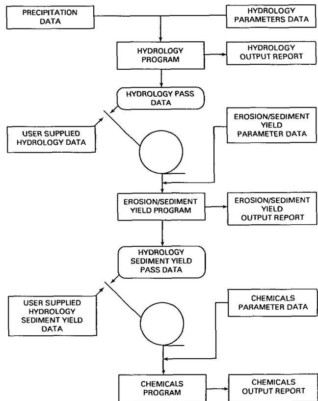
Figure 7. Generalized flow chart of the Chemicals, Runoff, and Erosion from Agricultural Management Systems (CREAMS) model (after U.S. Department of Agriculture, 1980)
