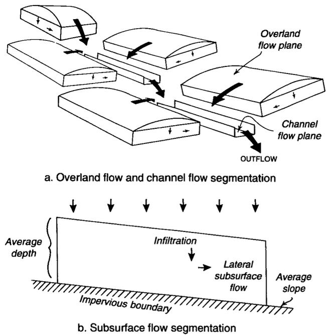
Figure 12. Schematic representation of the Institute of Hydrology Distributed Model or IHDM (after Rogers et al., 1985)
