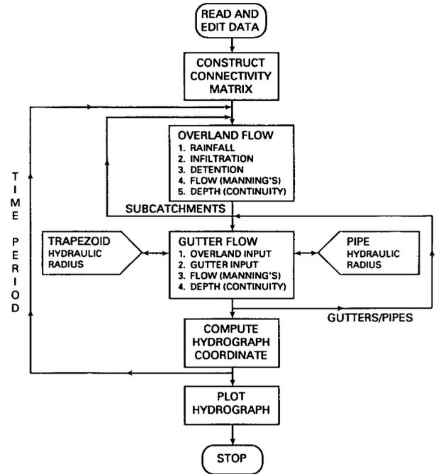
Figure 4. Generalized flow chart of the Storm Water Management Model or SWMM (after Lager et al., 1971)
