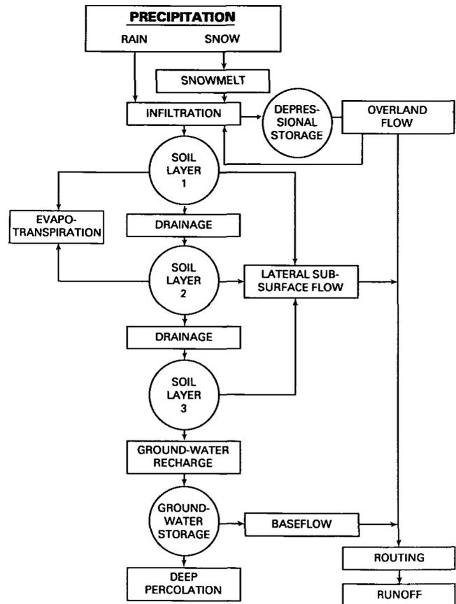
Figure 2. General structure of the U.S. Department of Agriculture Hydrograph Laboratory-74 (USDAHL-74) model (after Holtan et al., 1975)
