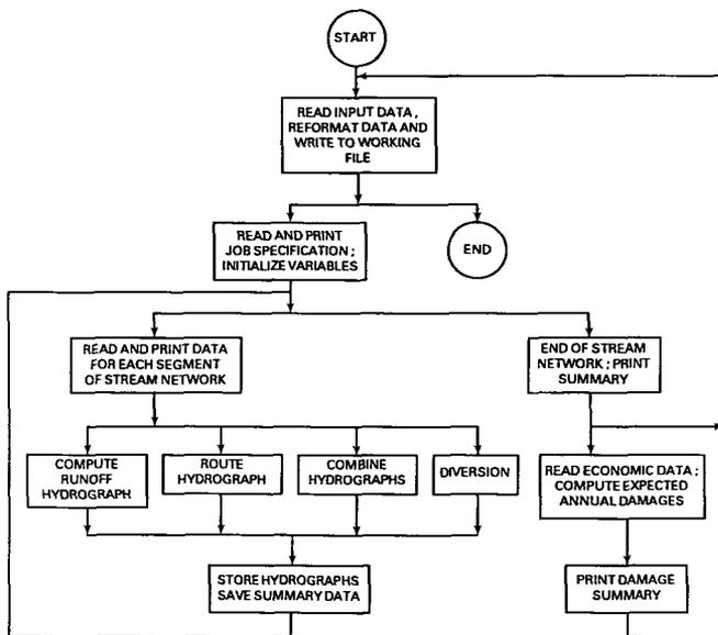
Figure 6. Flow chart representation of the Hydrologic Engineering Center-1 (HEC-1) model (after U.S. Army Corps of Engineers, 1985)
