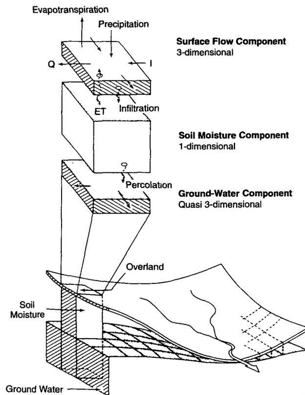
Figure 10. Components of the PACE Watershed Model or PWM (after Durgunoglu et al., 1987)
