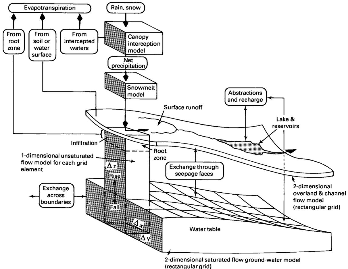
Figure 8. Conceptual representation of the SHE model (after Abbott et al., 1986)
