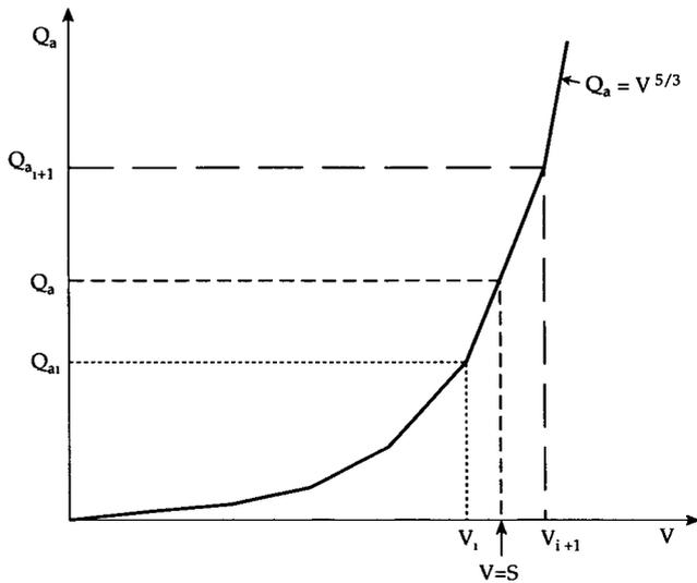
Figure 21. Piecewise linear segmented curve approximation for Manning equation
