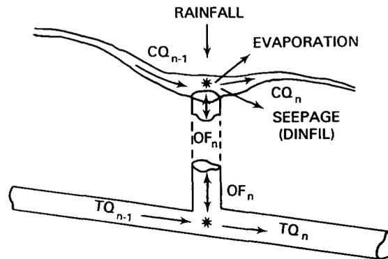
b. Flow pattern for surface drainage of a typical depression
