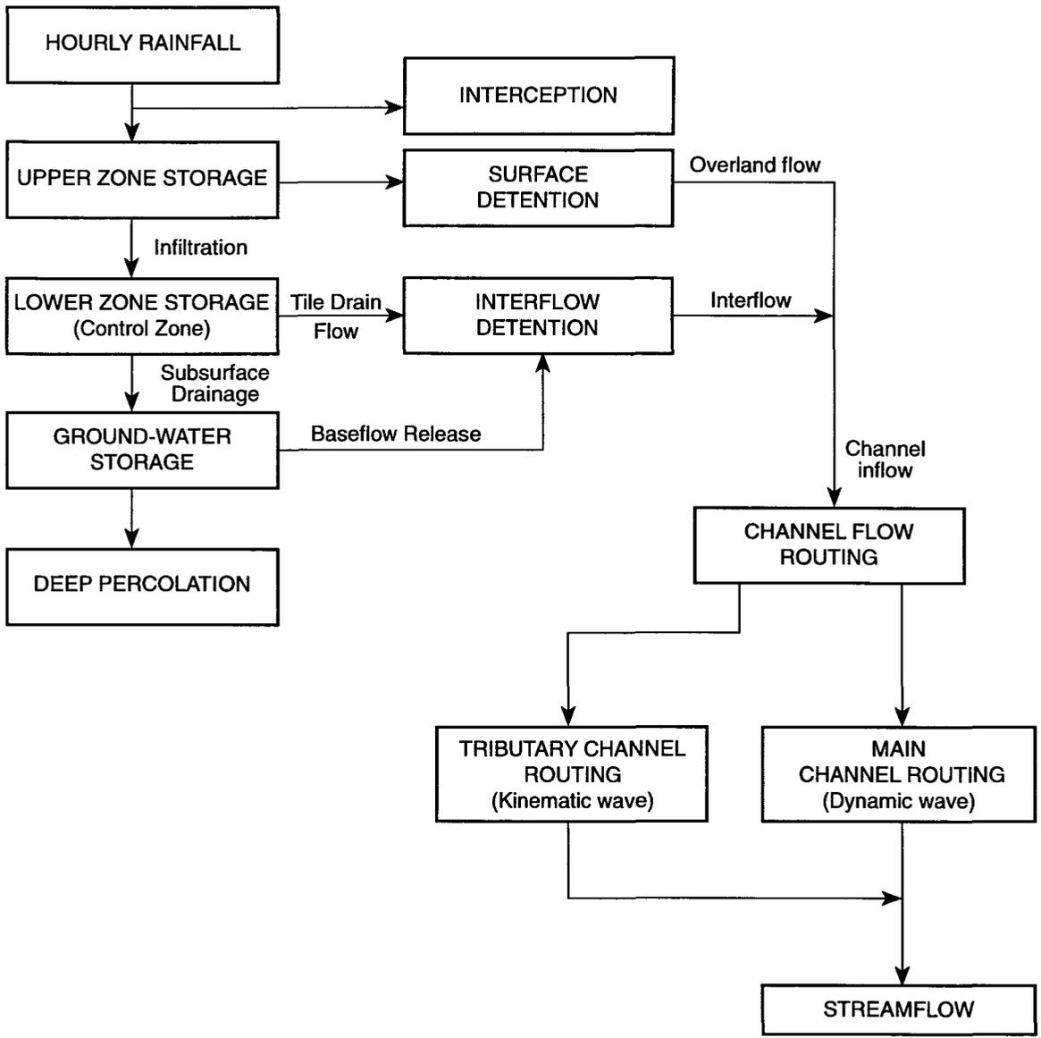
Figure 24. Wetland hydrologic model
