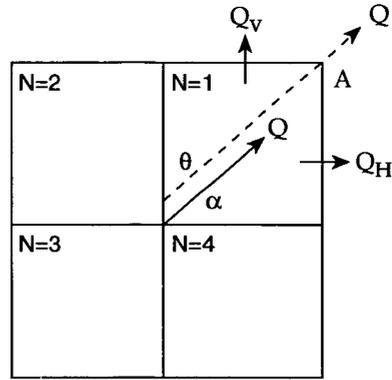
a. Schematic diagram of the flow direction and its resolution in element N=1 in relation to adjacent elements
