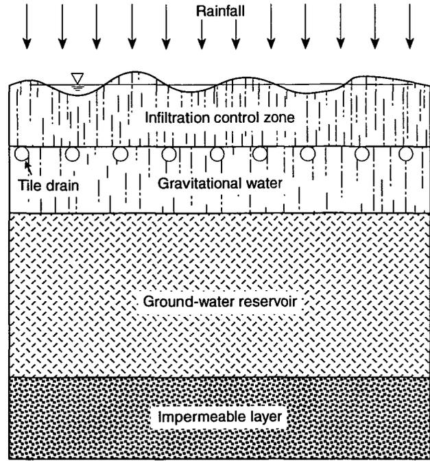
Figure 18. Schematic diagram of subsurface drainage
