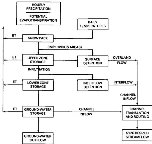
Figure 1. General form of the Stanford Watershed Model or SWM (after Crawford and Linsley, 1966)
