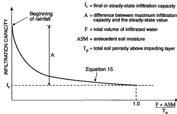
Figure 17. Distribution of infiltration capacity with soil moisture
