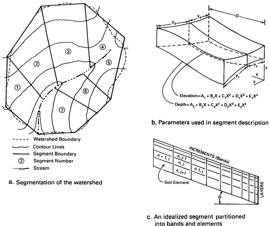
Figure 11. Watershed segmentation in the Variable Source Area Simulator 2 (VSAS2)
