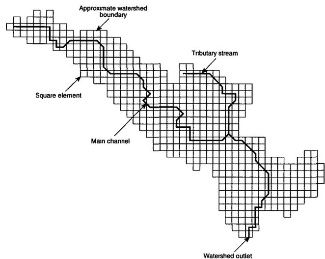
Figure 26. Discretization of Cypress Creek watershed (not drawn to scale)
