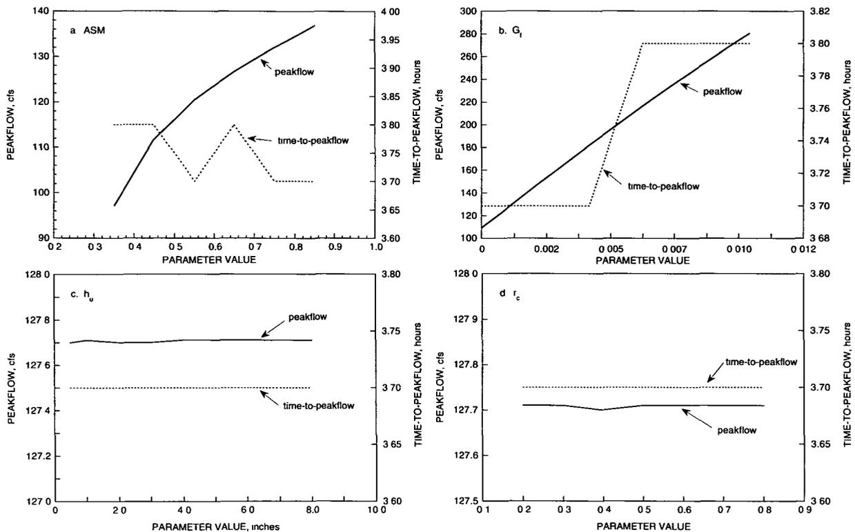
Figure 27. Variation of peakflow and time-to-peakflow to changes in a) ASM, b)  $G_f$ , c)  $h_u$ , d)  $r_c$ , e)  $DF$ , f)  $DC$ , g)  $n_o$ , h)  $n_c$ , i)  $f_c$ , and j)  $A$
