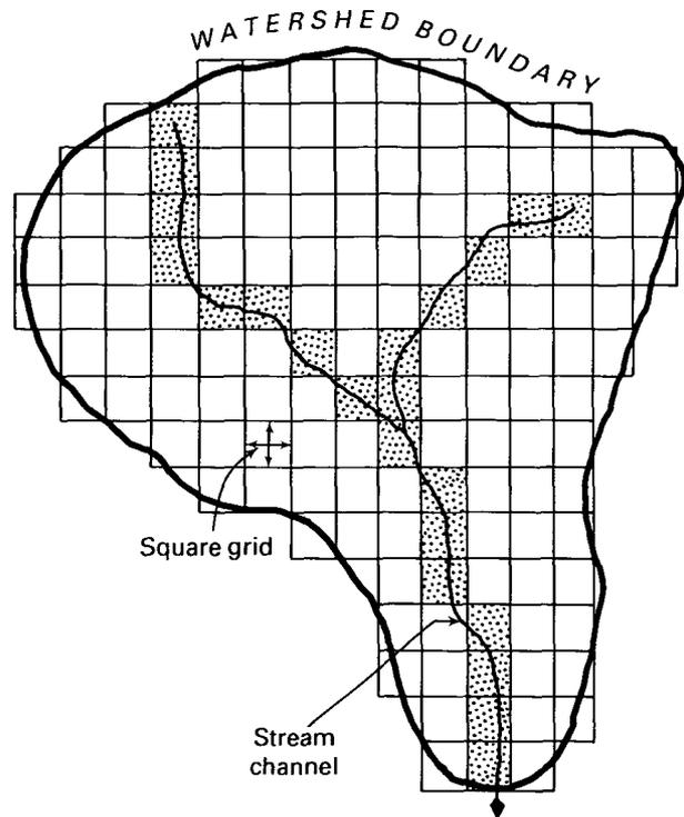
Figure 9. Square grid network in the Areal Nonpoint Source Watershed Environment Response Simulation (ANSWERS) model (after Beasley, 1977)
