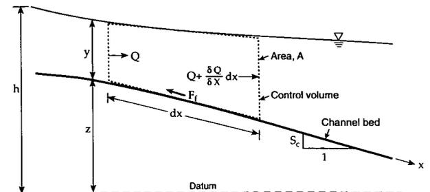
Figure 22. Control volume in a channel reach
