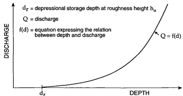
Figure 19. Depth-runoff relations for overland flow
