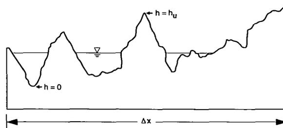
Figure 16. Ground surface topographical profile used to derive surface storage relations
