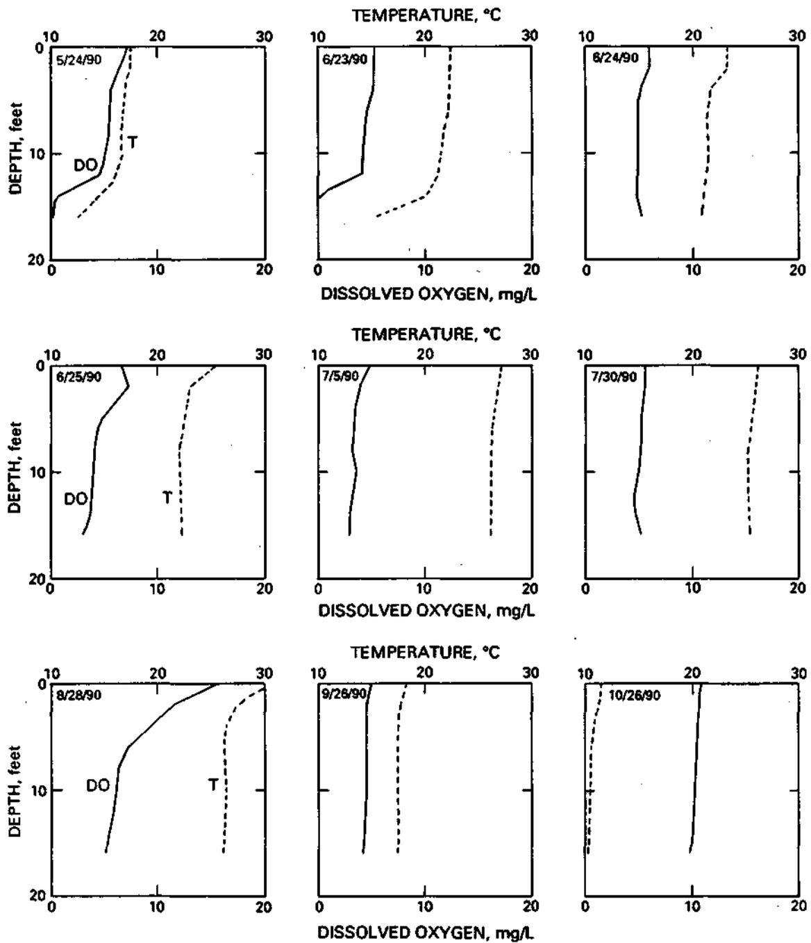
Figure 3. Temperature and dissolved oxygen profiles for the deep station on selected dates
