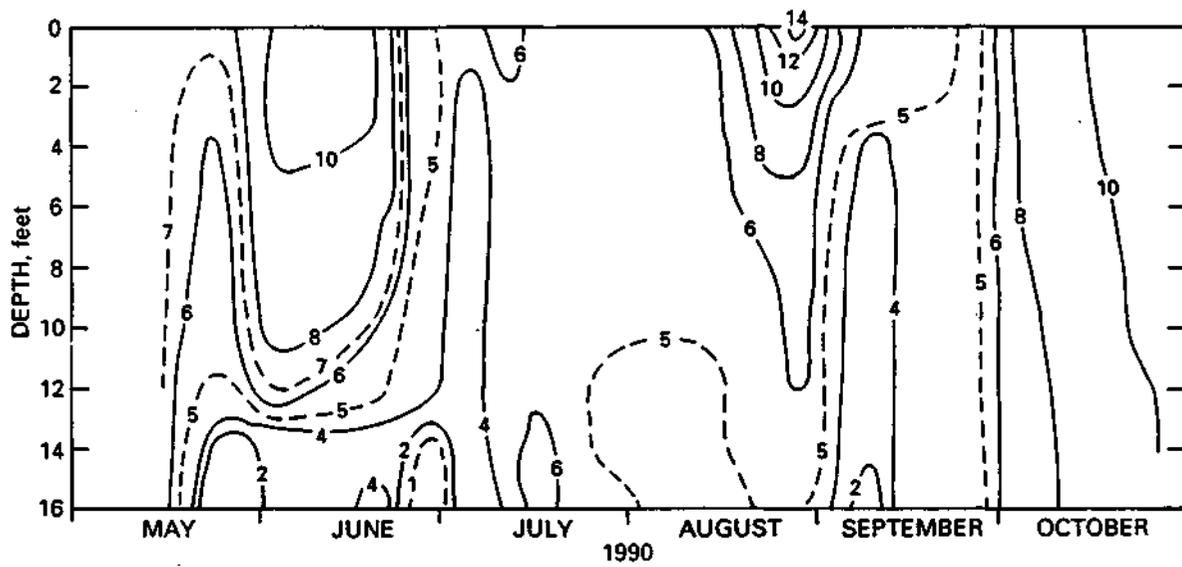
Figure 2. Isopleths of dissolved oxygen for the deep station
