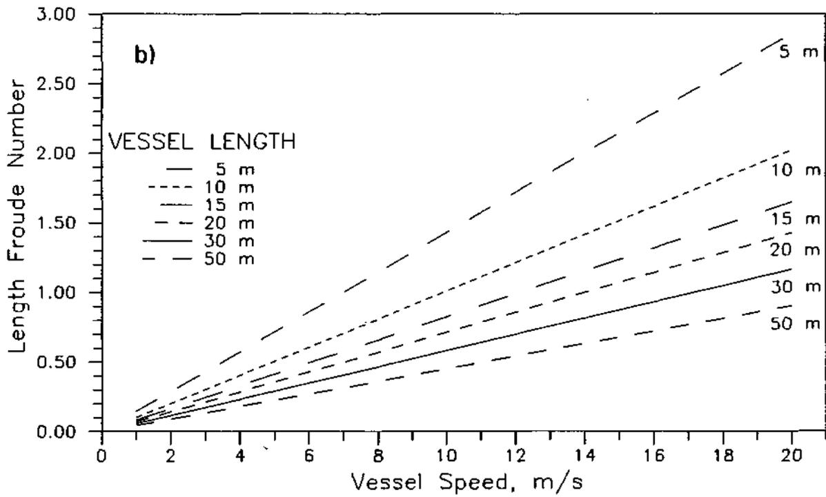
Figure 7. Length Froude Numbers,  $F_L = Vr/(gl)^{0.5}$ , for
