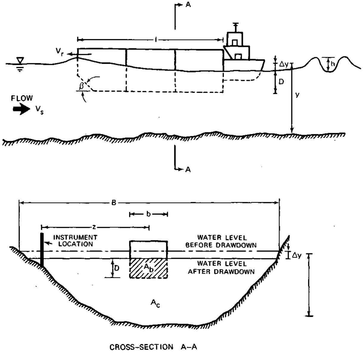
Figure 2. Definition sketch for vessel and environmental variables
