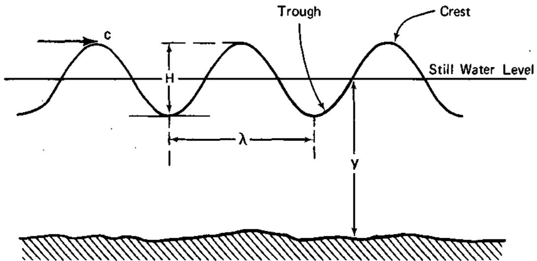
Figure 4. Longitudinal wave profile and wave variables
