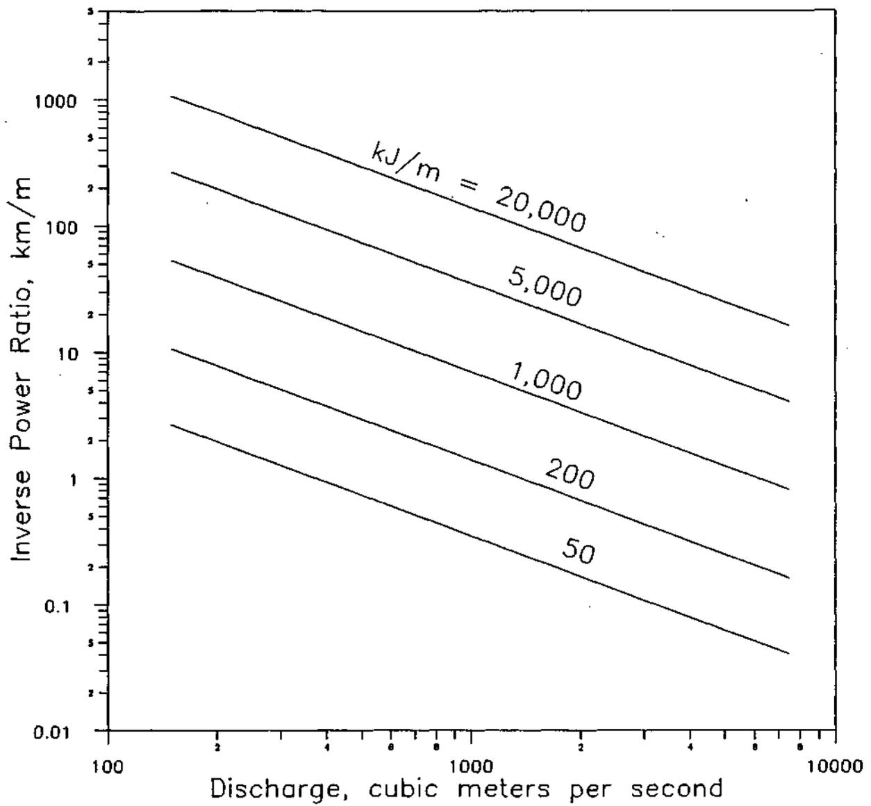
Figure 8. Inverse power ratio as a function of river flow rate and towboat power/speed ratio
