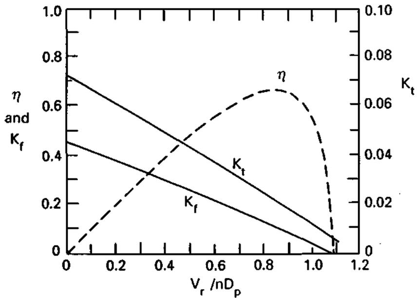
Figure 11. Typical dimensionless propeller performance curves:
