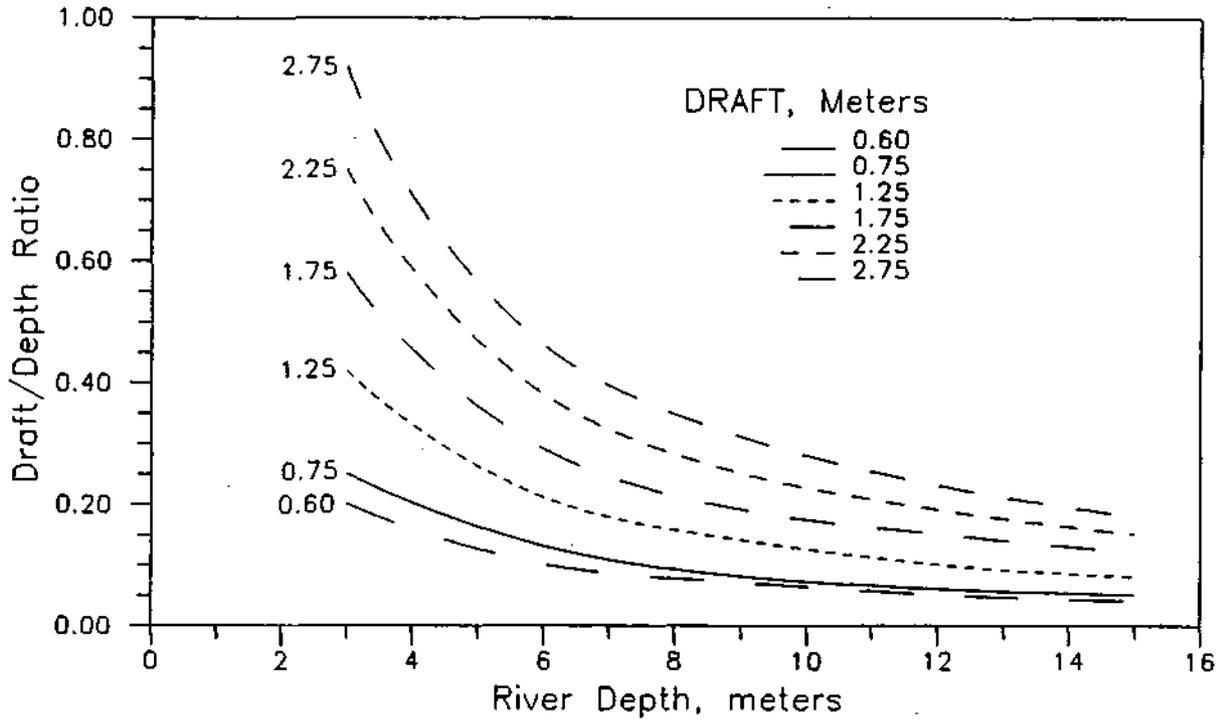
Figure 5. Draft/depth ratios for barge tows on the Upper Mississippi River System
