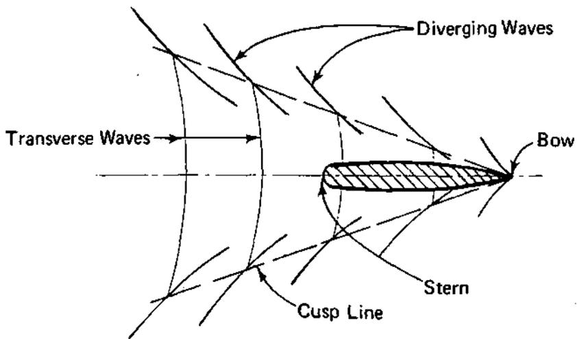
Figure 3. Wave pattern generated by a vessel
