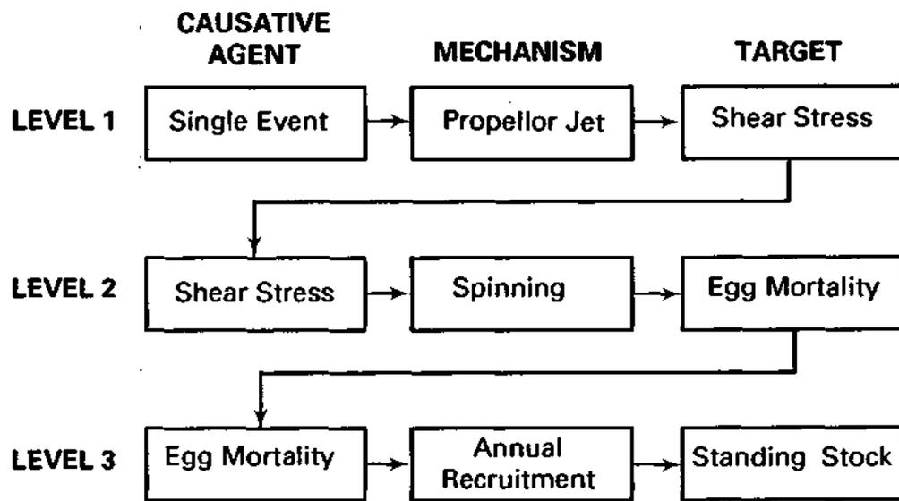
Figure 13. Conceptual model levels for single barge tow passage event effects
