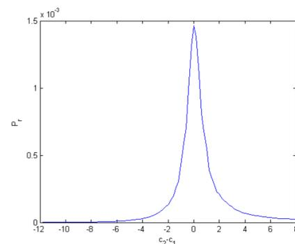
Figure 4. Power in the receiver as a function of the difference in spring-like constants.
