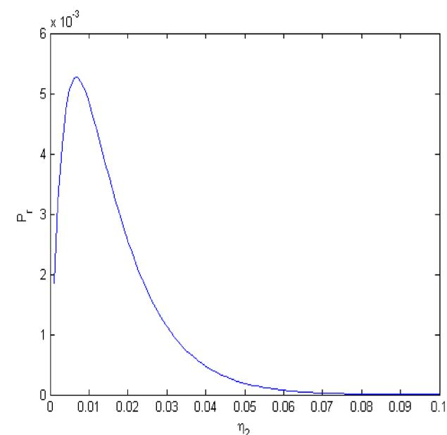
Figure 6. Power flowing through the receiver for different  $\eta_2$  values.
