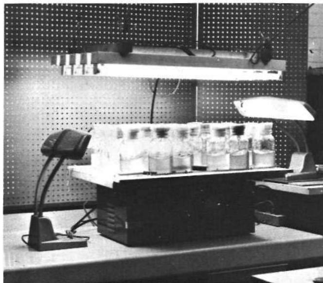
Figure 3. Shaker platform and illumination for incubation
