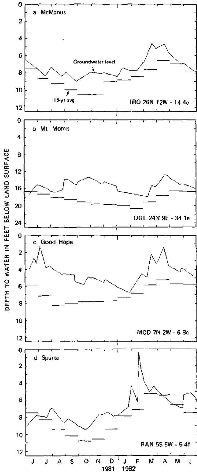
Figure 22. Groundwater hydrographs for representative observation wells
