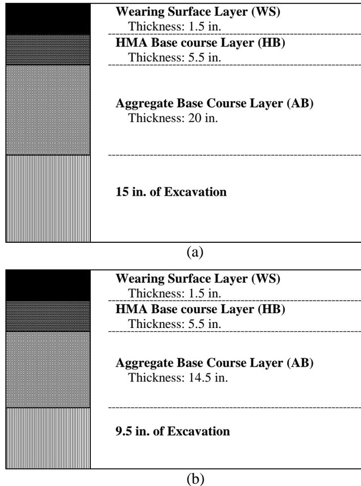
**Figure 15. Road profile for conventional pavement (a) and geotextile reinforced pavement (b).**
