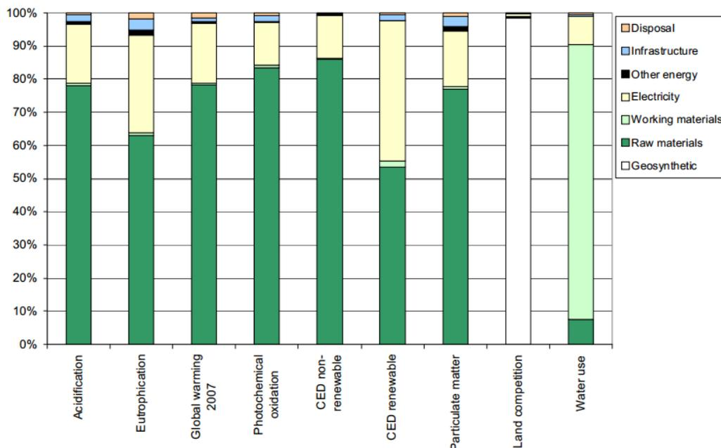
**Figure 4. Environmental impacts caused by the geosynthetic drainage layer (Werth et al., 2012).**
