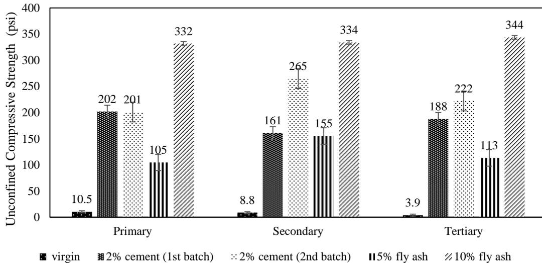
**Figure 12. Unconfined compressive strength test results for virgin QB samples and samples stabilized with 2% Portland cement, 5% Class C fly ash, and 10% Class C fly ash.**
