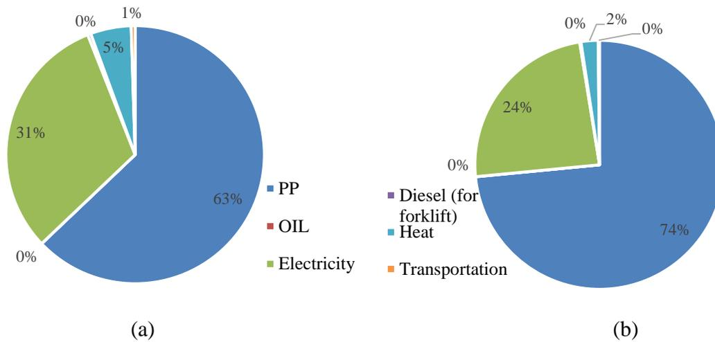
**Figure 14. Energy consumed (b) and GWP (a) for production of geotextile.**
