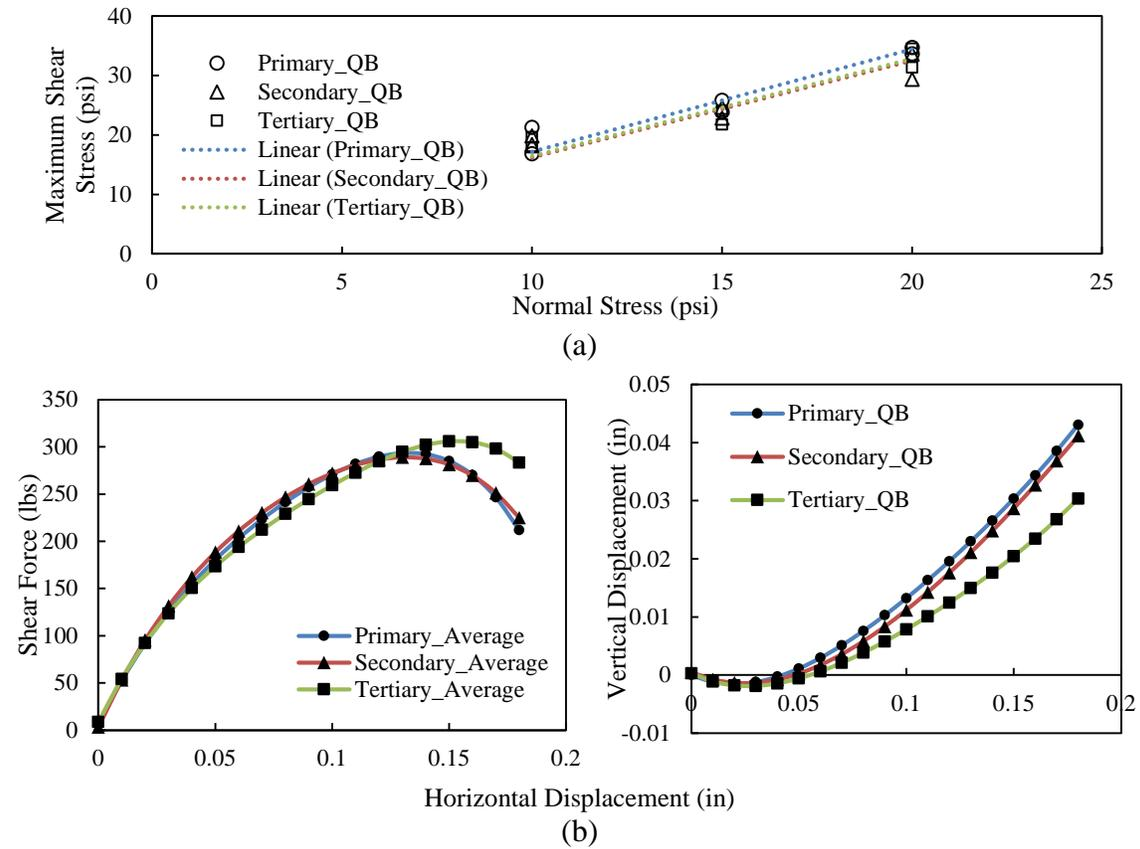
**Figure 9. Direct shear test results: (a) maximum shear stress under different normal stresses; (b) shear force and vertical displacement varying with horizontal displacement at 10 psi normal stress.**
