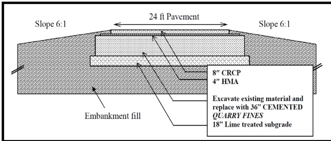
**Figure 2. Typical test embankment with cement-treated quarry fines as a pavement base material in Arlington, Texas (Puppala et al., 2012).**
