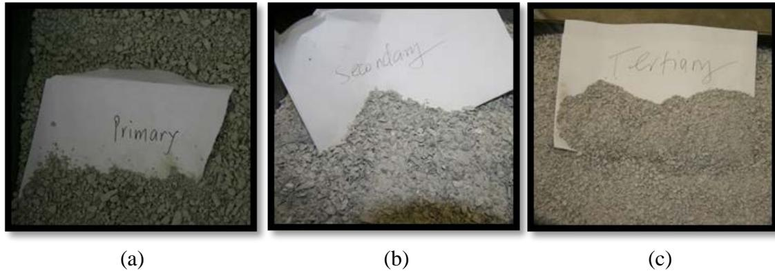
**Figure 6. Samples collected from different crushing stages: (a) Primary, (b) secondary, (c) tertiary stage.**
