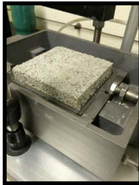
**Figure 8. A sample prepared for the direct shear test.**
