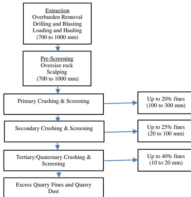
**Figure 1. Flowchart for a typical quarry operation (Stroup-Gardiner and Wattenberg-Komas, 2013).**
