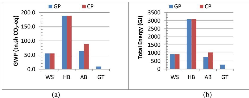
**Figure 16. Comparing GWP (a) and total energy (b) for material production of different pavement layers.**
