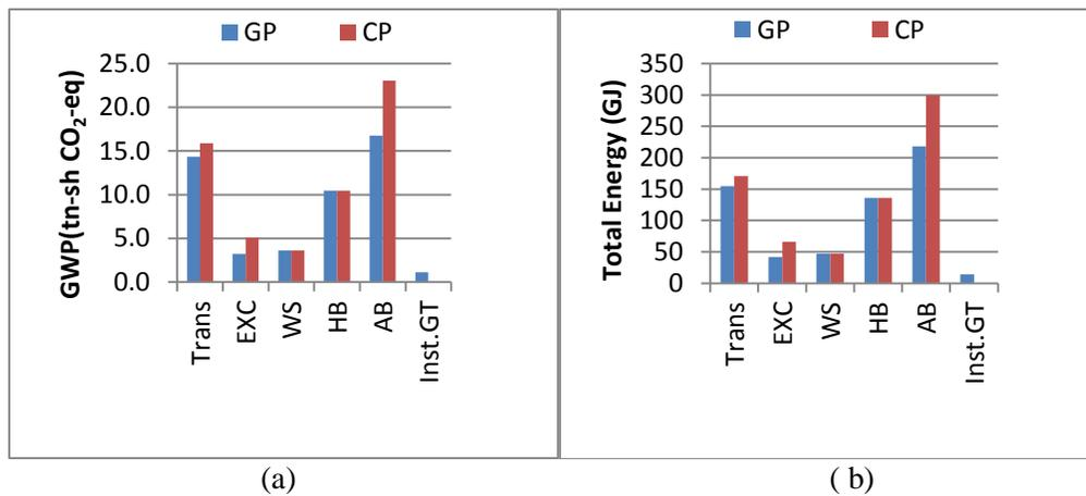
**Figure 17. Comparing GWP (a) and total energy (b) in construction of different pavement layers per 2 lane-mile.**
