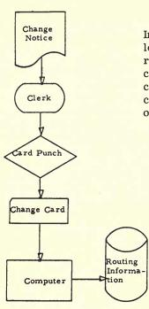
Information relating to additions, deletions and address changes to the routing lists are punched into IBM cards. These cards are fed into the computer which makes the necessary changes to the lists stored magnetically on the disk surfaces.
