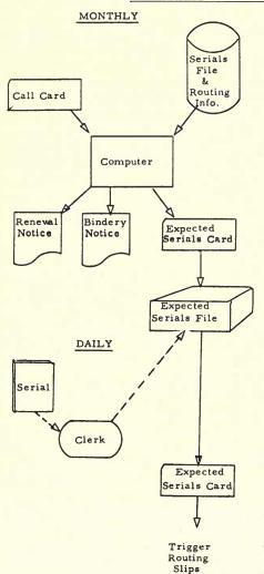
The Call Card calls from disk storage the computer program which generates the monthly Expected Serials File. This file consists of a punched IBM card for each copy of each serial expected the following month. The card is punched with journal name, volume number, month, copy number, destination library, bindery code, class number.
