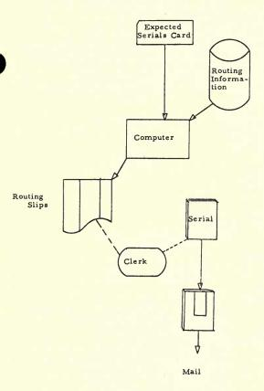
The Expected Serials Cards are fed into the computer. The disk file contains the routing lists, which are stored magnetically on its disk surfaces. The computer then prints the paper routing slips corresponding to the Expected Serials Cards. The routing slips contain serial name, number, issue, copy, and date, as well as a numbered list of the recipients.
