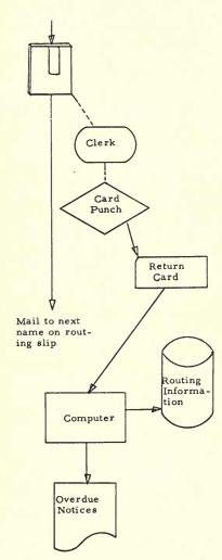
After a reader has finished the serial, he returns it to the library. The serials clerk key punches an IBM return card with the journal identification and the line number of the last name scratched off the list. The return card can contain information for more than one transaction.
