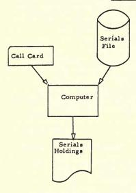
Periodically, the computer can print a Serials Holdings List from information stored magnetically on the disk file. This list can be prepared in multiple carbon copies or directly on reproduction mats by the computer.
