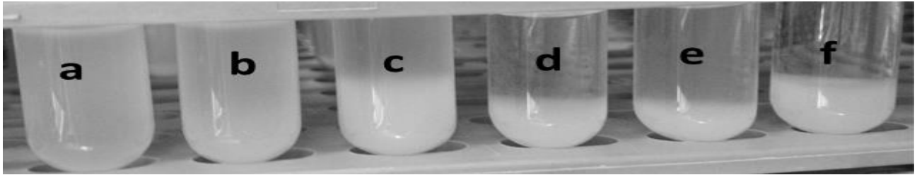
Figure 1. Examples of Degree of Aggregation. Tubes provide examples of how the degree of aggregation was ranked visually. a.) 0+ b.) 1+ c.) 2+ d.) 3+ e.) 3+ f.) 4+
