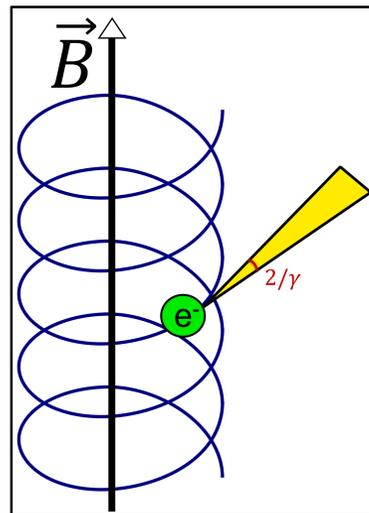
Schematic illustrating synchrotron radiation production by a relativistic electron (in green) orbiting around a magnetic field line (black). The electron follows a helical orbit (dark blue) and emits radiation into a cone-shaped region (yellow) of width  $2/\gamma$  (dark red).
